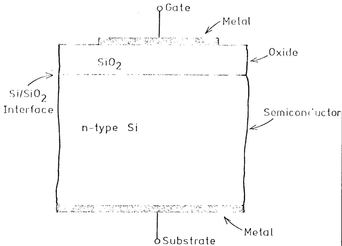
Figure 1.1 Structure of the MOS capacitor.
