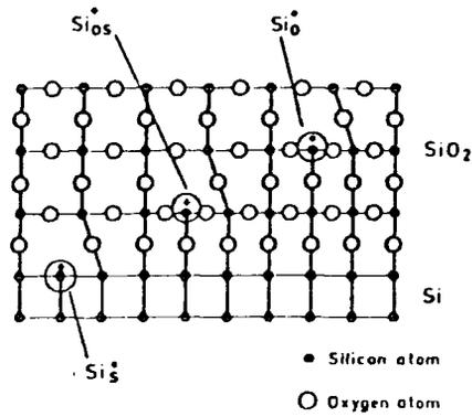
Figure 2.2 The silicon-silicon dioxide interface with three trivalent silicon defects (4)
