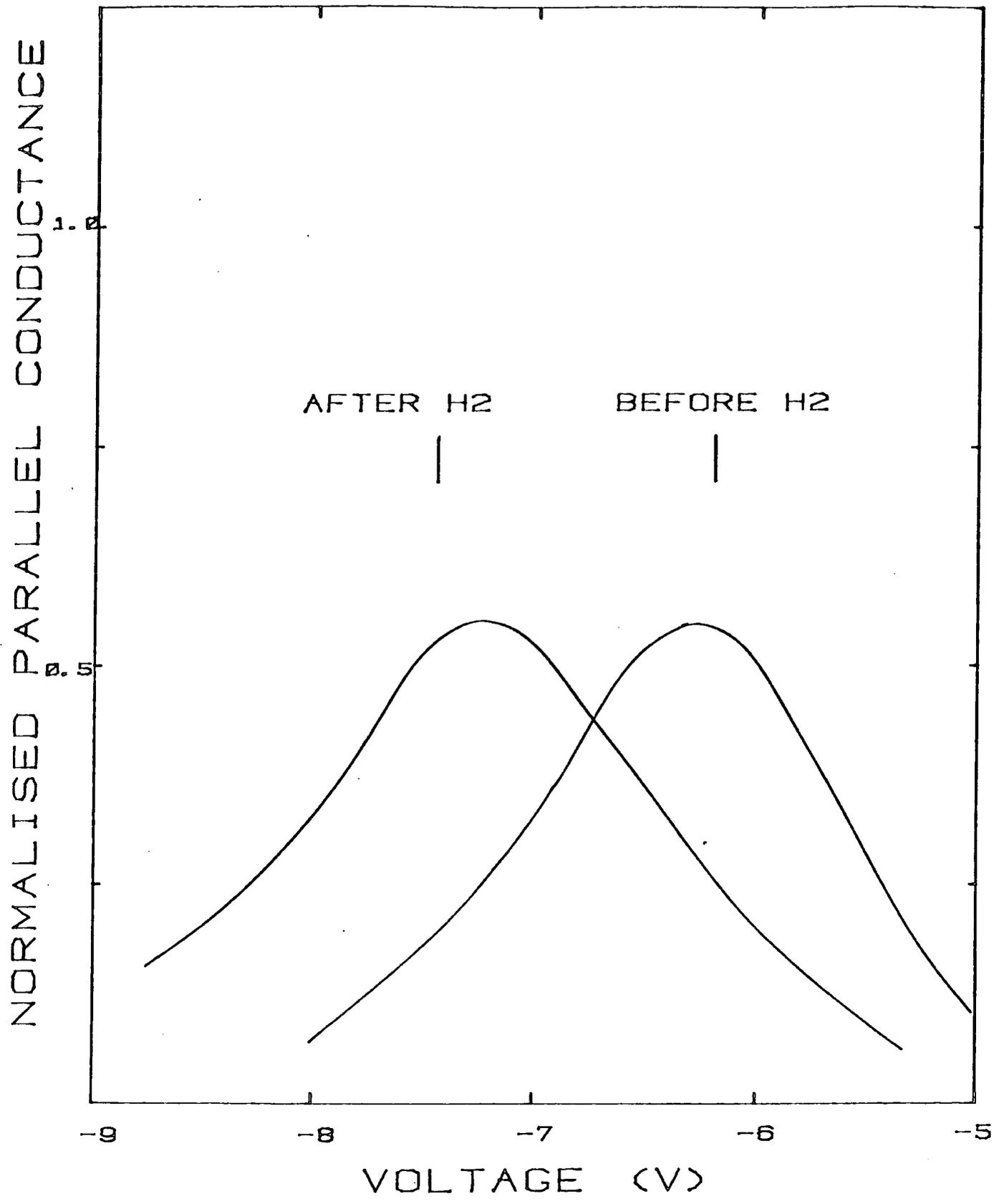
Figure 6.7 Parallel conductance plots for Pd MOS device, before and after exposure to hydrogen.
