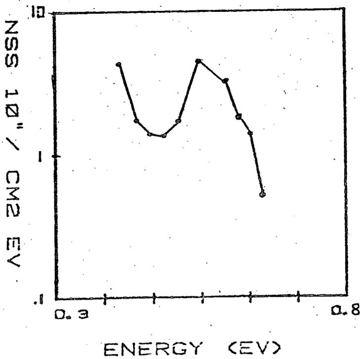
Figure 5.6 Quasi-static curves for gold-doped silicon sample.
