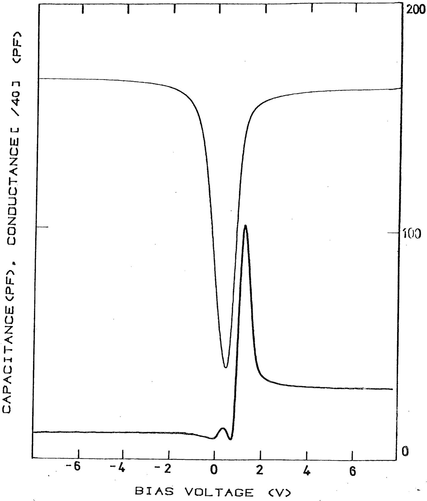
Figure 4.10 Measured admittance characteristics for epitaxial p-type sample.
