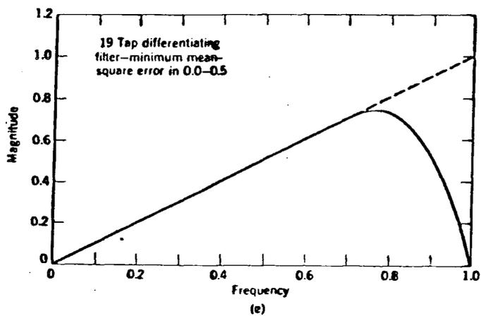
Figure 5.4 Frequency response of low noise differentiator filter. (4)
