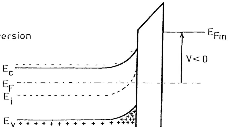
Figure 2.7 Energy band diagrams for an MOS structure depicting (a) accumulation, (b) depletion, (c) inversion.
