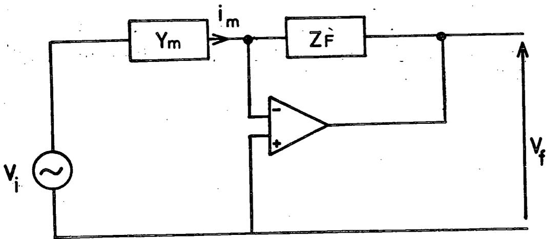
Figure 4.4 VEA measurement configuration.
