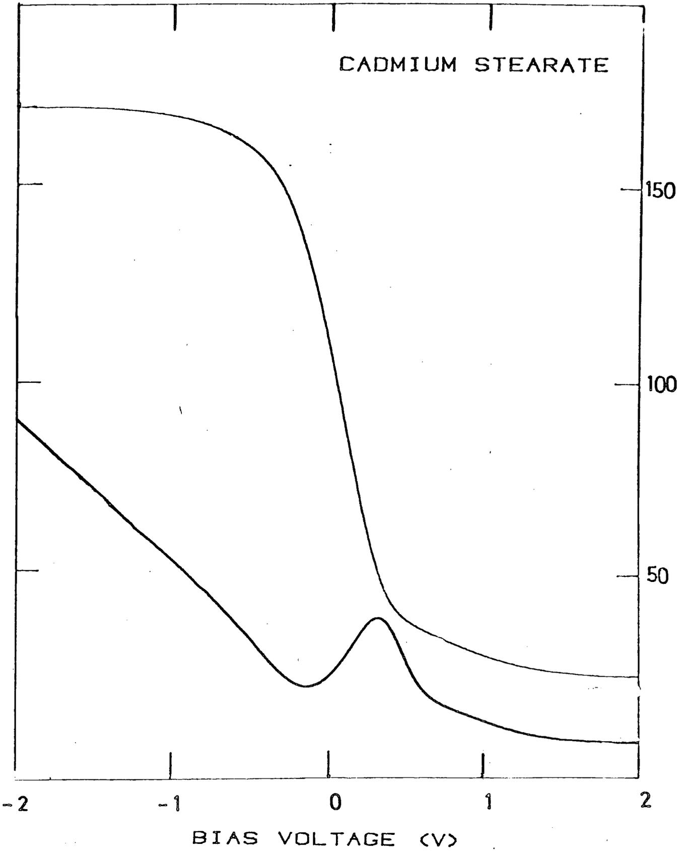
Figure 7.8 Langmuir film admittance-voltage characteristics.
