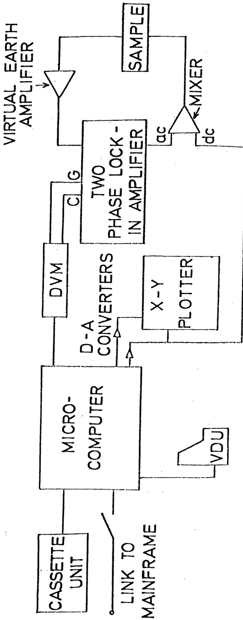
Figure 4.8 Experimental Layout for admittance measurements including microcomputer.
