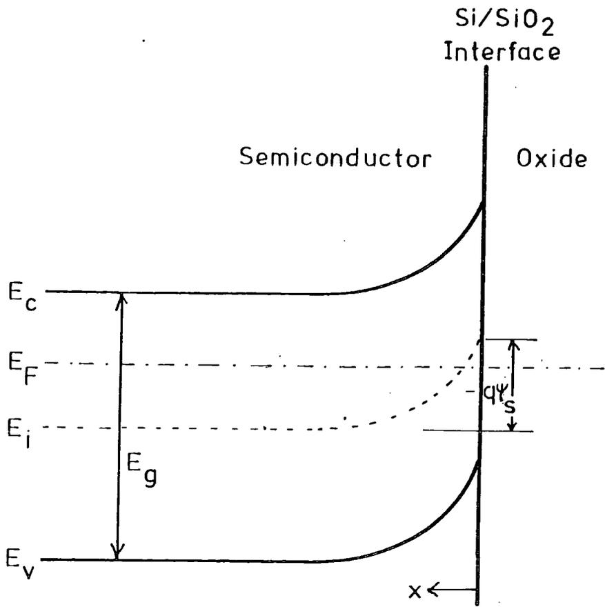
Figure 2.6 Band diagram of an MIS diode (Depletion situation).
