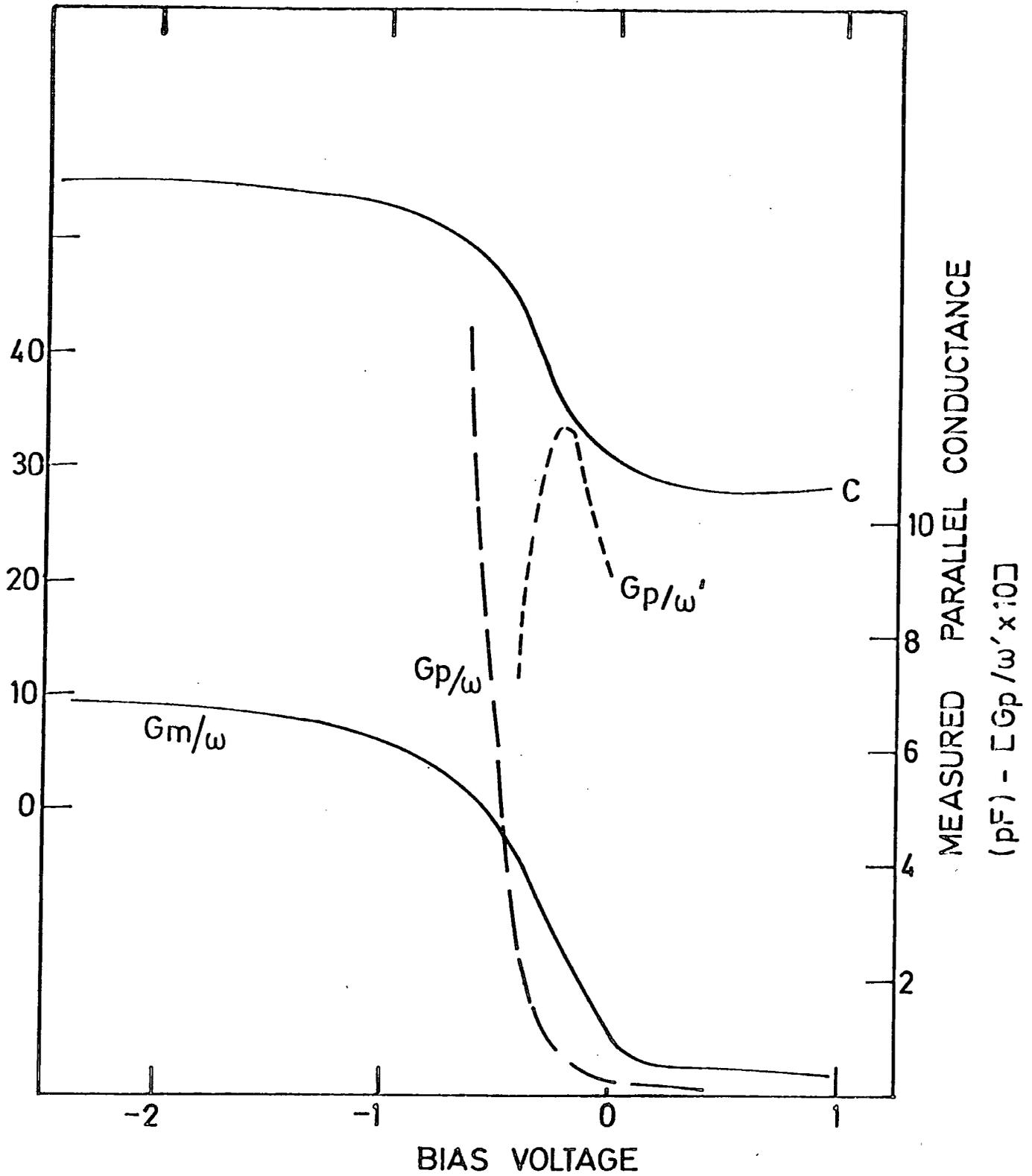
Figure 4.11 Admittance characteristics for bulk p-type sample.
