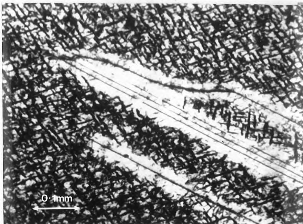
Fig. 7.13(a) Cathodoluminescent image of a ZnSe:In Sample annealed in molten zinc.
