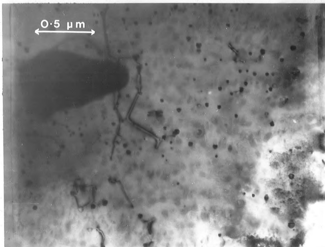
Fig. 7.21(c) The same as in figure 7.21(a) from another region showing Precipitates and Decorated Dislocations.
