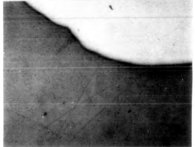
Fig. 7.4 Typical good quality top electrode
