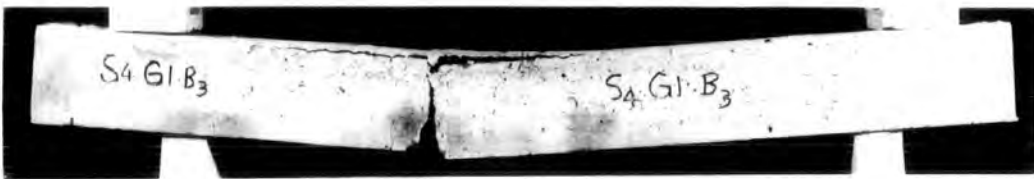
Beam made using face S_4 ( A_S = 48.3 \text{ mm.}^2 ) and core G_1
