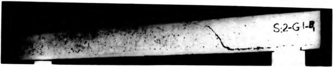
Beam of A_S = 56.0 \text{ mm}^2 (face S_2 ) and core G_1
