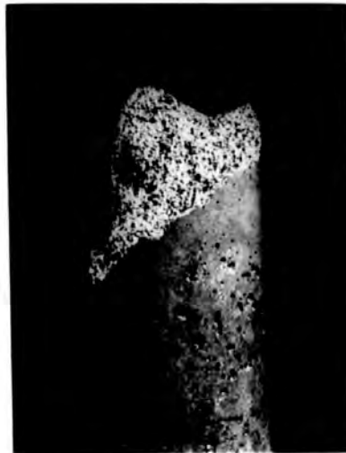
Figure (3.11) : Typical Torsion failure.
