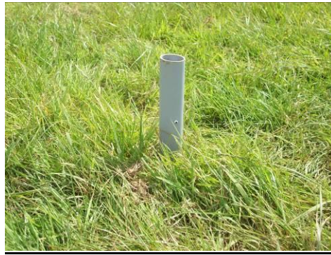
Figure 4.4 Dip-well inserted > 90cm into ground
