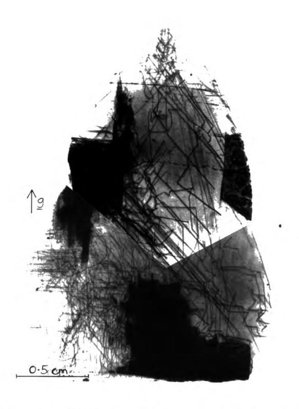
Figure 5.4: Synchrotron radiation topographs of lithium tetraborate (crystal D) using 040 reflection and wavelength of 1  $\hbox{\mbox{$\mathring{A}$}}$ .
