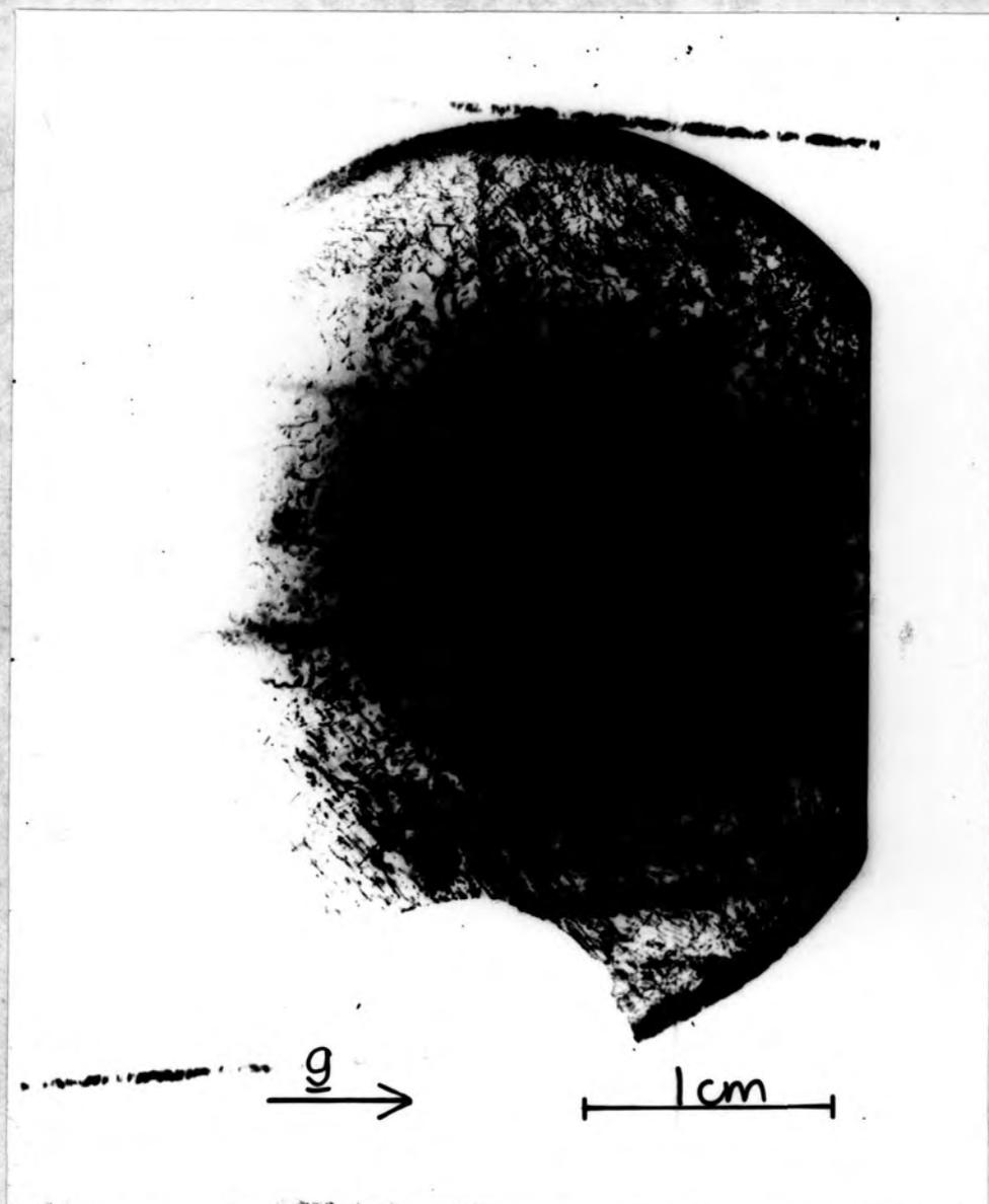
Figure 5.2: Projection topograph of lithium tetraborate (crystal B) using characteristic Mo K $\alpha$  radiation of wavelength 0.7101 Å and 040 reflection.
