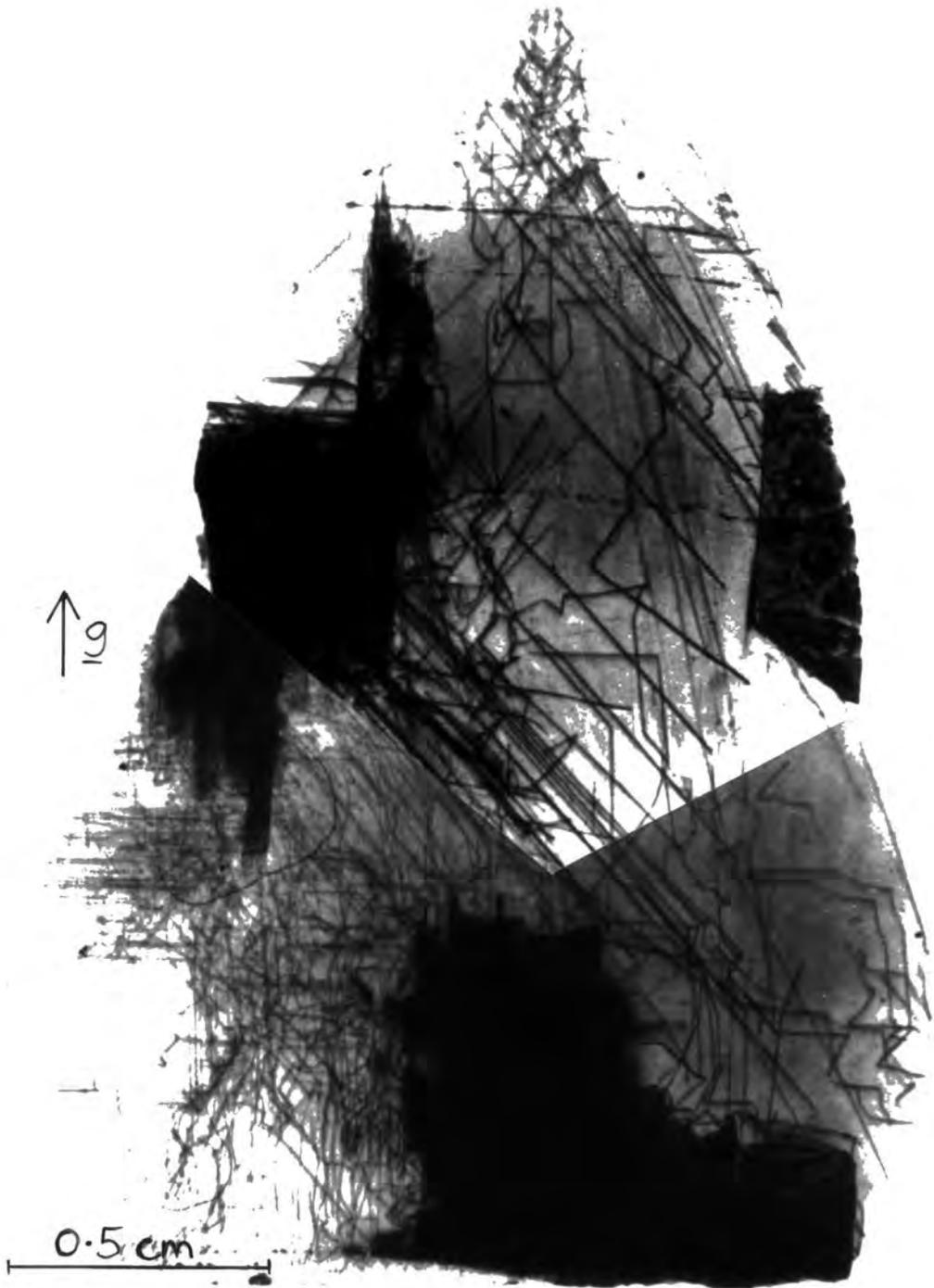
Figure 5.4: Synchrotron radiation topographs of lithium tetraborate (crystal D) using 040 reflection and wavelength of 1 Å.
