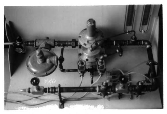
FIGURE 20 Photograph of pneumatic test rig
