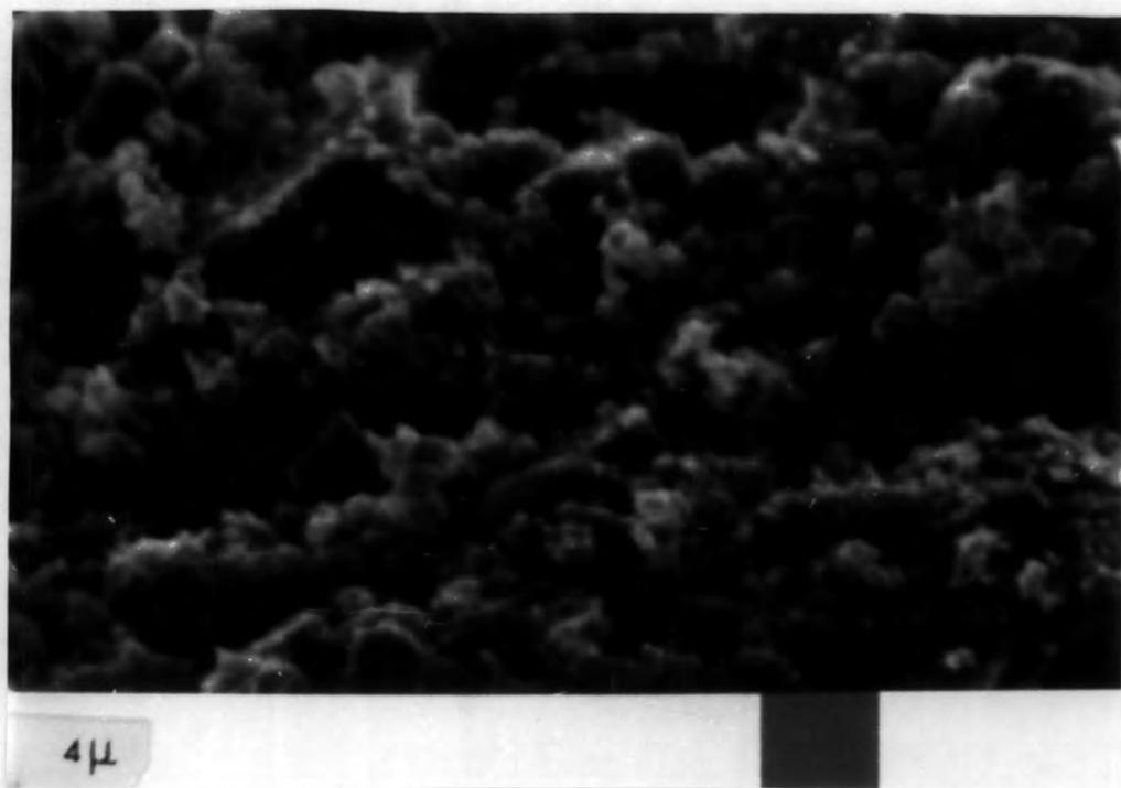
Fig.6.11: Merck CdSe powder particles after 32 minutes dry ball milling.
