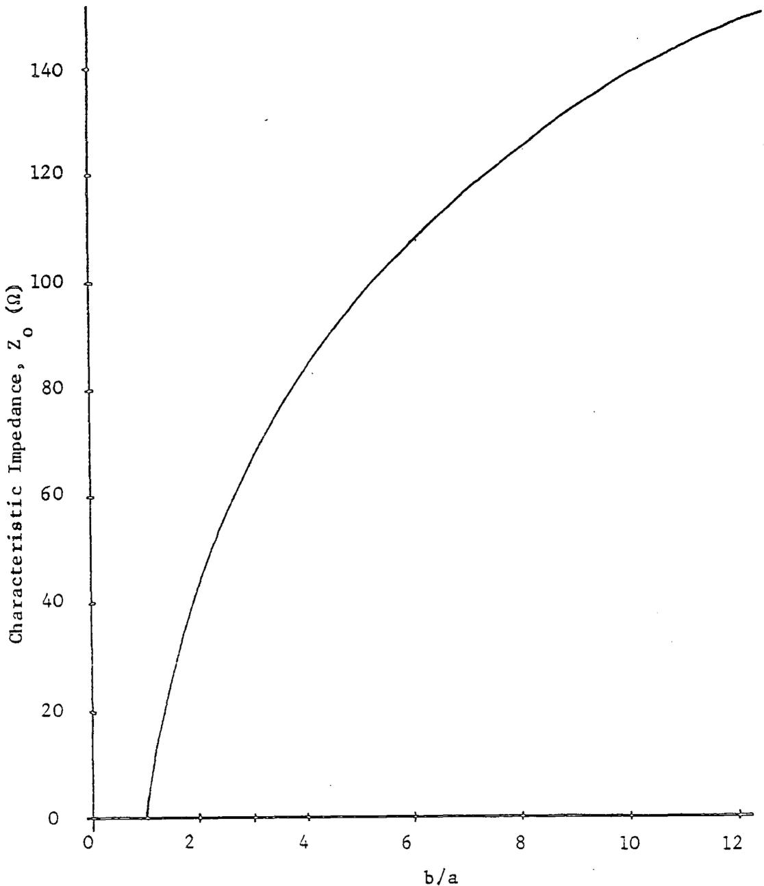
Figure 2.18  $Z_0$  versus  $b/a$  for a coaxial line
