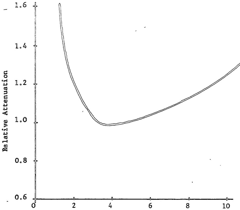
Figure 2.19 Attenuation versus  $b/a$  for a coaxial line
