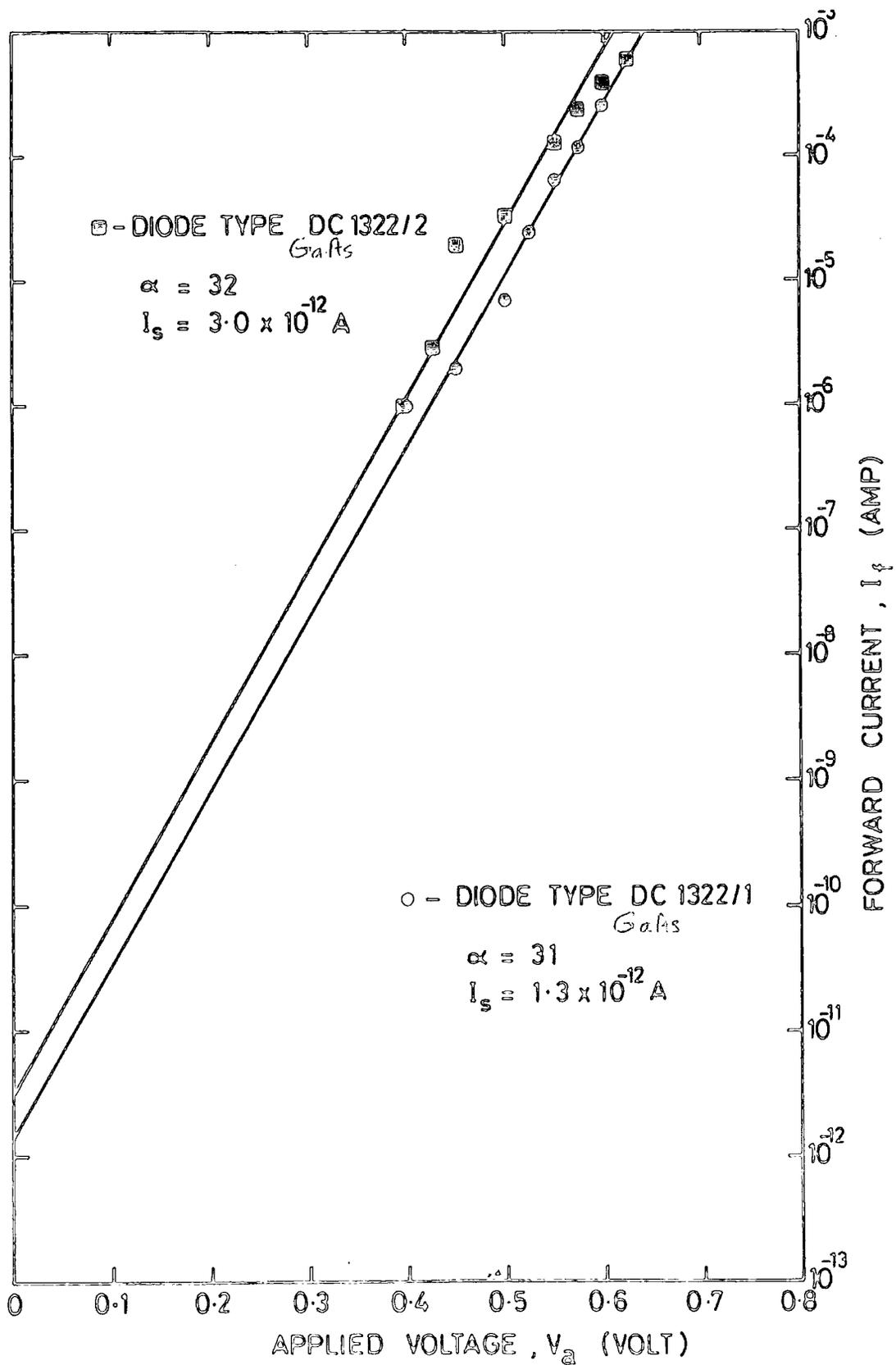
FIG. 6.2.1 DETERMINATION OF  $\alpha$  AND  $I_s$
