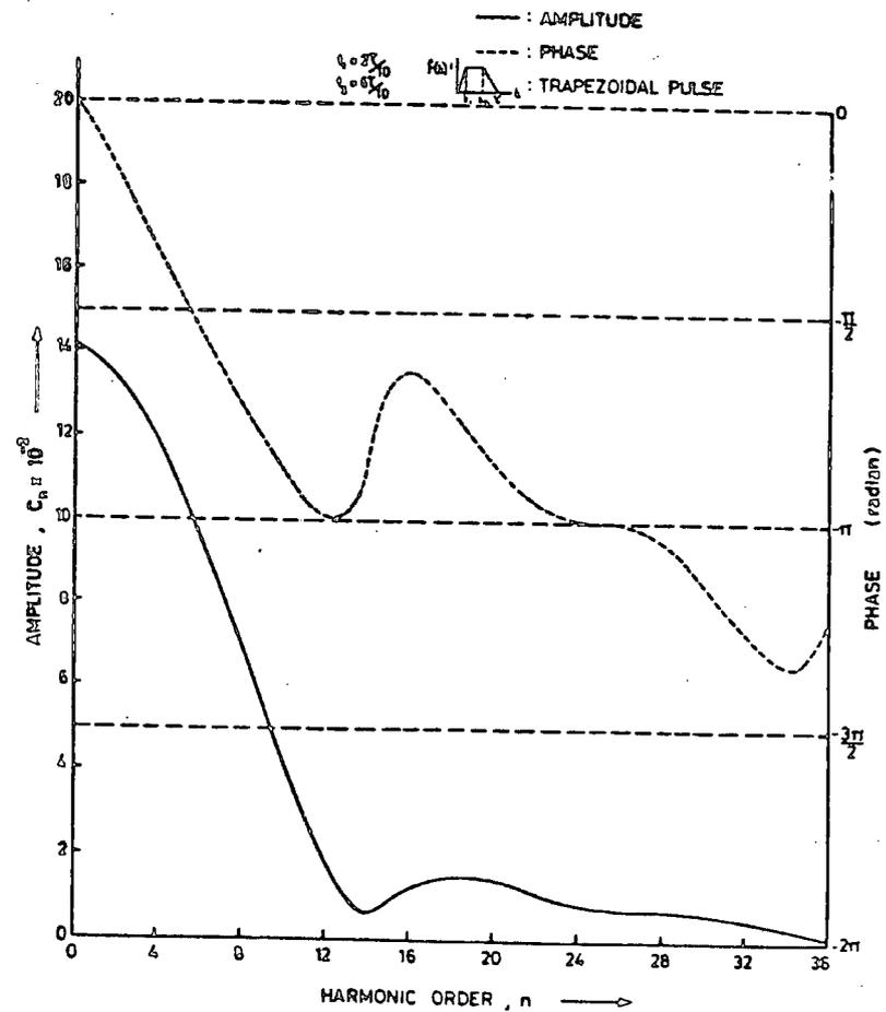
FIG. 2-6(h) AMPLITUDE AND PHASE SPECTRA
