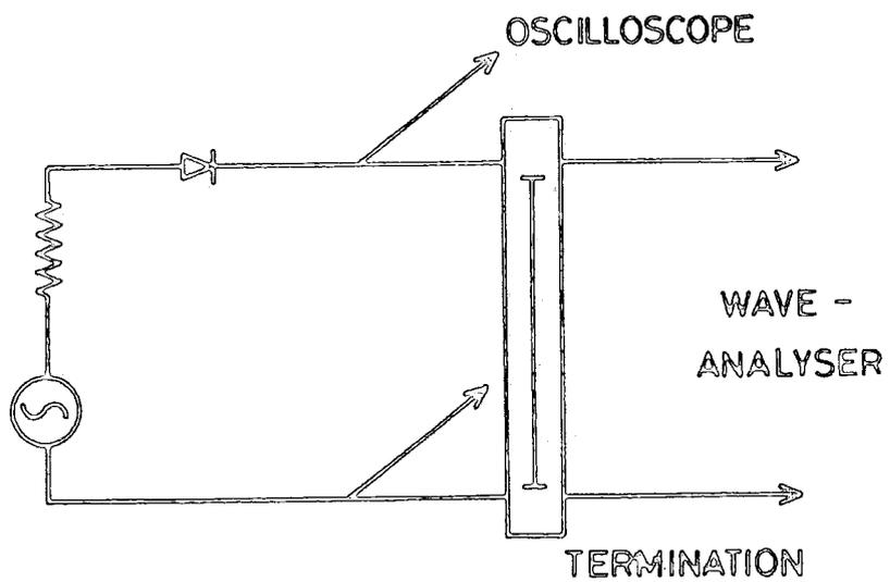
FIG. 3·3 CIRCUIT DIAGRAM - MEASUREMENT OF HARMONIC CONTENT OF A DIODE
