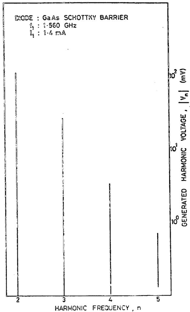
FIG. 6-3-1 AMPLITUDE SPECTRUM
