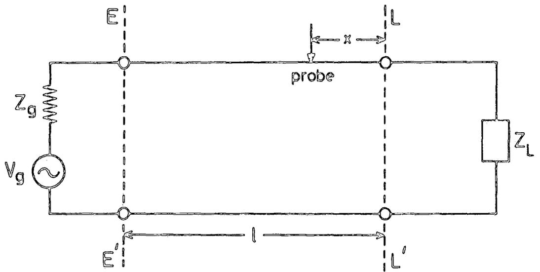
FIG.4.1 A GENERAL CIRCUIT DIAGRAM FOR A COAXIAL SLOTTED LINE
