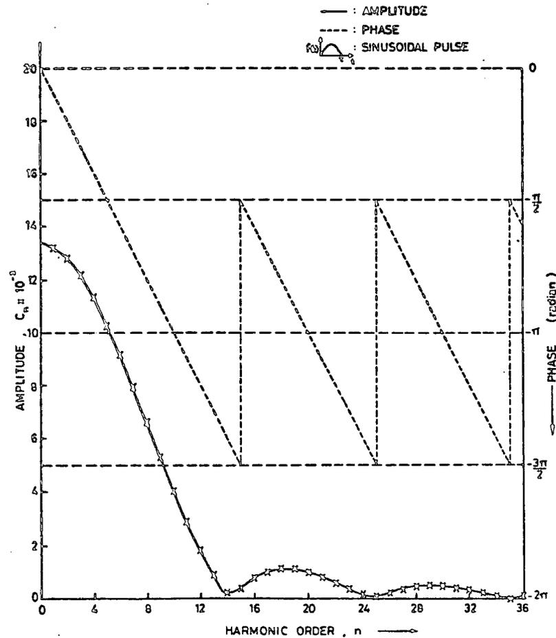
FIG. 2-5(f) AMPLITUDE AND PHASE SPECTRA
