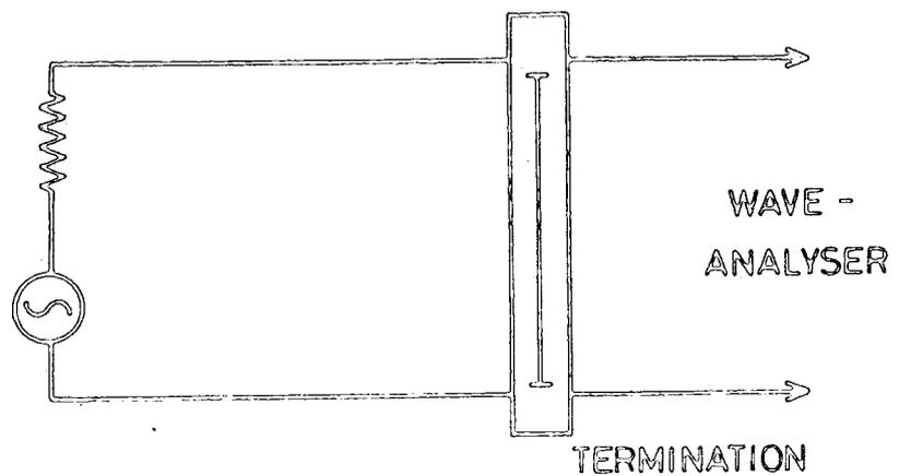
FIG. 3-2 CIRCUIT DIAGRAM - MEASUREMENT OF  $I_1$
