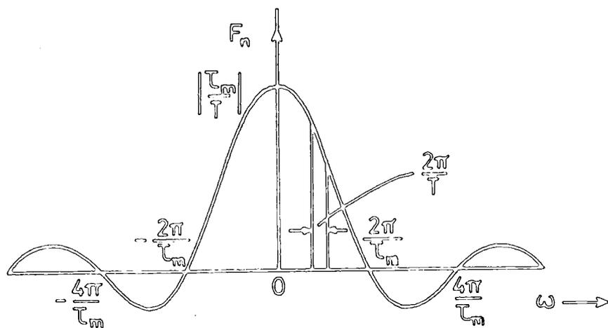
FIG. 2-3 AMPLITUDE SPECTRUM
