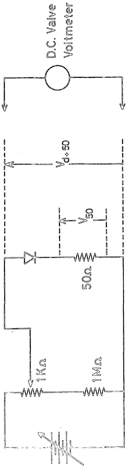
FIG. 5.1 CIRCUIT FOR THE D.C. CHARACTERISATION
