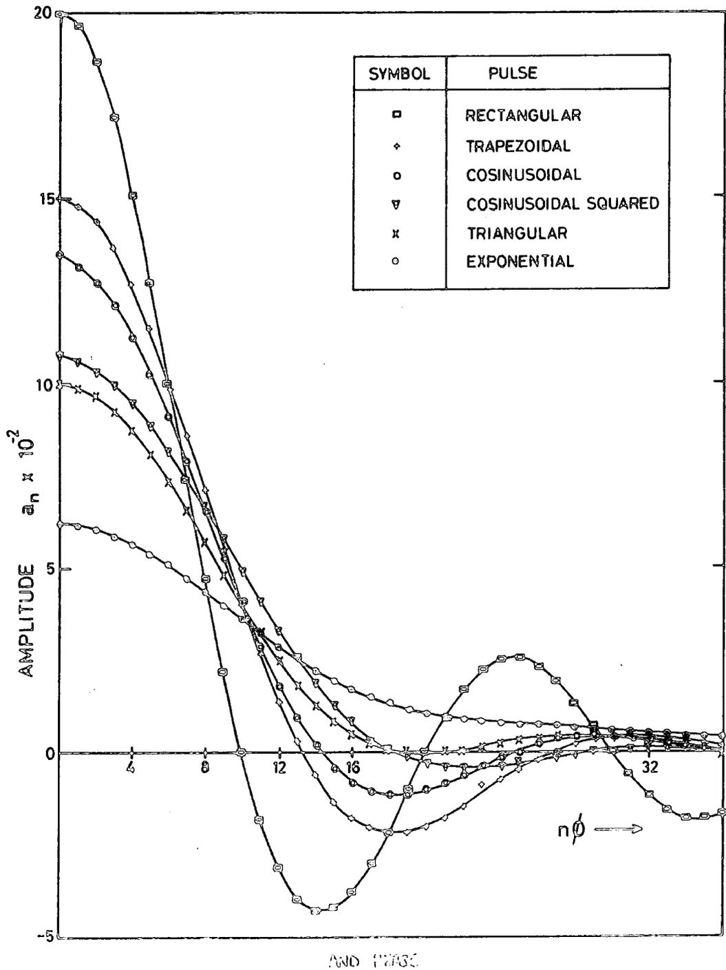
FIG. 2-4(b) AMPLITUDE/SPECTRA (symmetrical case)
