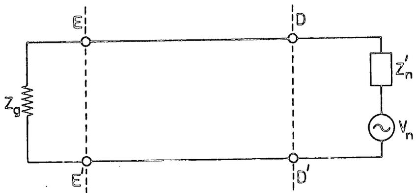
FIG.4.5 CIRCUIT DIAGRAM WHEN THE DEVICE AND THE SLOTTED LINE ARE WORKING AT THE HARMONICS
