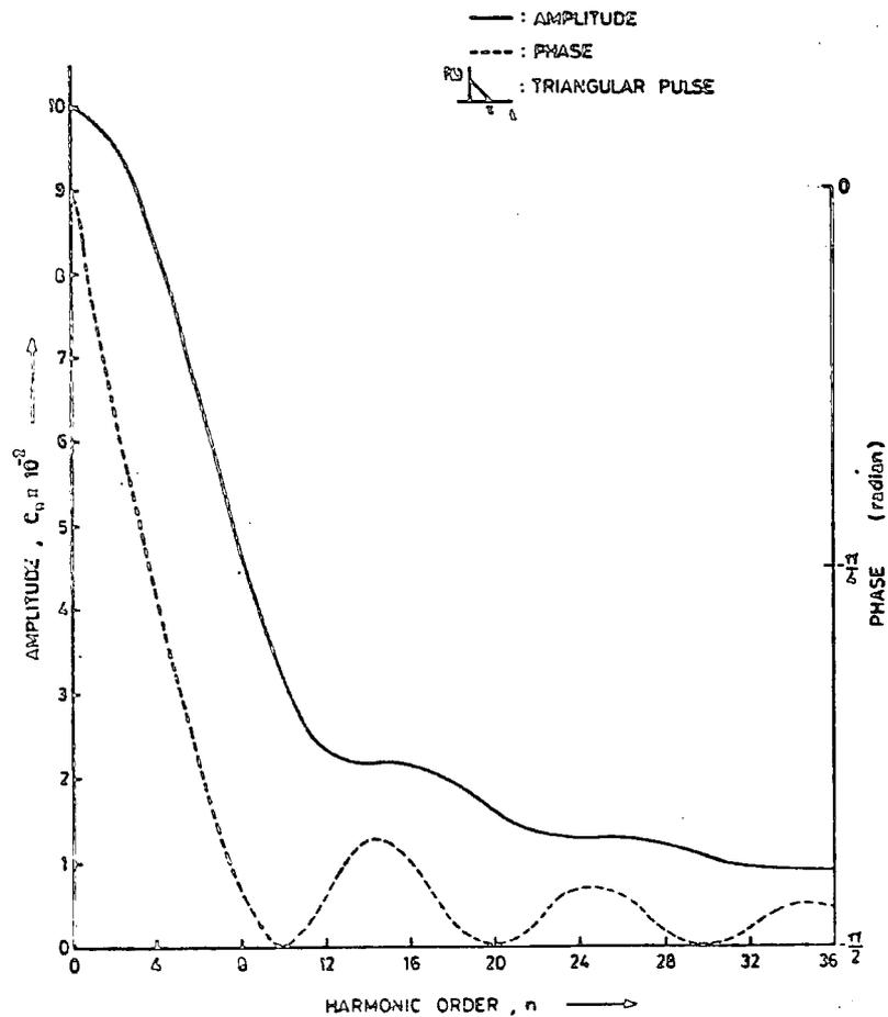
FIG. 2-6(c) AMPLITUDE AND PHASE SPECTRA
