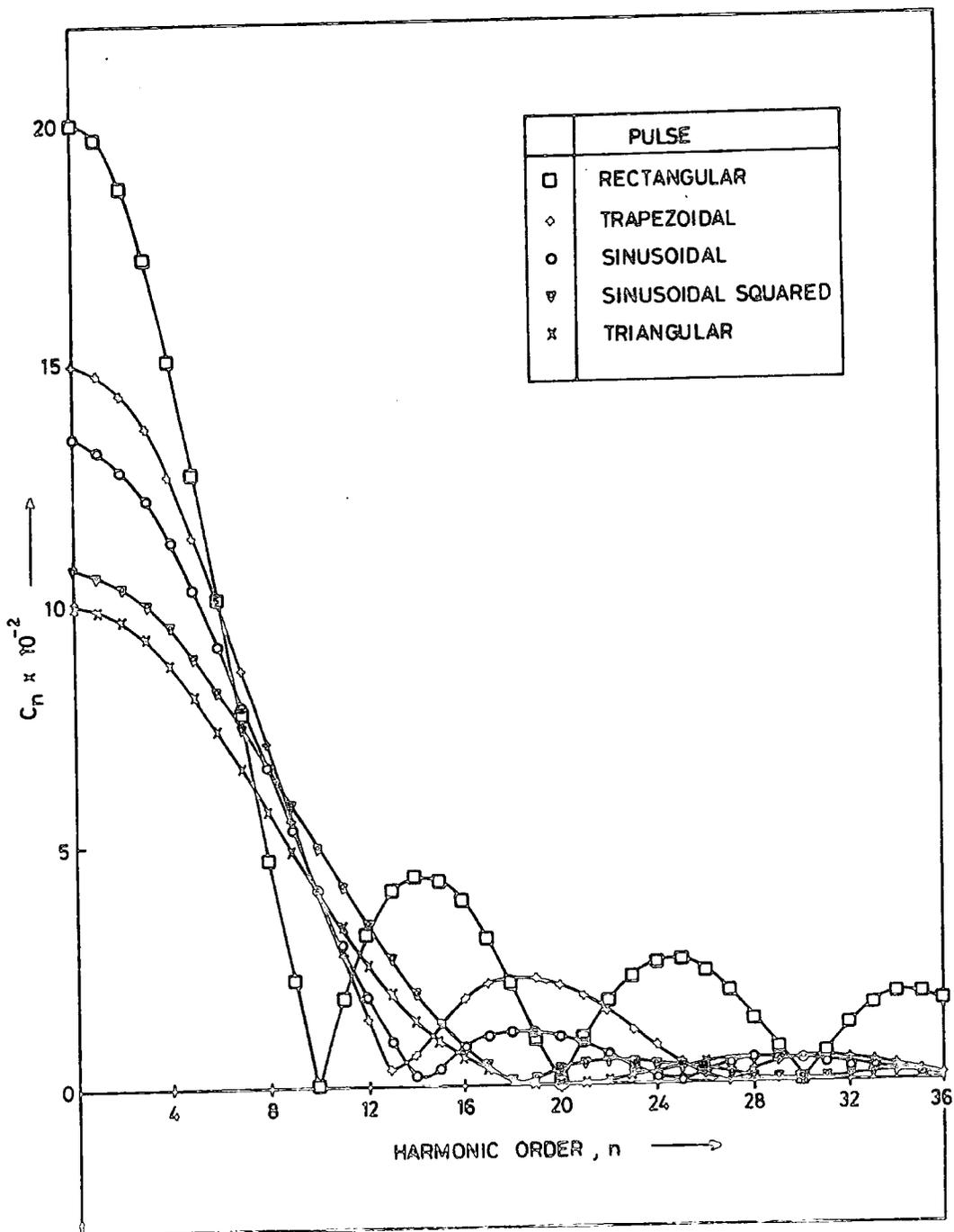
FIG. 2-5(b) AMPLITUDE SPECTRA - SYMMETRICAL CASES
