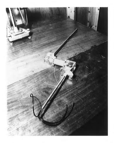
Figure 2.7(a) THE CRANKED YAW PROBE
