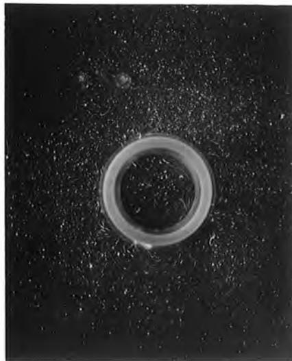
Figure 3.6(a) ROTOR WITHOUT CASING: TRANSIENT FLOWS
