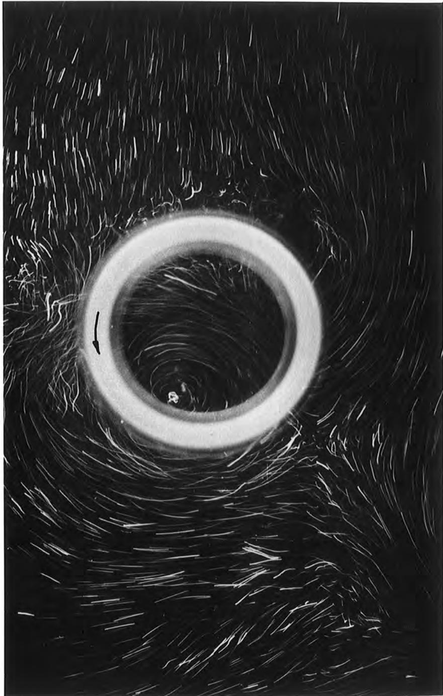
Figure 3.5 ROTOR WITHOUT CASING: STEADY STATE FLOW II
