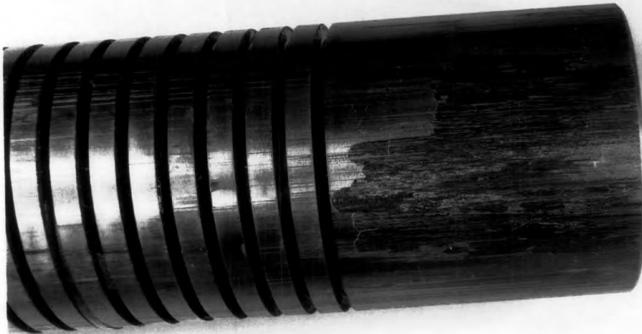
Plate 1 Scuffed Piston from a Hydrogen Compressor (Courtesy of ICI plc)
