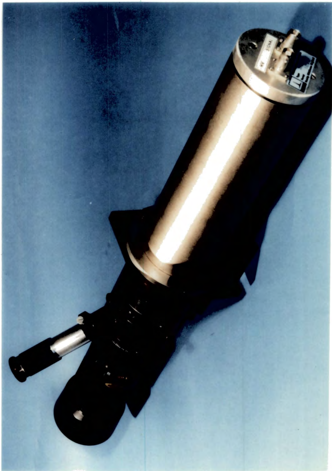
THE LDA OPTICAL SYSTEM - DETECTION OPTICS AND PHOTOMULTIPLIER TUBE ASSEMBLY
