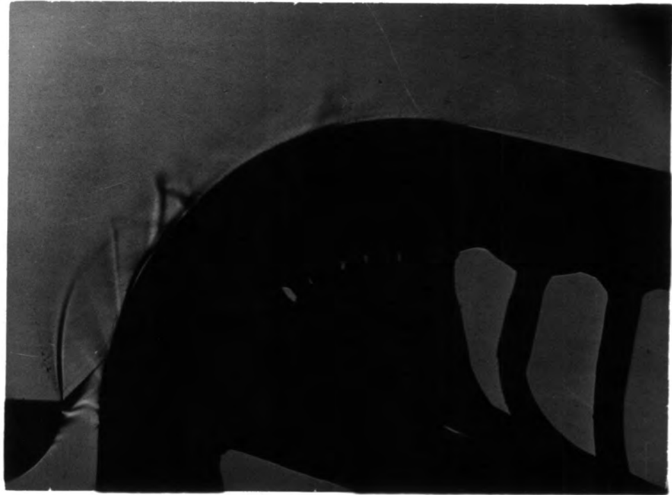
PLATE 9: Shadowgraph, Pa/Po = 0.323 Slot = 4 mm
