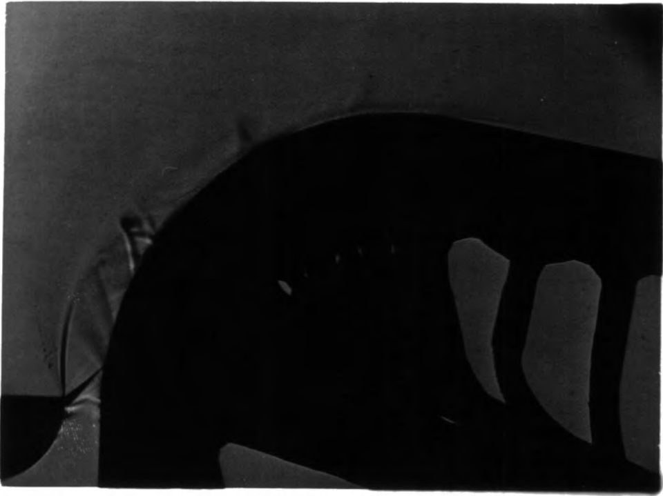
PLATE 8: Shadowgraph, Pa/Po = 0.370 Slot = 4 mm
