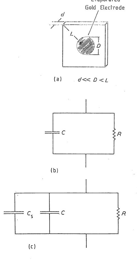
Figure 6.1. (a) General form of sample and (b) and (c) its equivalent circuits.
