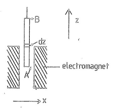
Figure 3.1. Principle of the Gouy method.
