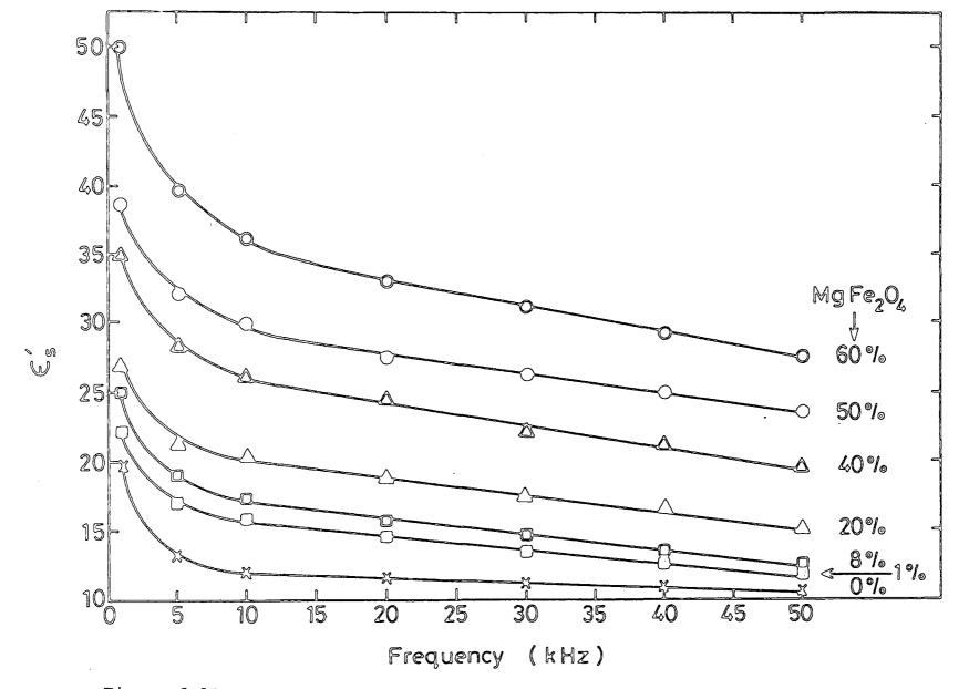
Figure 6.10. Frequency dependence of permittivity in mixed Mg Fe<sub>2</sub> O<sub>4</sub> / MgO powders.
