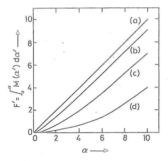
$F^{\circ}$  - Proportional to force, F, measured on Gouy magnetometer.  $\alpha$  - Proportional to field between magnet poles.
