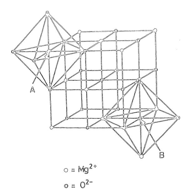
Figure 2.1. The crystal structure of MgO'showing the octahedral co-ordination of the Mg (A) and O (B) ions.
