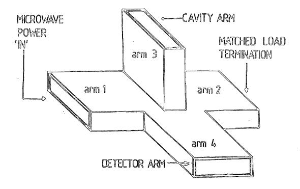
Figure 4.4. Microwave bridge (showing Varian numbering).
