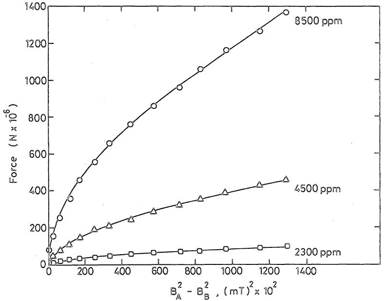
Figure 3.11. Variation of Gouy force with applied field<sup>2</sup> for Fe/MgC samples after 3<sup>1</sup>/<sub>2</sub> hours heating at 800°C in Oxygen. Figure 3.12. Form of plot of force versus field for superparamagnetics.
