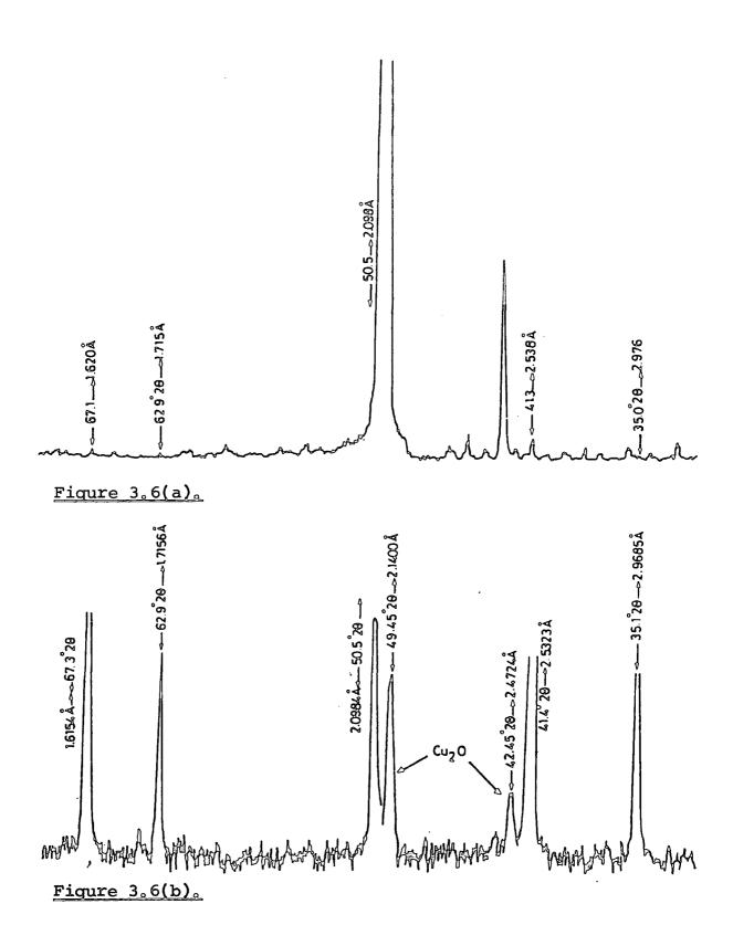
Figure 3.6. Comparison of XRD spectra of (a) Cr/MgO single crystal chippings and (b) Alpha Ventron 99% pure Magnesioferrite (Mg Fe $_2$  O $_4$ ).
