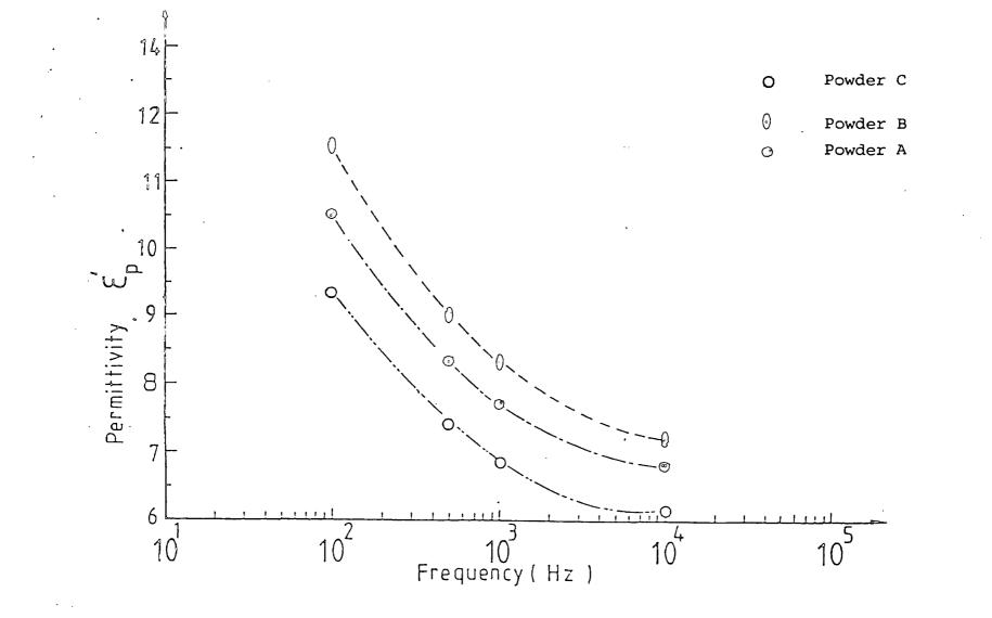
Figure 6.6. Permittivity - frequency variations for commercial MgO powders taken from the central region of a fused melt. Powder A, not heated; Powder B, with annealing heat treatment; Powder C, heat treated and quench cooled.
