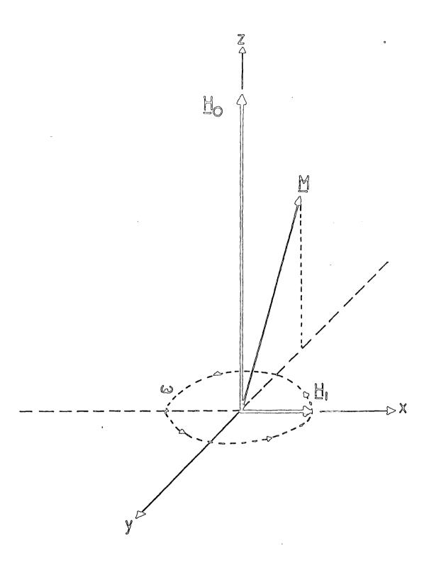
Figure 4.2. Precessing electron moment.
