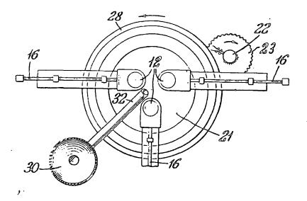
Figure 1.2. Large scale furnace for magnesia fusion. Key: graphite electrode, 12; electrode support, 14; busbars, 16; hydraulic lift, 18; steel shell, 20; melt, 21; rotation motor, 22; gear, 23; chain, 24; rollers, 26; hopper, 30; chute, 32.
