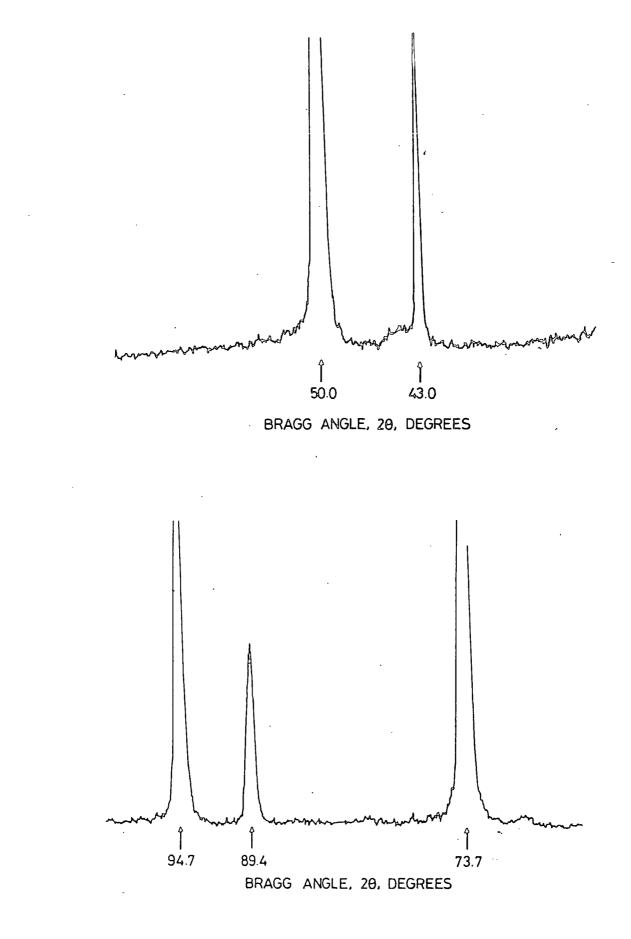
Figure 2.6. XRD spectrum of pure MgO.
