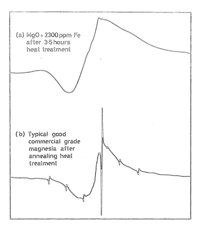
Figure 5.9. Comparison of (a) deliberately doped Fe/MgO after 3½ hours at 800%C in oxygen with (b) good commercial magnesia after annealing heat treatment.
