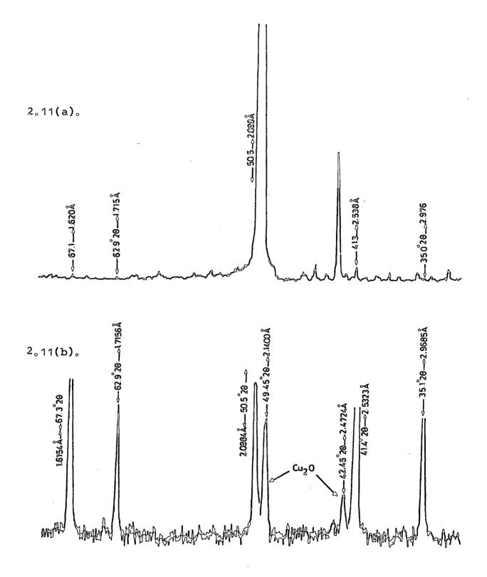
Figure 2.11. Comparison of the XRD spectra of (a) good commercial magnesia with (b) pure magnesioferrite.
