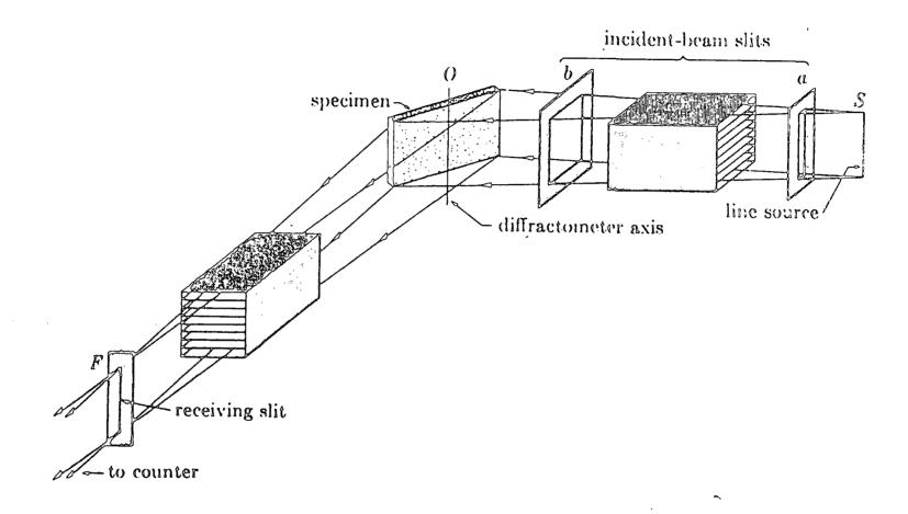
Figure 2.3. Arrangement of slits in a diffractometer.
