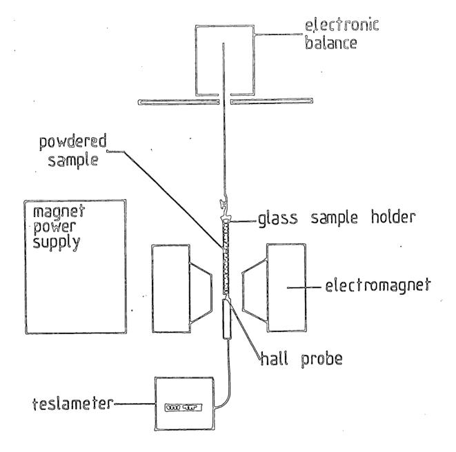
Figure 3.3. Apparatus for measuring volume susceptibility.
