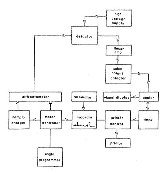
Figure 2.5. Block diagram of the XRD system.
