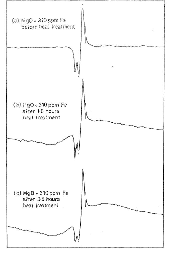
Figure 5.7. Samples of Fe/MgO before and after heating at 800°C in Oxygen.
