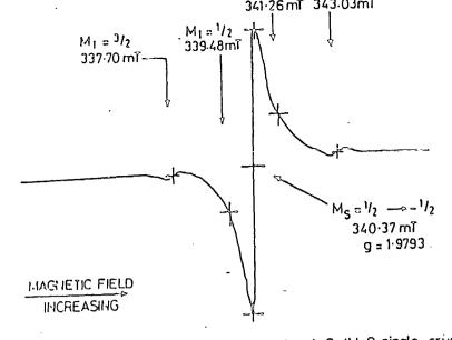
(a) .Detail of ESR spectrum of powdered Cr/MgO single crystal; 800 ppm Cr, 293K, 9-429 GHz.
