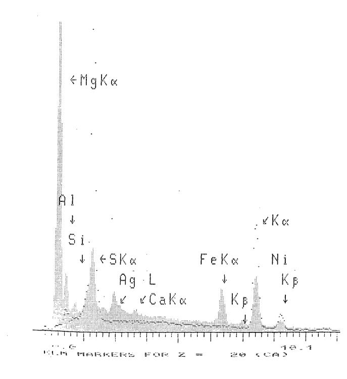
Figure  $2_{\circ}10_{\circ}$  EDAX trace for material of the black region of the fusion, (scanning  $0_{\circ}5 \text{ mm}^2$  of the surface "-----" scanning  $1_{\circ}0 \text{ mm}^2$  of the surface ".....").
