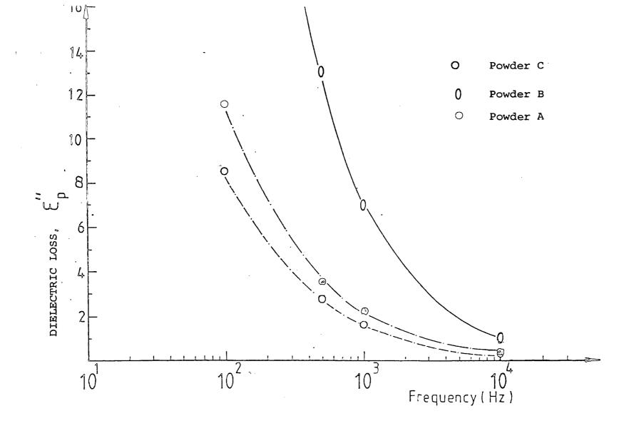
Figure 6.7. Dielectric loss - frequency variation for commercial MgO powders taken from the centre of a fused melt. Powder A, unheated; Powder B, annealing heat treatment; Powder C, heat treated and quench cooled.
