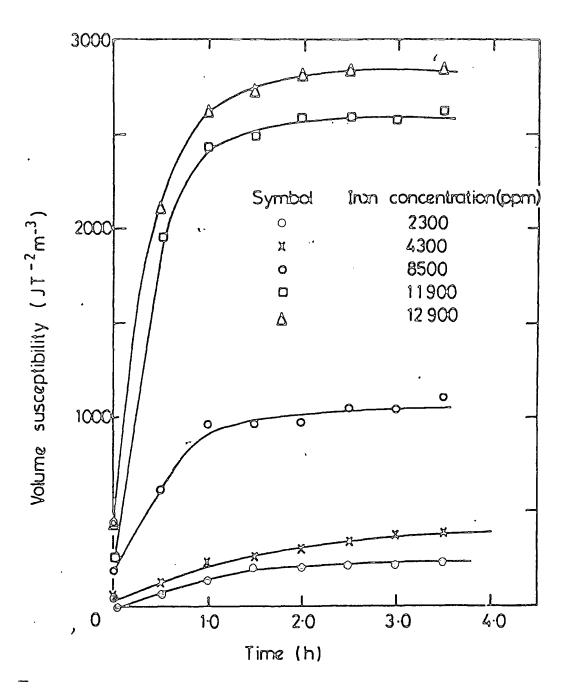
Figure 3.7. Variation of volume susceptibility with lenght of heat treatment for Fe/MgO samples.
