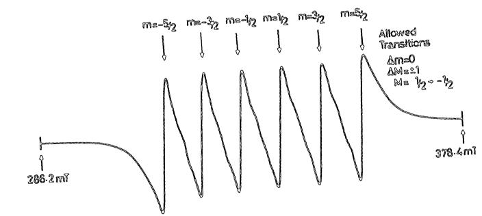
Figure 4.9(b). ESR spectrum of powdered Mn/MgO; 2900 ppm Mn, 9.380 GHz, 293 K. 4.8.4 E.S.R. Spectra of N1/MgO
