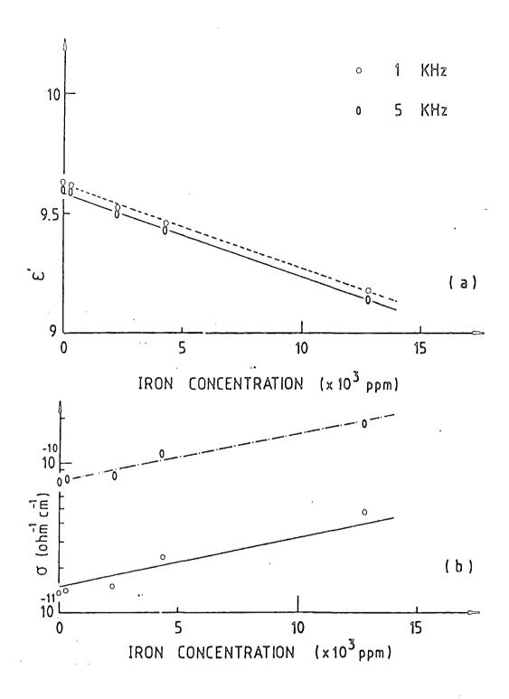
Figure 6.4. The dependence of (a)  $\varepsilon^{0}$  and (b)  $\sigma$  on Fe concentration.
