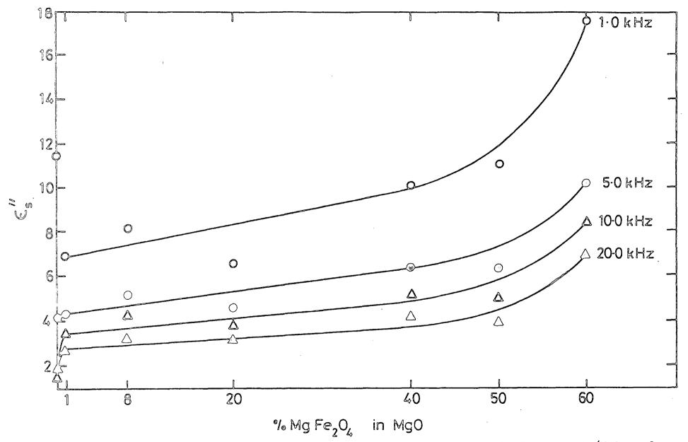
Figure 6.9. The dielectric loss - concentration dependence of mixed Mg Fe $_2$  O $_4$ /MgO powders.
