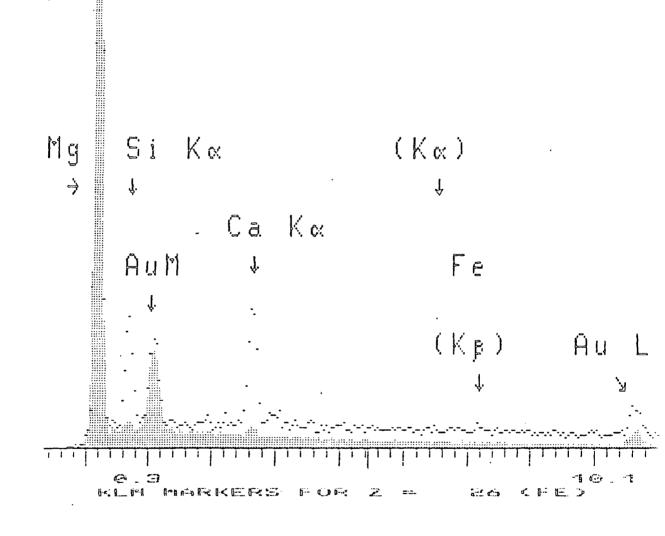
Figure 2.9. EDAX trace for material from the centre of the fusion, (scanning  $0.5 \text{ mm}^2$  of the surface "-----" scanning 1.0 mm<sup>2</sup> of the surface "....").
