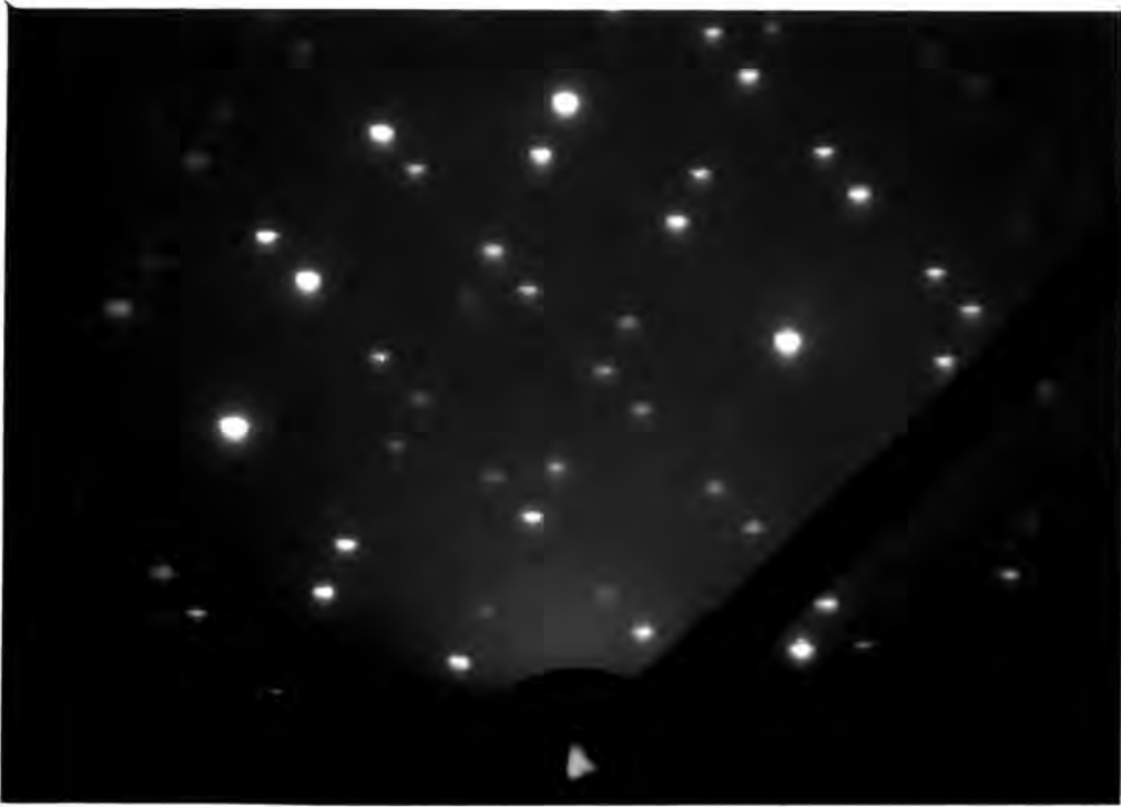
Figure 6.5a [110] RHEED pattern from a surface intersected by twins on the (\bar{1}\bar{1}\bar{1}) and (\bar{1}11) planes.
