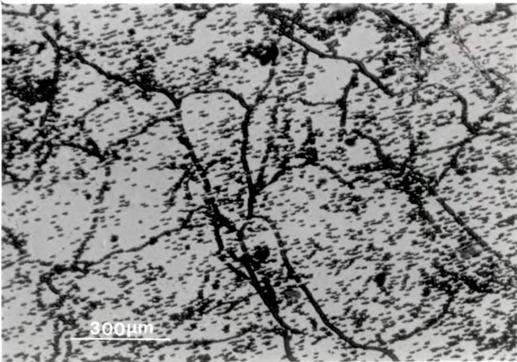
Figure 8.2 Sub-grain boundaries etched with Inoue's EAg-1 reagent.
