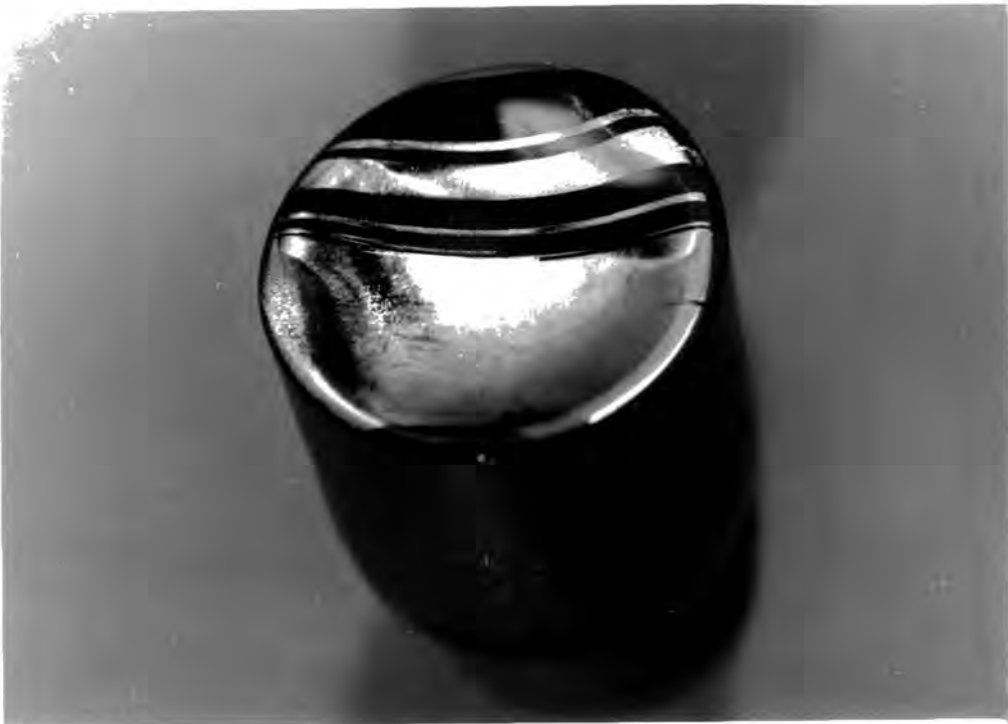
Figure 6.1 Growth face of a boule showing twin lamellae.
