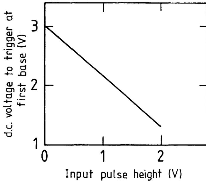
Figure A.2: The discriminator circuit and its relationship between the d.c. level on the first transistor and the minimum input pulse height required to trigger the circuit.
