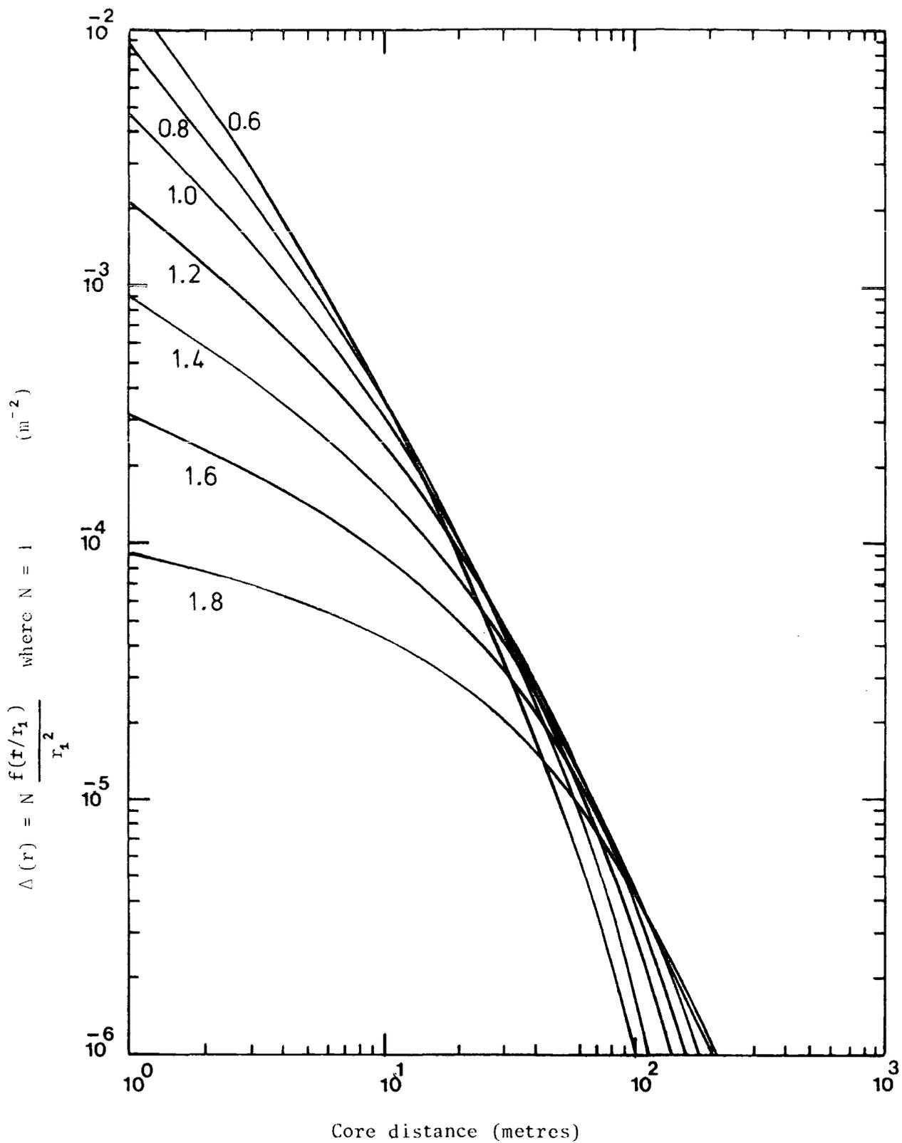
Figure 5.5: The lateral distribution of electrons in showers of unit size in air at level ( $r_0 = 79\text{m}$ ). The number attached to each curve is the age parameter (s) of the shower.
