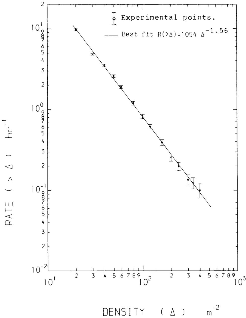
Figure 4.8: The integral density spectrum of electrons at sea level measured by using a microcomputer data acquisition system. The solid line is the best fit line for the experimental points.
