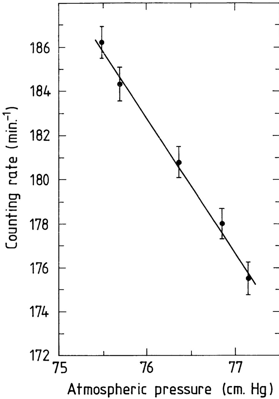
Figure 3.14: Variation of counting rate with atmospheric pressure.
