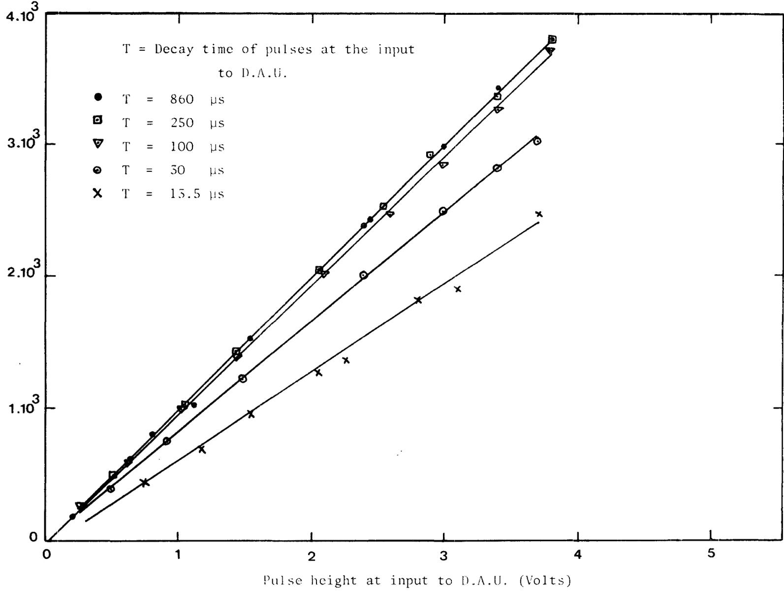
Figure 2.7 : Calibration of the data acquisition unit using a stretcher amplifier to generate pulses of different decay time at the input to the D.A.U. Pulses of decay time 10 μs at the input to the stretcher amplifier were used.
