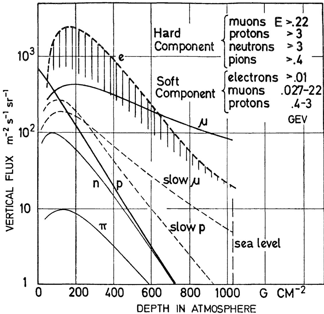
Figure 3.1 : The vertical fluxes of different components of cosmic rays within the atmosphere.
