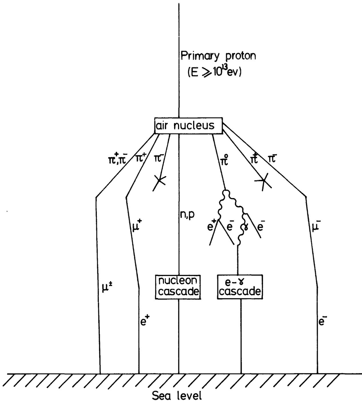
Figure 5.1: Diagram showing the major processes taking place in the atmosphere when an extensive air shower is observed at sea level.
