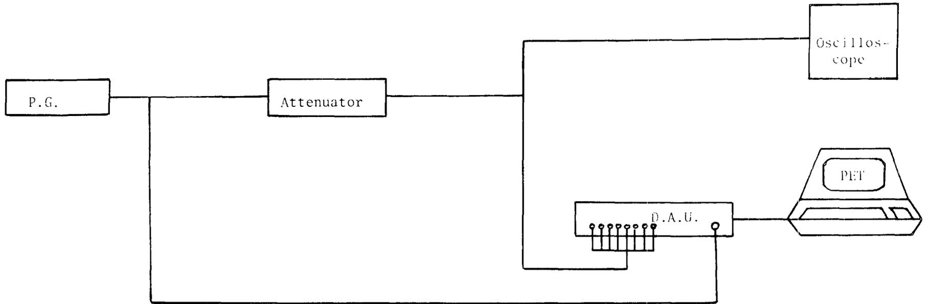
Figure 2.2 : Block diagram of the system used to calibrate the data acquisition unit (D.A.U.) with no stretcher amplifier.
