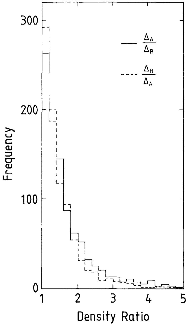
Figure 4.10: The frequency distribution of the ratio of the density of particles through one of scintillators to the other. The number of density ratios = 1816.
