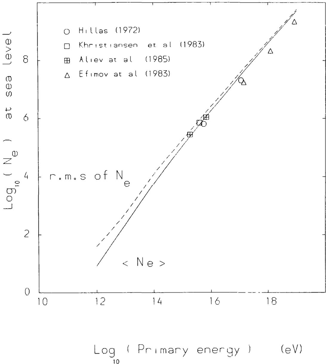
**Figure 6.18:** Average size of showers at sea level as a function of the primary proton energy, calculated by simulation program MC007. The solid curve is the average of 1000 simulated results and the dashed curve is the root mean squares of the same sample. Some experimental data are plotted for comparison.
