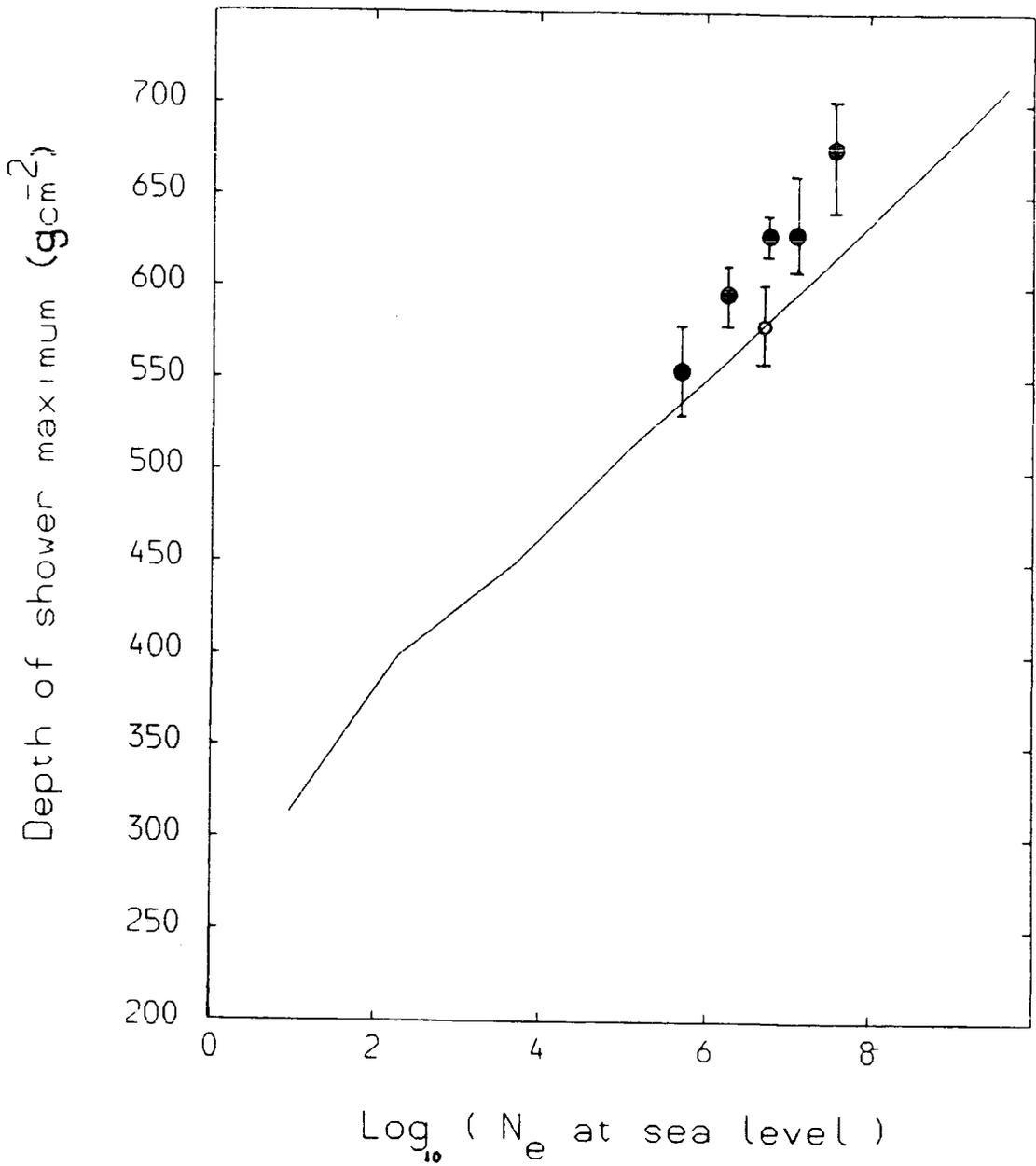
Figure 6.22: The depth of shower size maximum as a function of shower size at sea level. It is the depth at which the average longitudinal development of electron number reaches its maximum. Experimental points, due to Inoue et al.(1985) are plotted with the present simulation result.
