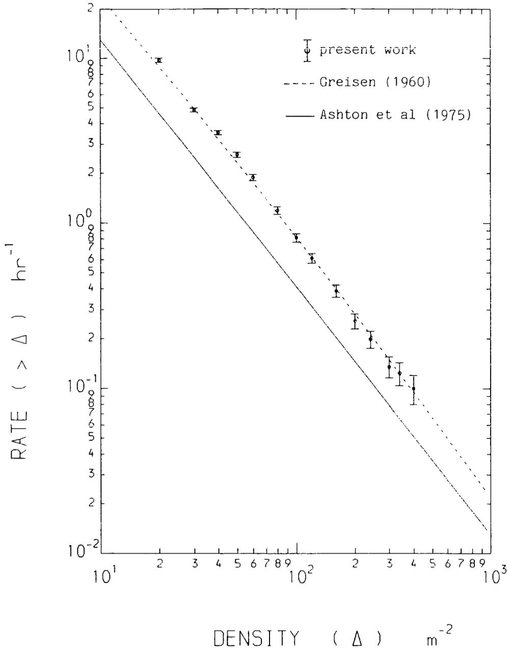
Figure 4.9: The integral density spectrum of electrons at sea level measured by using a microcomputer data acquisition system and compared with the results given by Greisen (1960) and Ashton et al (1975).
