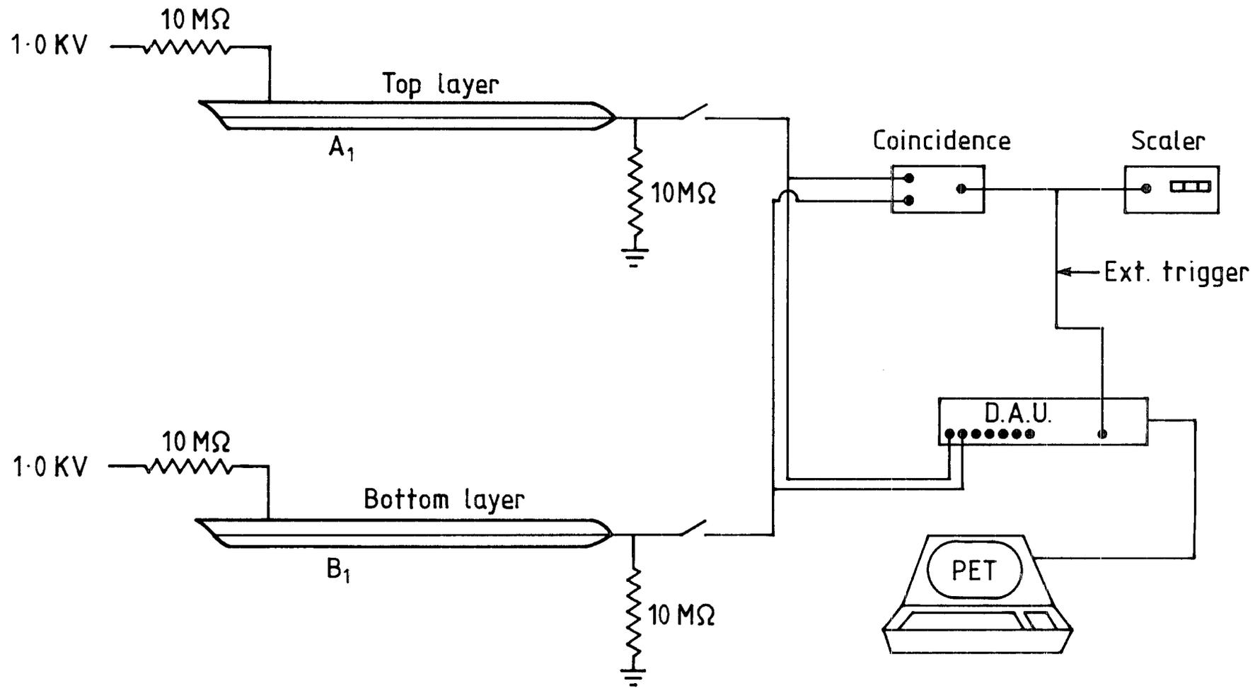
Figure 3.5: Block diagram of Geiger-Müller cosmic ray telescope.
