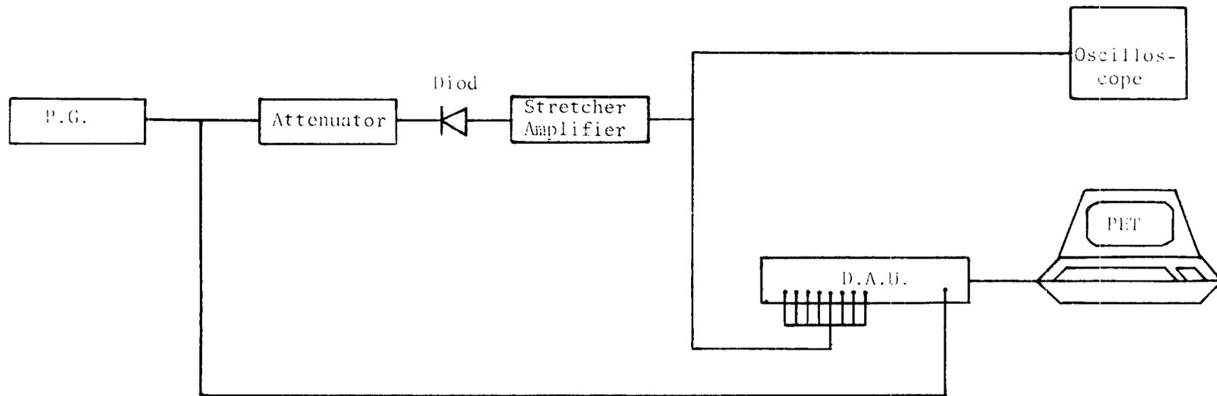
Figure 2.6 : Block diagram of the system used to calibrate the data acquisition unit (D.A.U.) using a stretcher amplifier to generate pulses of different decay time at the input to the D.A.U.
