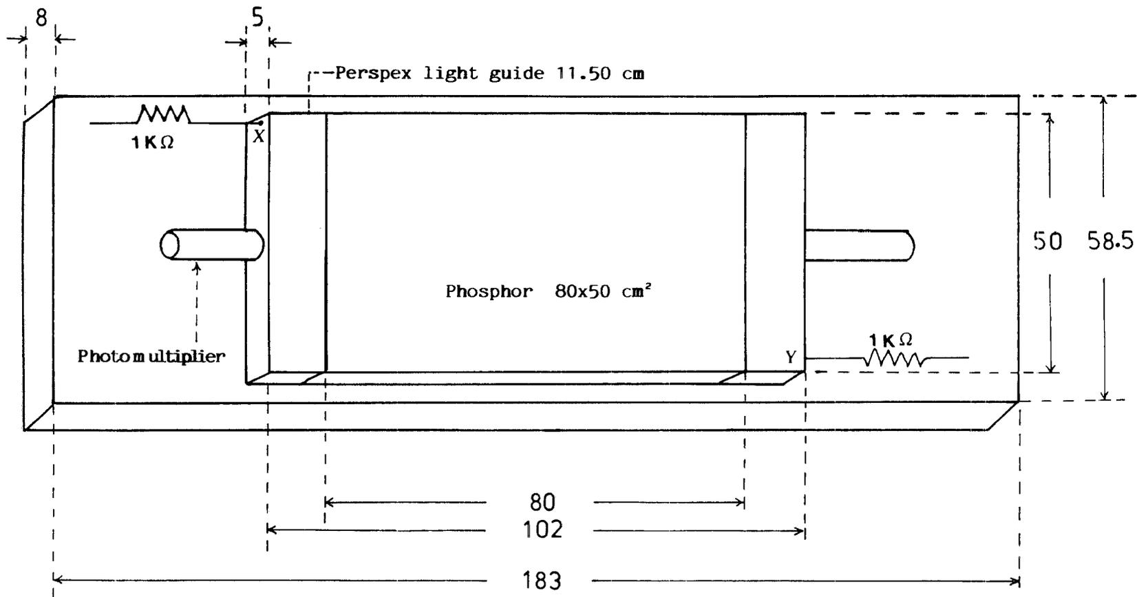
**Figure 4.2:** Design of plastic scintillation counter.
