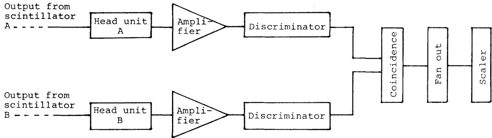
Figure 4.6: Block diagram of the system used to measure the density spectrum in the region  $2.7 - 37 \text{ m}^{-2}$ .
