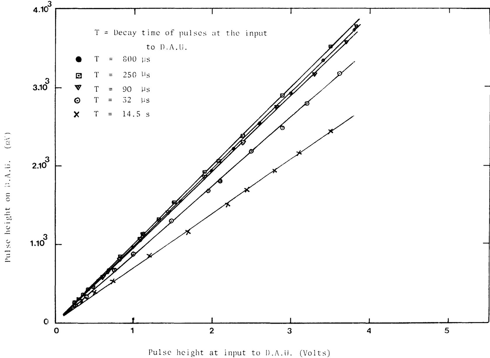
Figure 2.8 : Calibration of the data acquisition unit using a stretcher amplifier to generate pulses of different decay time at the input to the D.A.U. Pulses of decay time 1  $\mu$ s at the input to the stretcher amplifier were used.
