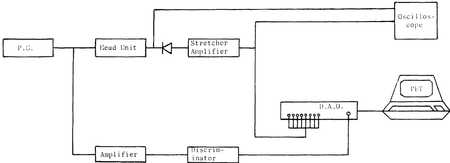
Figure 2.9 : Block diagram of the final workable system used for calibration of the combination of the stretcher amplifier and the data acquisition unit (D.A.U.)
