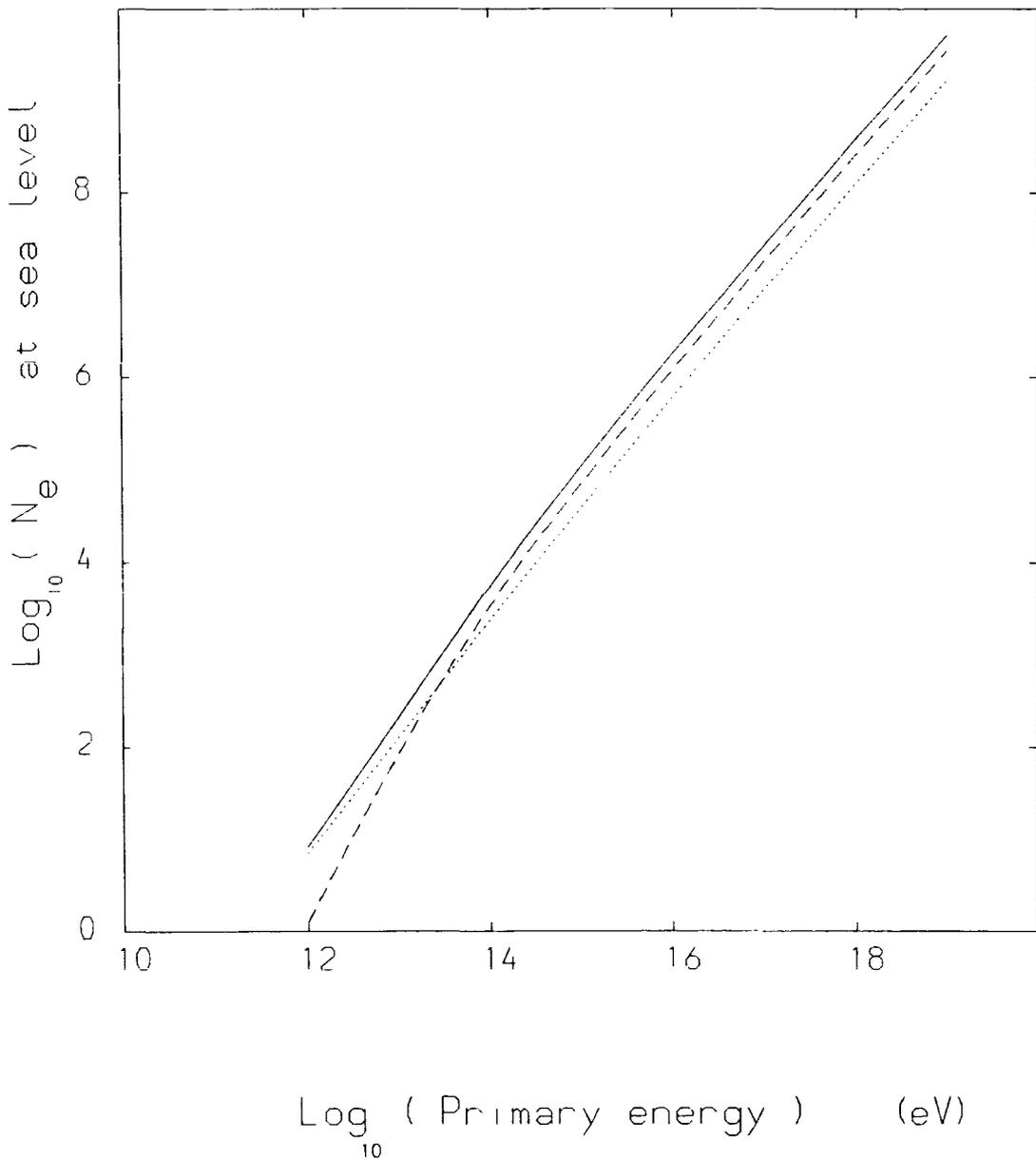
**Figure 6.17:** Average size of showers at sea level as a function of the primary proton energy, calculated by simulation. Solid curve is the simulation by program MC007. Dashed curve is the simulation by MC006 (number of electrons produced by pion cascade originating from charged pions). Dotted curve is the simulation by MC004 (number of electrons produced by neutral pion production only)
