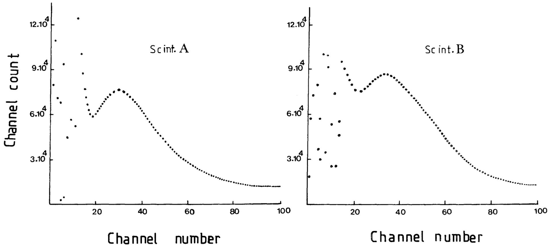
Figure 4.3: Typical single particle cosmic ray peak for each of scintillators A and B as displayed on the pulse height analyser.
