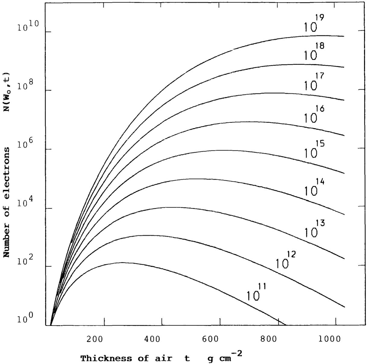
Figure 5.4: Mean number of electrons as a function of air thickness for showers initiated by photons. Photon energies,  $W_0$ , are shown on the graph, in eV.
