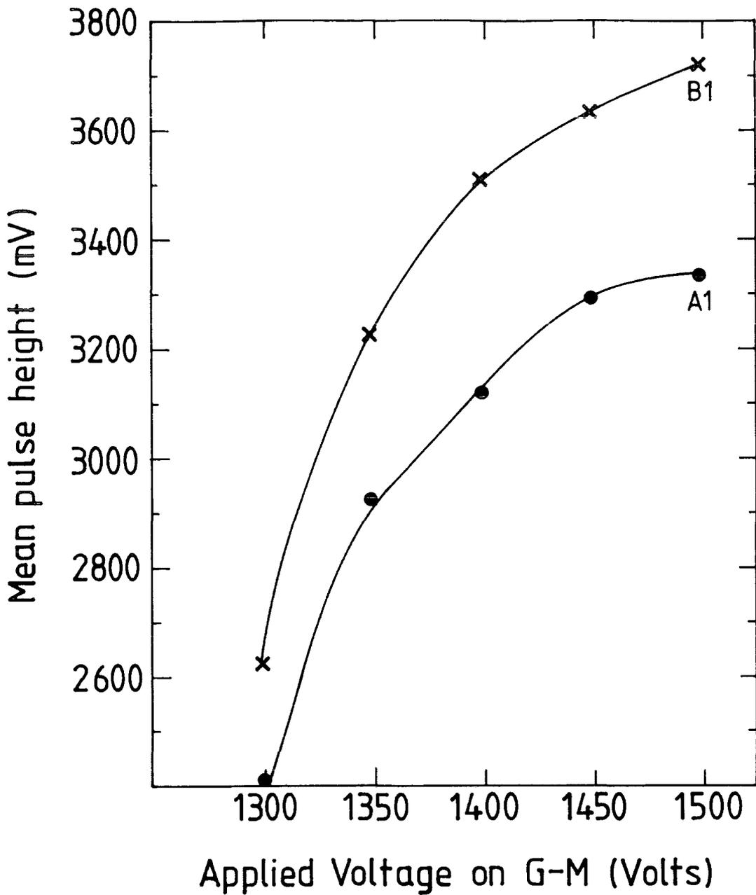
Figure 3.8: Effect of applied voltage on the pulse height of Geiger-Müller counters  $A_1$  and  $B_1$ .
