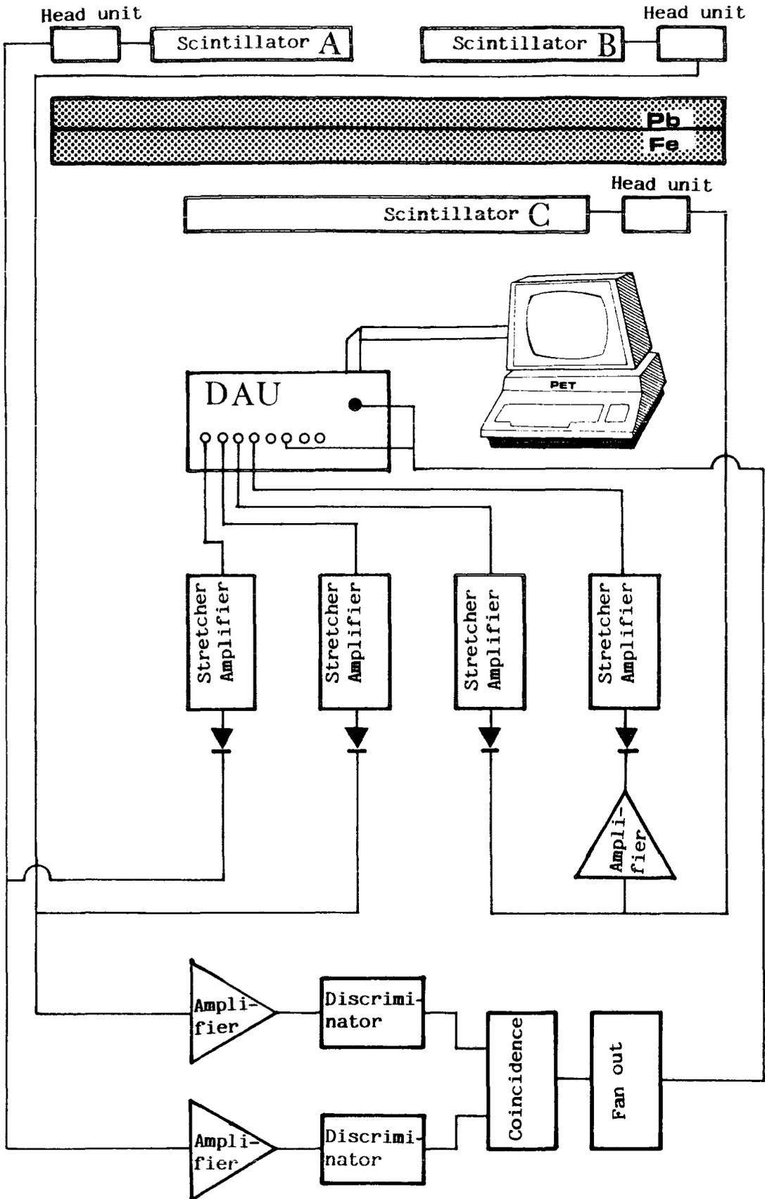
Figure 4.5: Block diagram of the system used in the present experiment.
