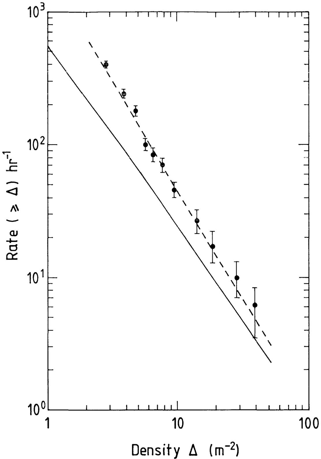
Figure 4.7: The integral density spectrum of electrons at sea level measured by using discriminators, two-fold coincidence and scaler.
