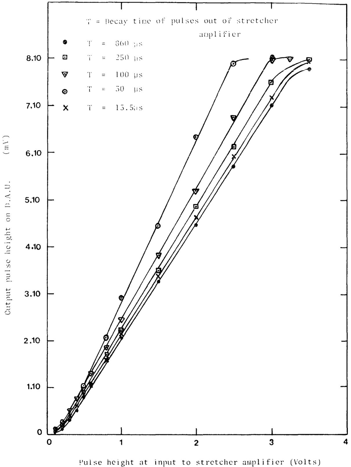
Figure 2.10: Calibration of the combination of stretcher amplifier and the data acquisition unit using  $10 \mu s$  decay time input exponential pulses.
