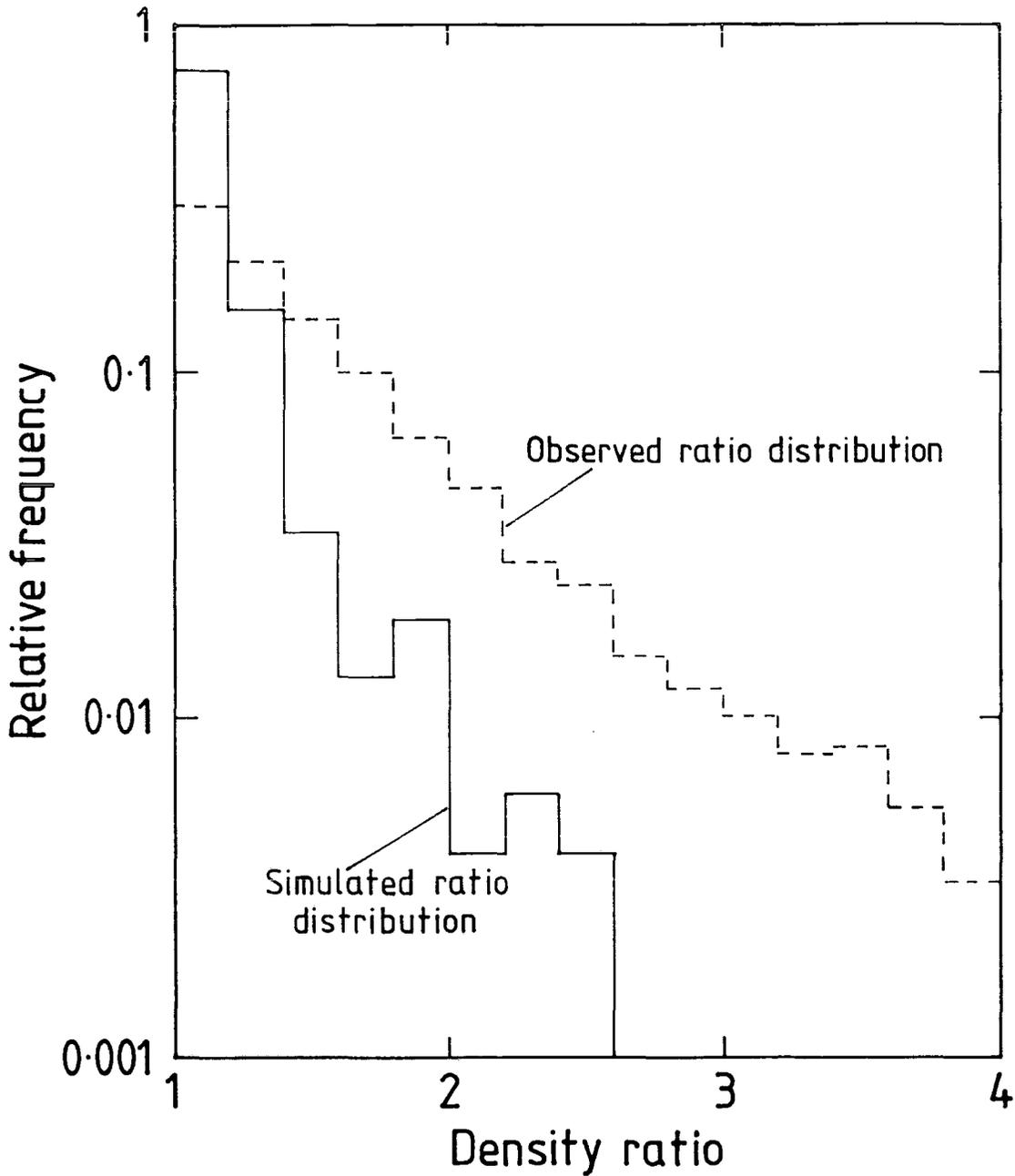
Figure 4.17: The frequency distribution of the ratio of the density of particles through one of scintillators to the other, for 1000 simulated showers by program 'MC.DENSITY01'. The experimental frequency distribution of the ratios is plotted for comparison. The number of experimental density ratios = 1816.
