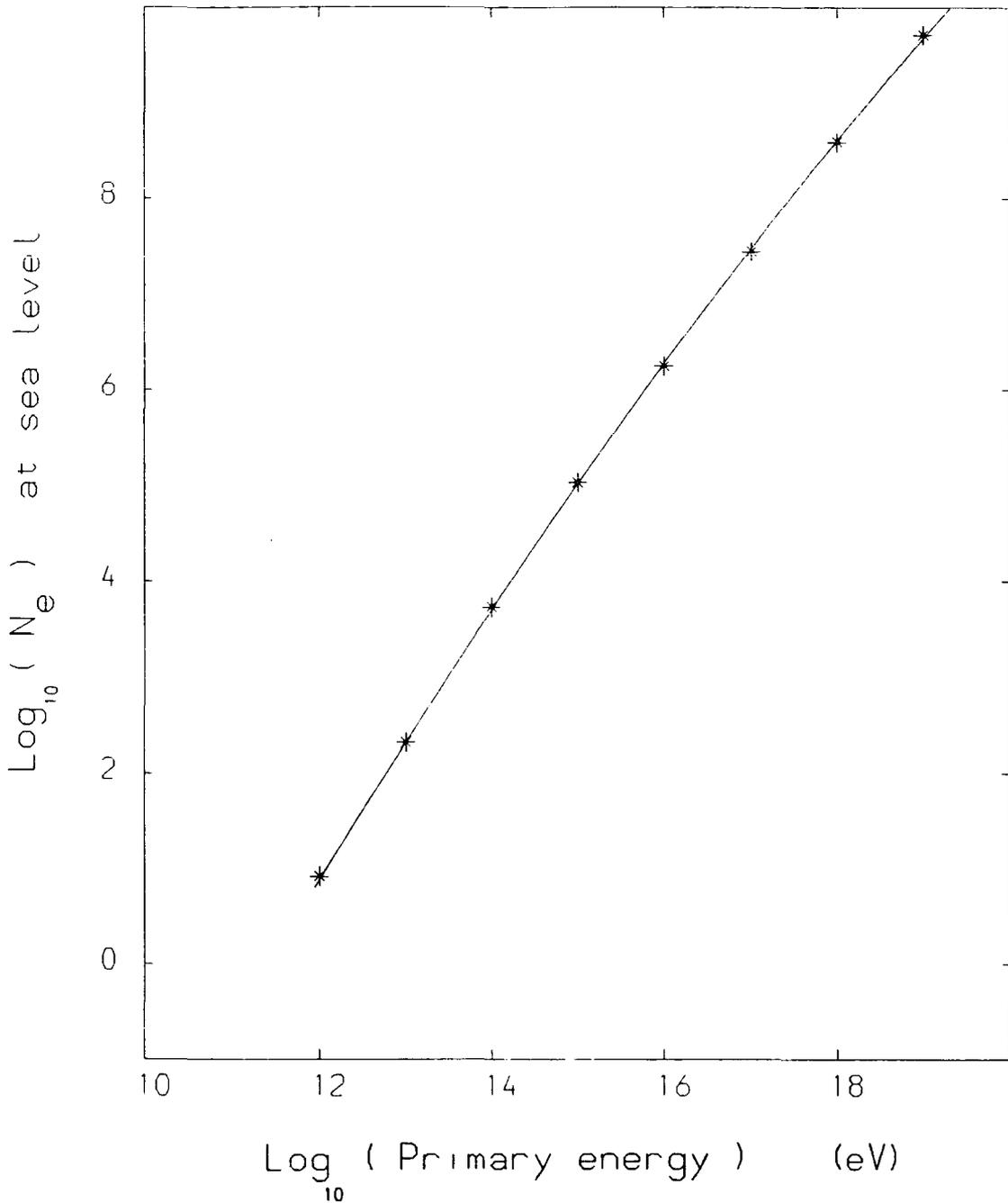
Figure 6.20: The best fit (solid curve) of the average simulated shower size at sea level as a function of the primary proton energy, simulated by the program MC007 (stars). The curve is described by:
