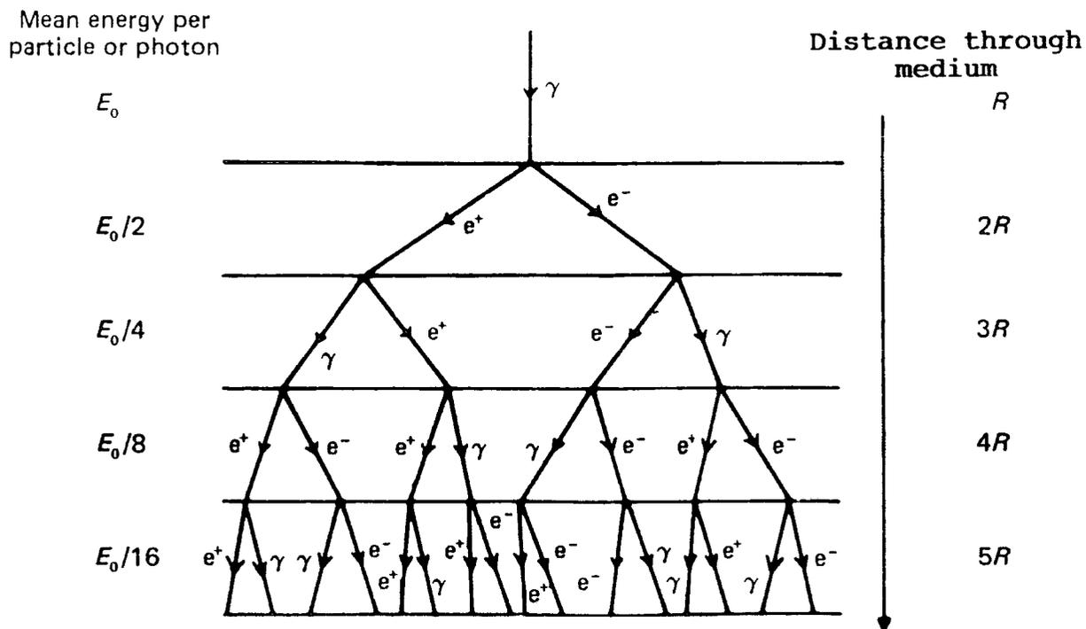
Figure 5.2 : A simple model of an electromagnetic shower.
