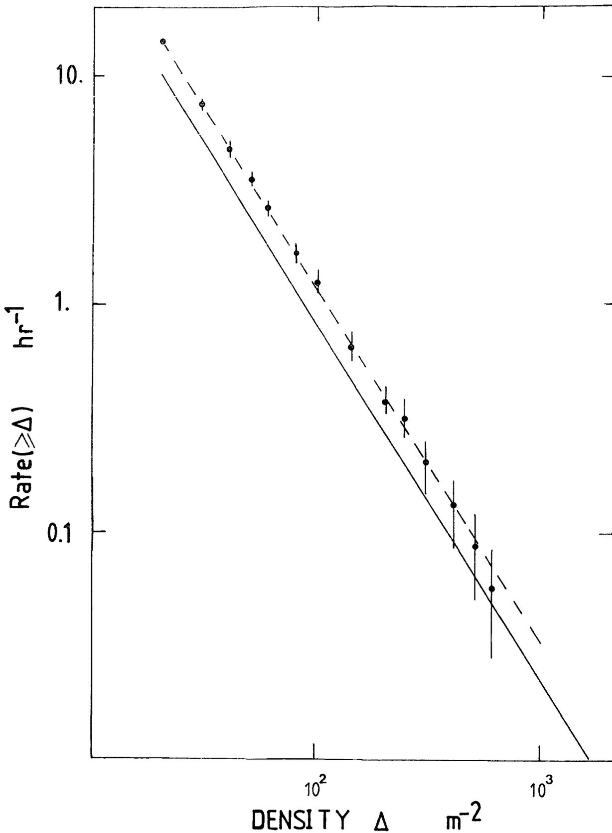
Figure 4.16: Simulated density spectrum by program 'MC.DENSITY01' produced for simulation of 1000 showers. The dashed line is the best fit line and the solid line represents the density spectrum obtained in this work.
