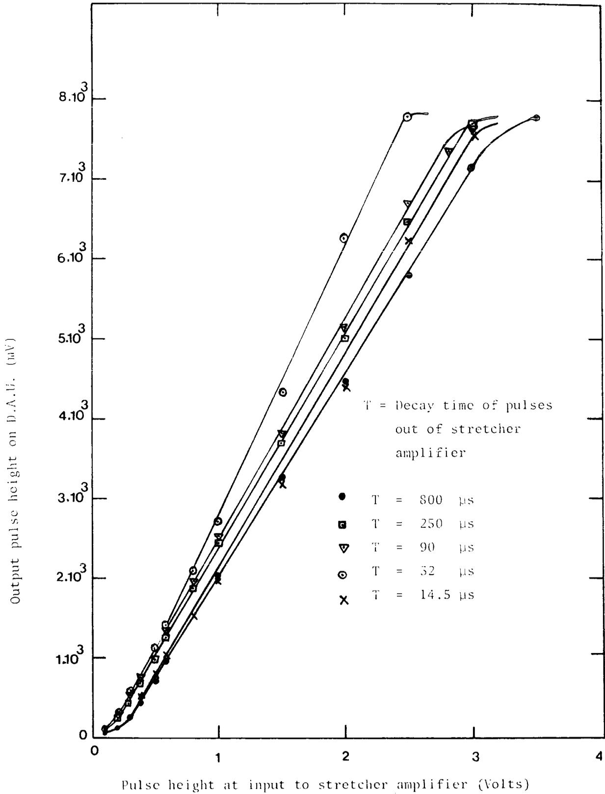
Figure 2.12: Calibration of the combination of stretcher amplifier and the data acquisition unit using 1  $\mu$ s width input square pulses.
