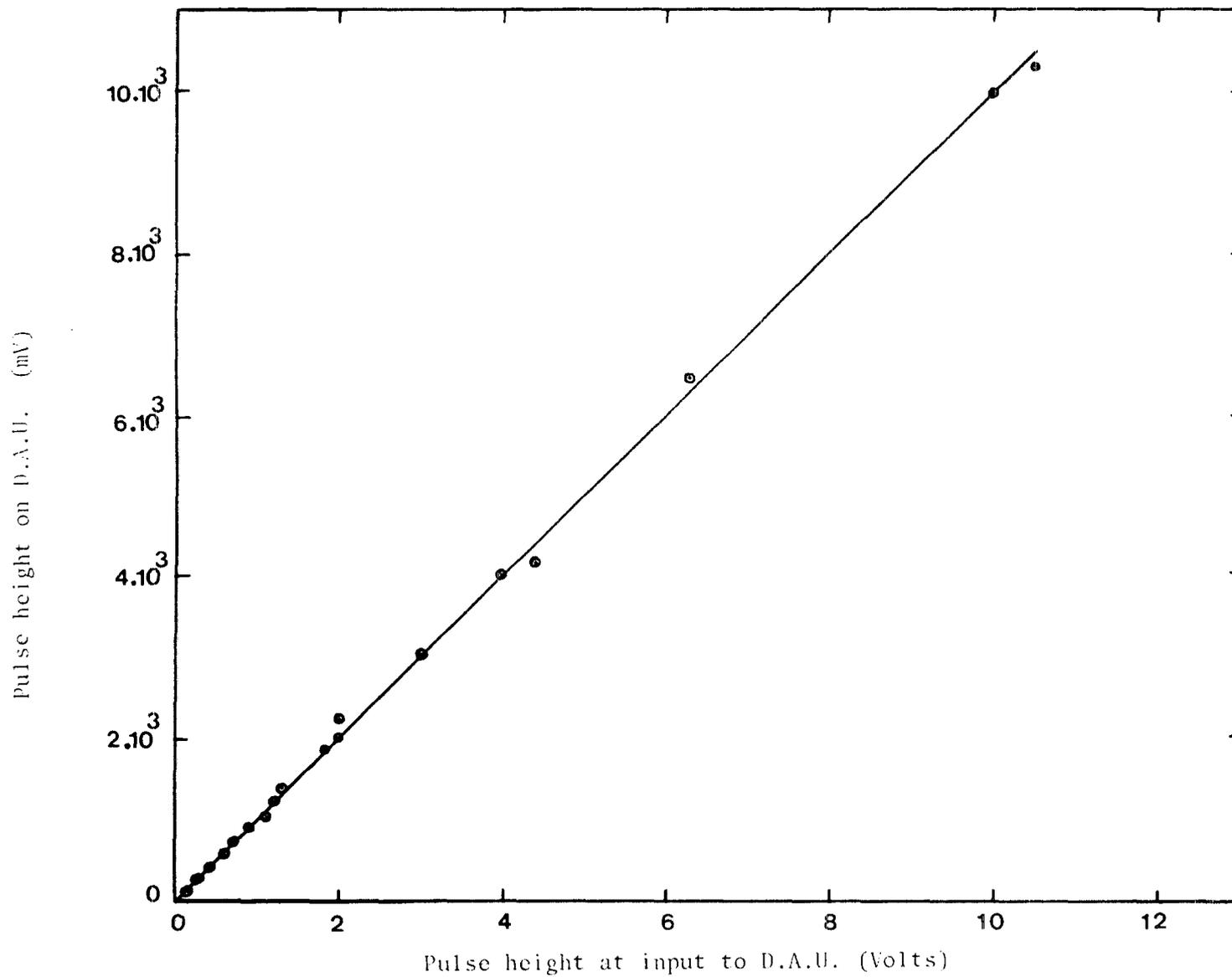
Figure 2.5 : Calibration of the data acquisition unit using 50  $\mu$ s width input square pulses. Similar results obtained for pulse widths down to 7  $\mu$ s (see figure 2.4 ).
