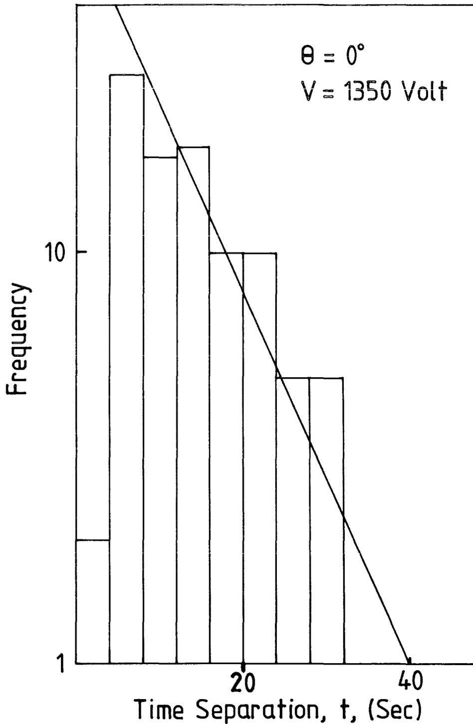
Figure 3.7: Differential distribution of time separation of 96 successive events for counters  $A_1$  and  $B_1$  in a running time 0.69 hours corresponding to a mean time separation  $T = 10$  seconds. The fitted straight line is of the form  $n(t) = n_0 e^{-t/T}$ .
