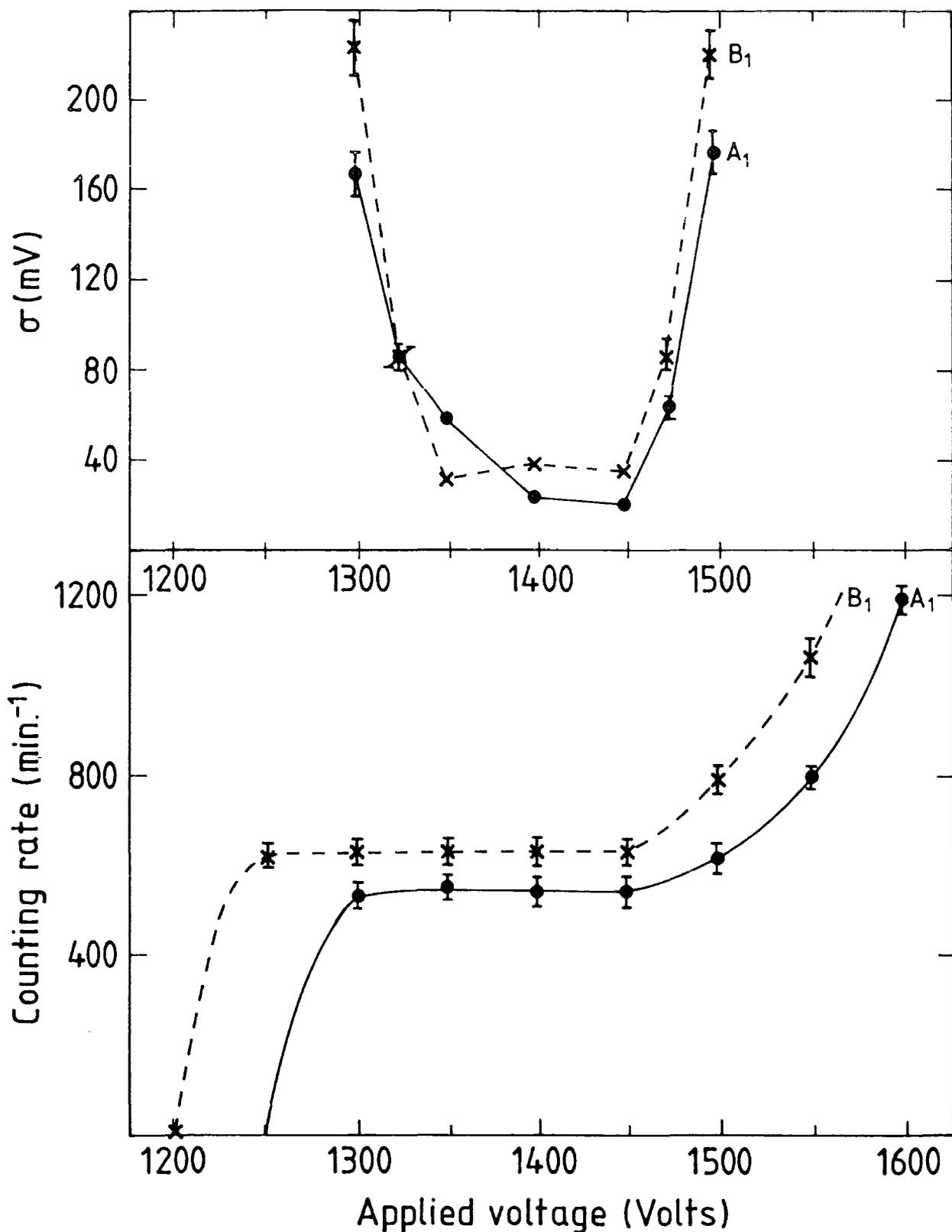
Figure 3.10: Comparison of the variation of the standard deviation ( $\sigma$ ) of the pulse height distribution about the mean value with counter operating voltage and the variation of the background counting rate with operating voltage for counters A<sub>1</sub> and B<sub>1</sub>.
