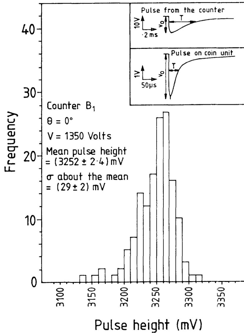
Figure 3.6: Pulse height distribution obtained by Geiger-Müller counters A<sub>1</sub> and B<sub>1</sub>.
