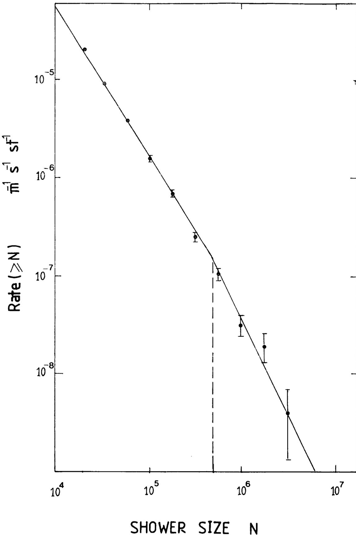
Figure 4.15: Simulated size spectrum by subroutine 'SIZE' produced by simulating 1000 showers. The line is the size spectrum given by Hillas (1970) which was used to generate the shower sizes.
