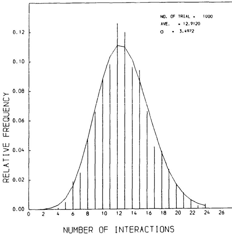
Figure 6.7: The graphical output of the program MC001, (bars). It shows the frequency distribution of the number of interactions which a cosmic ray proton with mean free path of  $80 \text{ g cm}^{-2}$ , undergoes before it reaches the sea-level. The simulation done for 1000 protons. The solid curve is the expected Poisson distribution.
