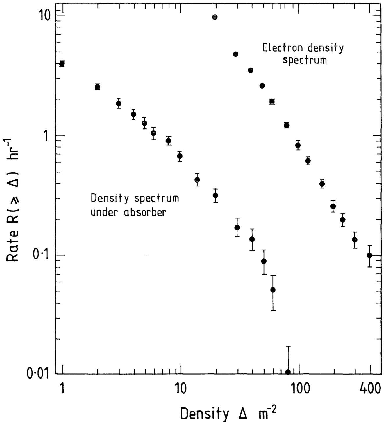
Figure 4.13: The integral density spectrum of the particles observed under the absorber, compared with the electron integral density spectrum.
