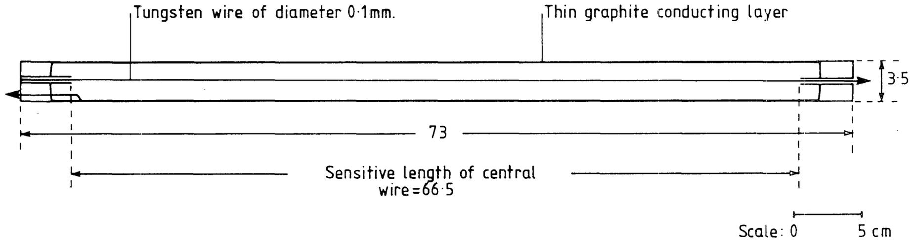
Figure 3.3: Diagram showing Geiger-Müller counter construction.
