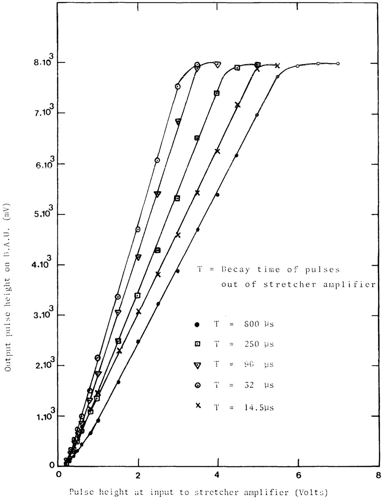
Figure 2.11: Calibration of the combination of stretcher amplifier and the data acquisition unit using  $1 \mu\text{s}$  decay time input exponential pulses.
