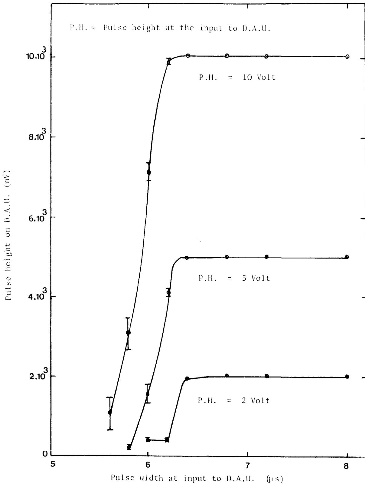
Figure 2.4 : Determination of threshold readable pulse height at the input to the data acquisition unit.
