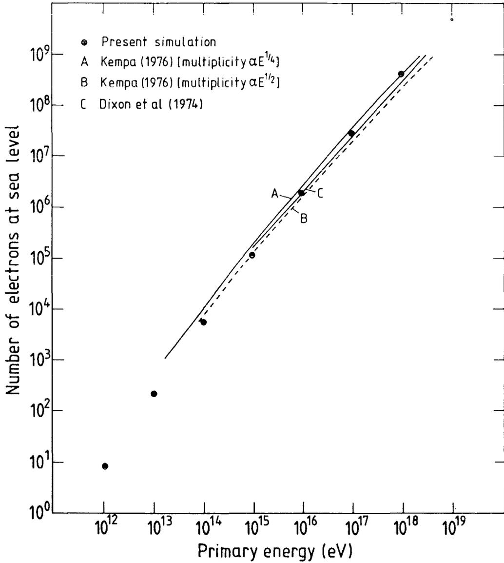
Figure 6.19: Average size of showers at sea level as a function of the primary proton energy, calculated by simulation. The present simulation (solid circles) is compared with some previous works.
