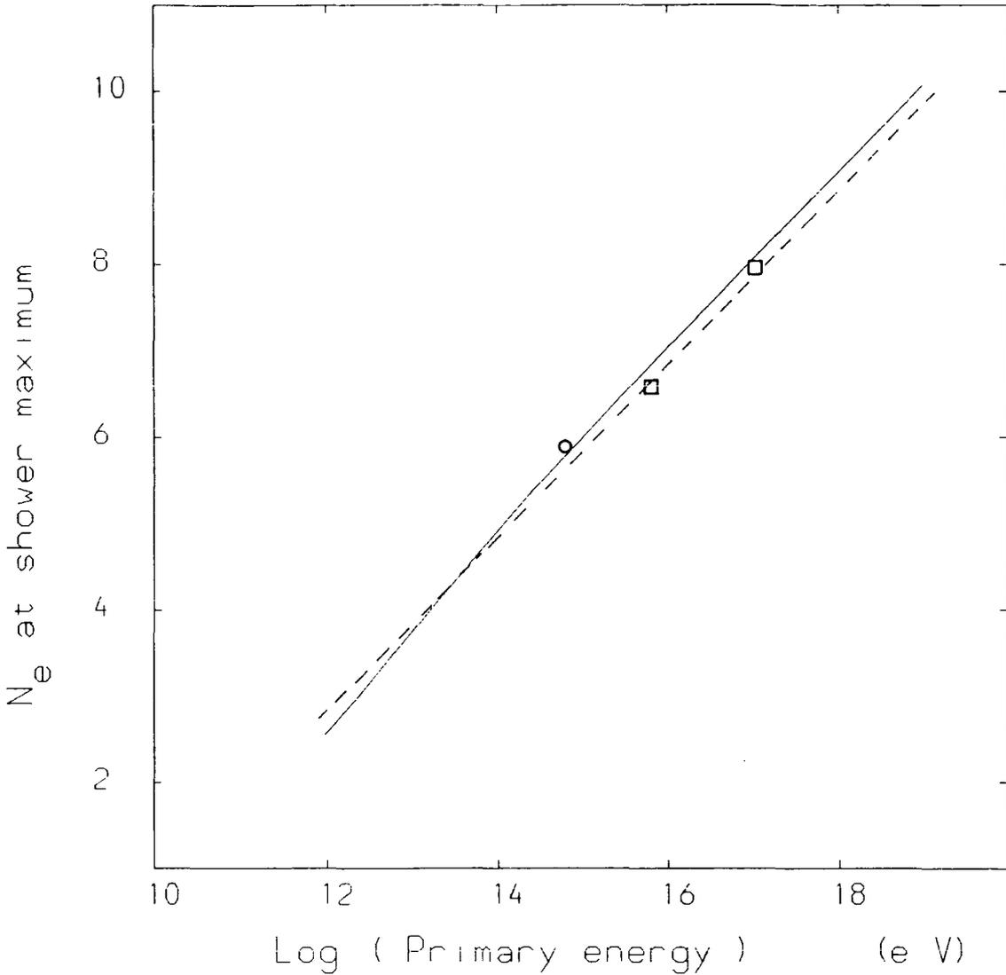
Figure 6.23: The shower size at the maximum of development curve represents the average behaviour of 1000 simulated showers (MC007), as a function of the primary energy. The dashed line is  $N_e = E_p / 1.4$  with  $E_p$  in GeV as La Pointe (1968) suggested. The circle is derived from Nikolski (1962) and the squares are from Hillas (1972).
