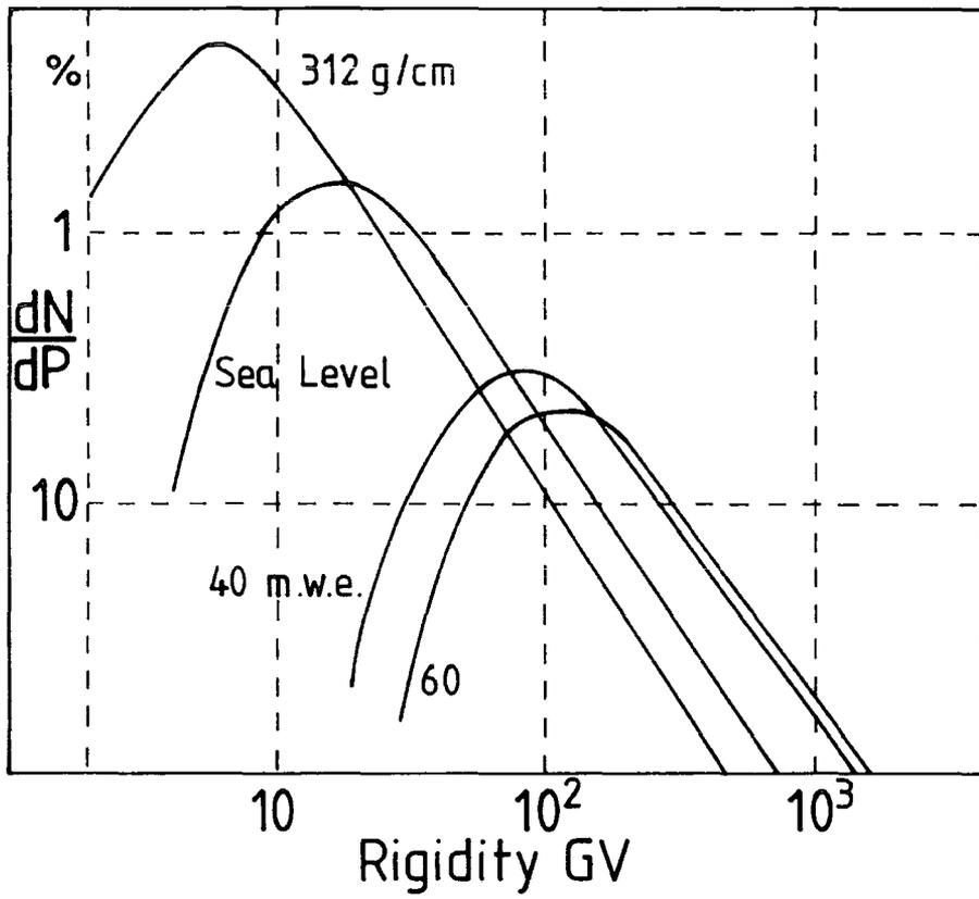
Figure 3.11: Differential response curves for meson monitors (after Webber and Quenby 1959).
