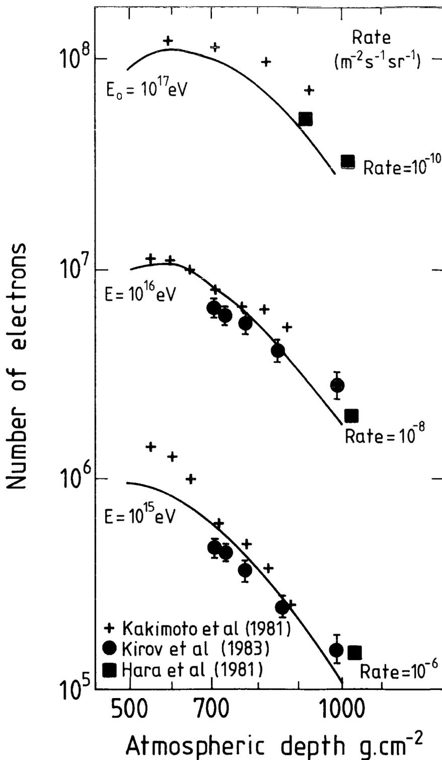
Figure 6.24: The shower size as it propagates through the atmosphere. The curves represent the simulation carried out by MC007 and the primary energy of each is written on each curve. The experimental data is plotted, but for given rate rather than primary energy.
