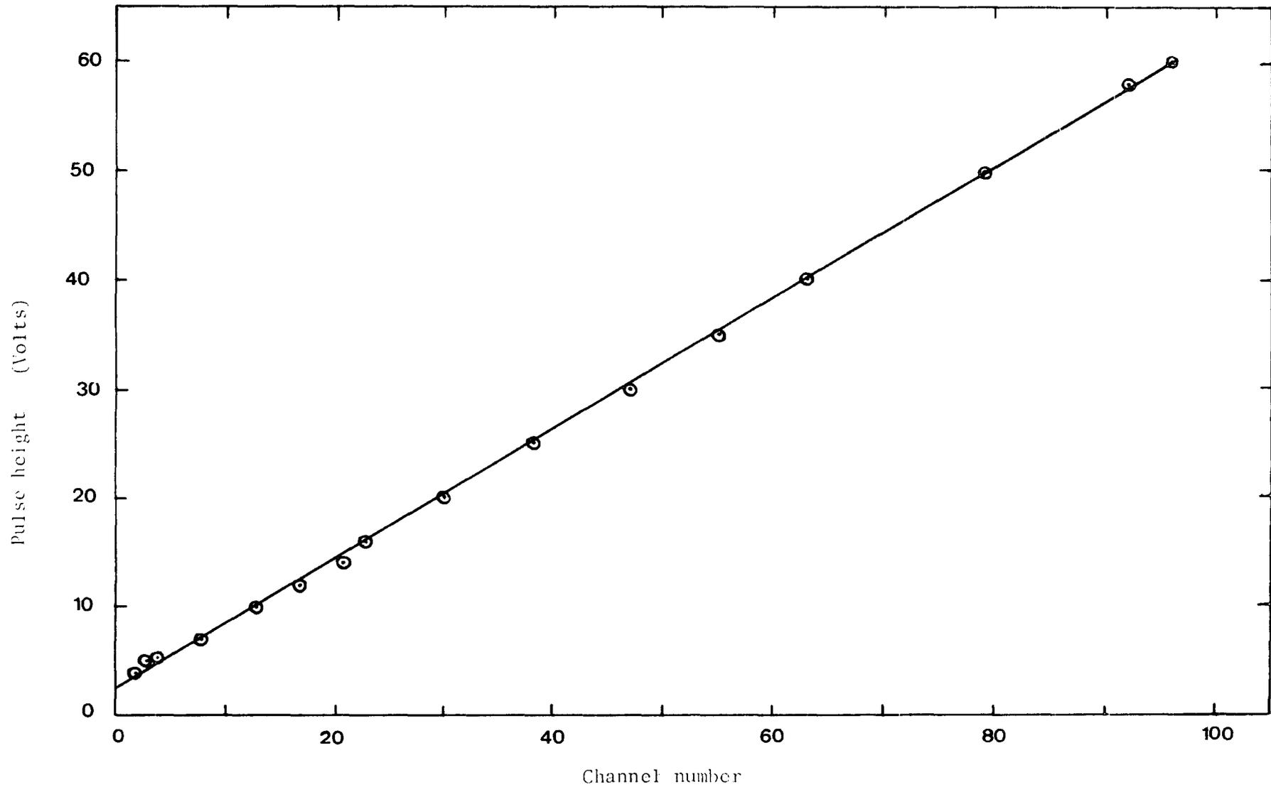
Figure 4.4: Calibration of the pulse height analyser using  $1 \mu\text{s}$  width input exponential pulses.
