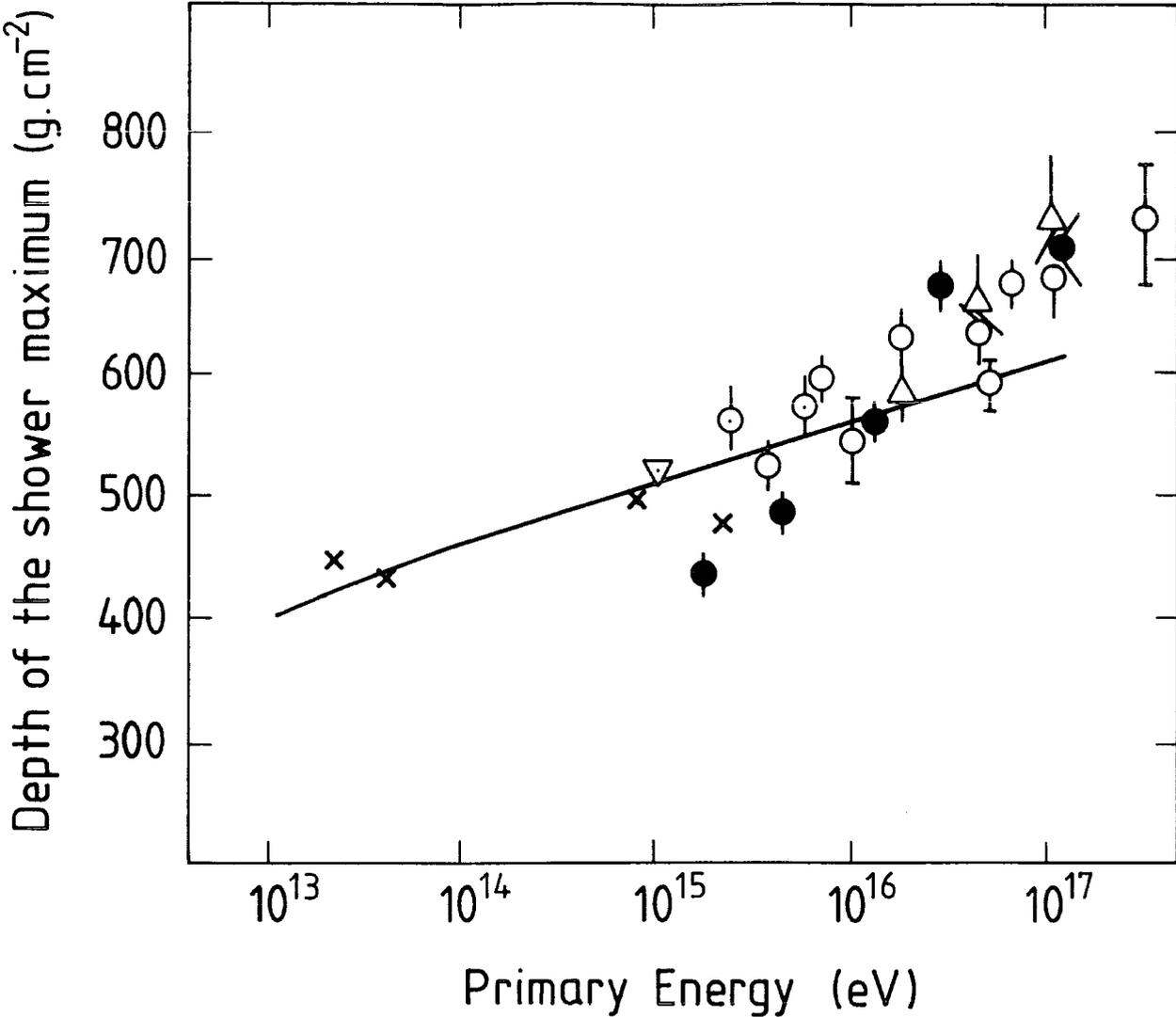
Figure 6.21: The depth of shower size maximum as a function of primary nucleon energy. It is the depth at which the average longitudinal development of electron number reaches its maximum. Some experimental data collected by Capdevielle and Gawin (1985) are compared with the result of the present simulation.
