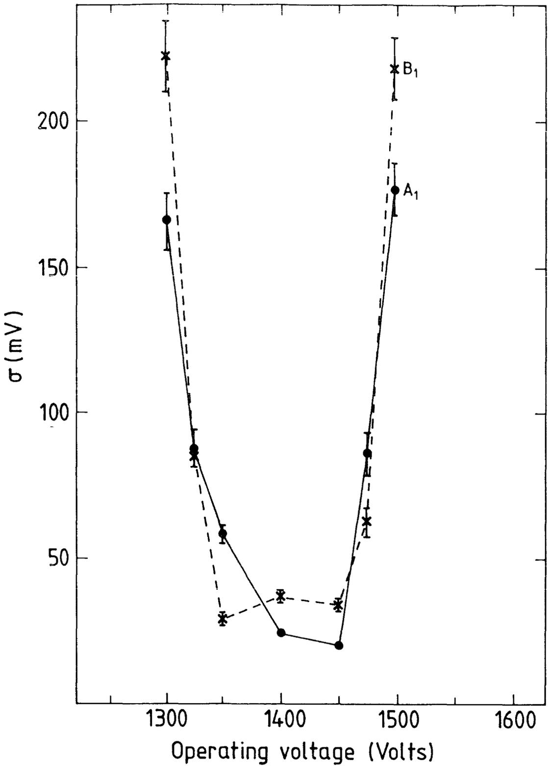
Figure 3.9: Dependence of the standard deviation ( $\sigma$ ) of the pulse height distribution about the mean value on the counter operating voltage for counters A<sub>1</sub> and B<sub>1</sub>
