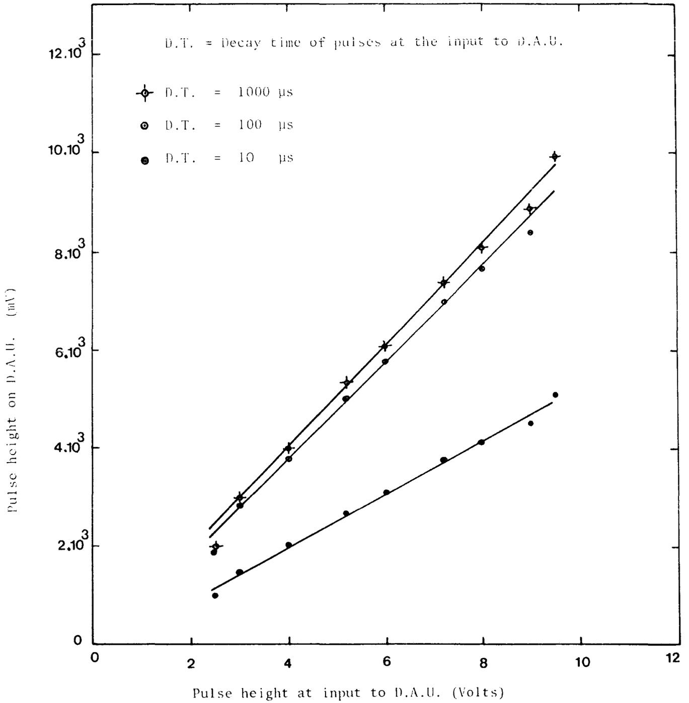
Figure 2.5 : Calibration of the data acquisition unit using negative exponential pulses.
