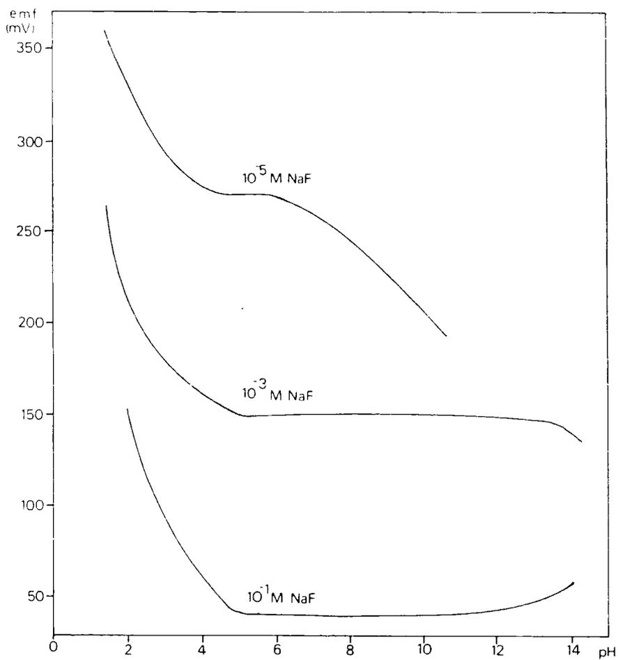
Fig. 4.6 Effect of pH on Measured EMF for the Activation Fluoride Ion Electrode
