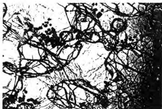
Figure 3b. Chrome-spinel concentrations on the upper surfaces of olivine crystals from unit 2 peridotite. Scale bar = 0.5 mm.
