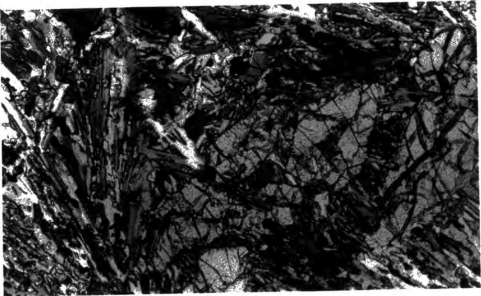
Fig 2.6 Skeletal olivines in variolitic-textured gabbro. Loc 53A. NM38609549.
