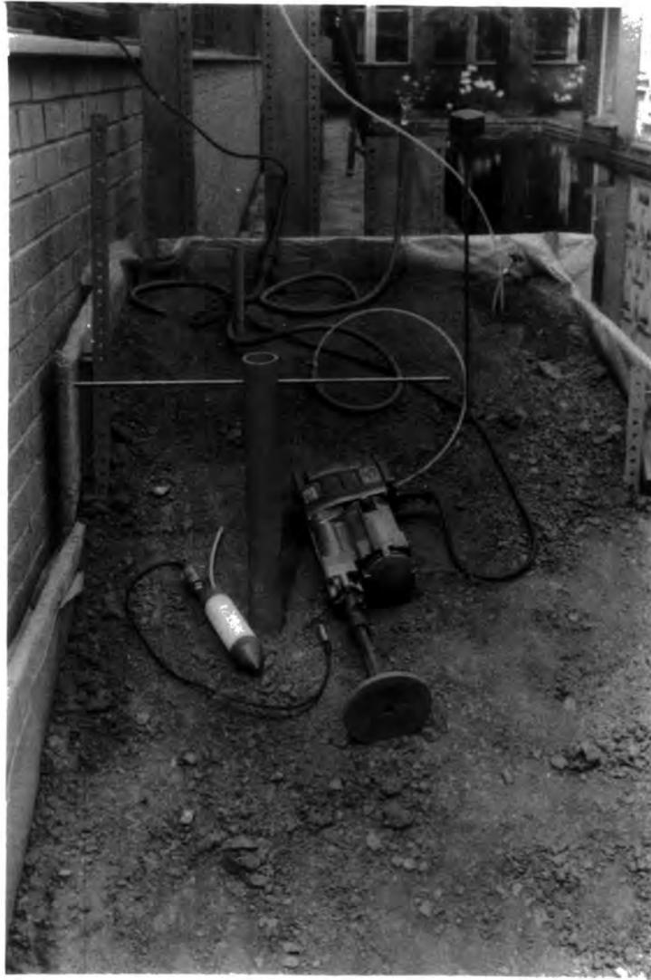
**Figure 6.7** Construction of Maltby experimental tip showing tensiometer ready for installing in hole made by cutter tube.
