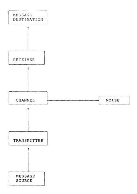
Figure 1.1 An engineer's model of the communication process (From C.E. Shannon and W. Weaver, The Mathematical Theory of Communication, University of Illinois Press, 1949)
