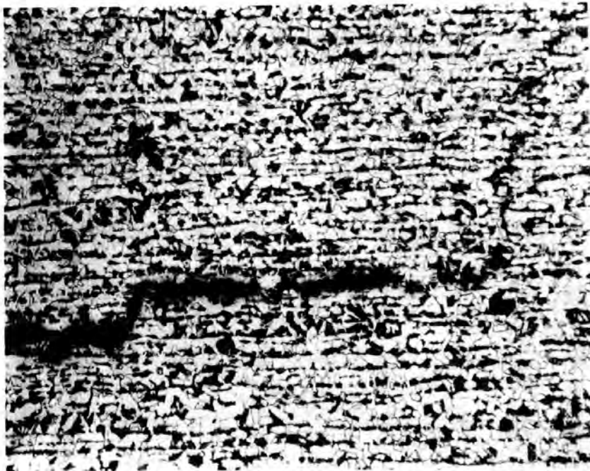
Figure 107 Metallographic section of pipe section 3 showing the extent of the banding x 100
