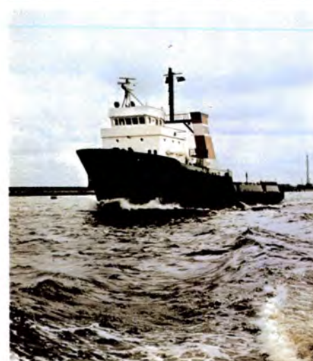
Oil Hustler is one of O.I.L.'s latest supply vessels, developing 8000 bhp. Among other contracts, this vessel has provided support services for underwater inspection of production platforms in the UK sector of the North Sea. O.I.L.'s supply ships are fully equipped for anchor handling and towing in addition to their supply duties for drilling rigs and production platforms.
