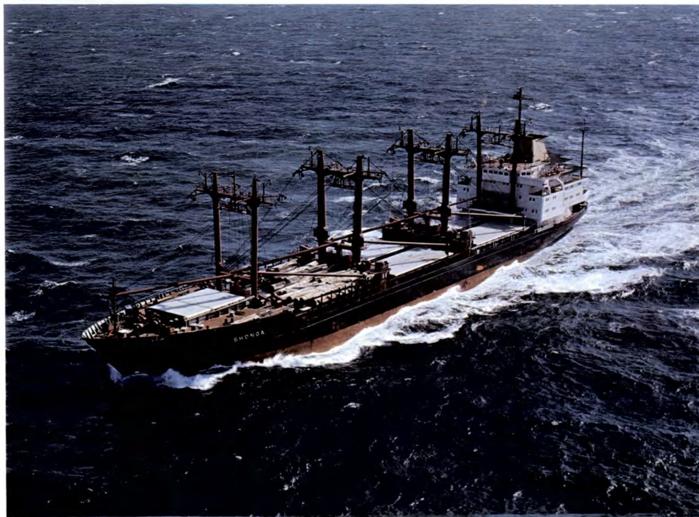
Shonga is one of Elder Dempster's two multi-purpose/semi-container freighters which entered service in 1974. Both vessels operate on UKWAL's Express Service from London to Apapa, Nigeria. They can load 396 containers and, when utilised to their best advantage with a mixture of general cargo, 290 containers.
