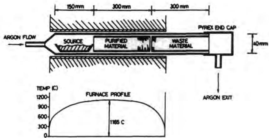
Figure 3.6 Purification of ZnSe by argon flow sublimation.
