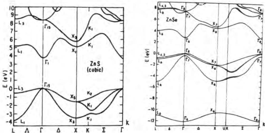
Figure 2.3 Band structure of ZnS and ZnSe (ref. 1,2).
