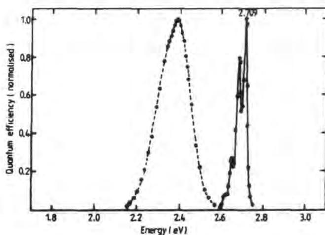
Figure 3.10 Photoluminescence emission at 80 K from samples of ZnSe after heating in Zn/Ga at 600 °C (broken curve) and 850 °C (full curve) (ref. 22)).
