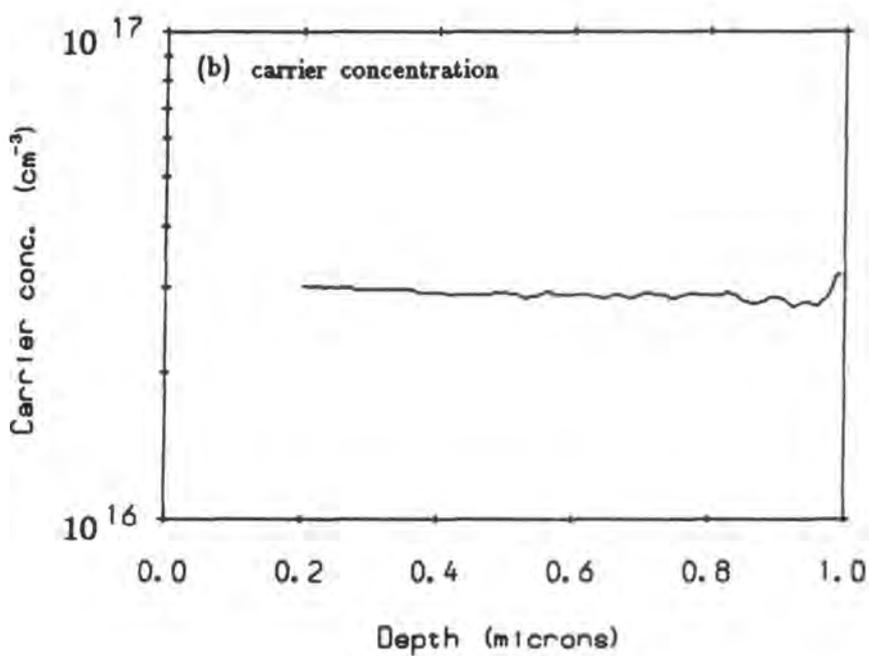
Figure 4.9 (a)  $\frac{1}{C^2}$  vs  $V$  and (b) the corresponding carrier concentration profile of an MOCVD grown layer of ZnSe.
