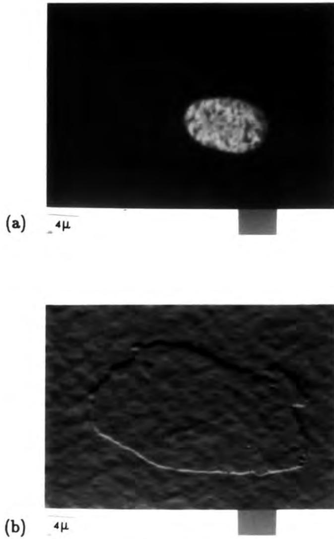
Figure 5.13 (a) EBIC image and (b) secondary electron micrograph of an ZnSe MIS device with a polycrystalline ZnS I-layer.
