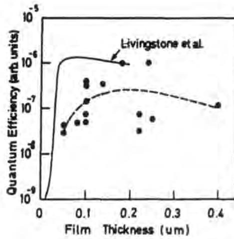
Figure 3.1 Quantum efficiency of ZnSe MIS diodes as a function of I-layer thickness (ref. [8]).
