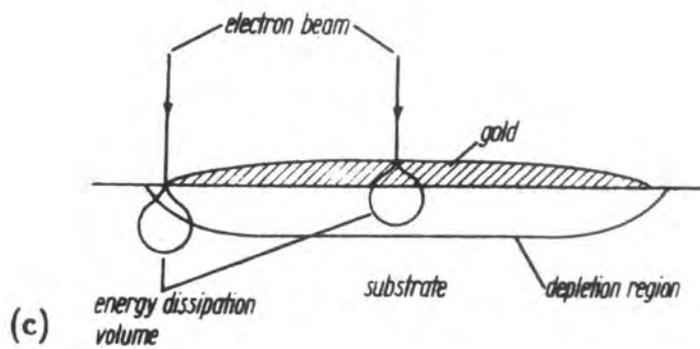
Figure 5.12 (a) EBIC image and (b) secondary electron micrograph of a gold Schottky contact on epitaxial MOCVD ZnSe, (c) model to explain the EBIC contrast of MS diodes (ref. [15]).
