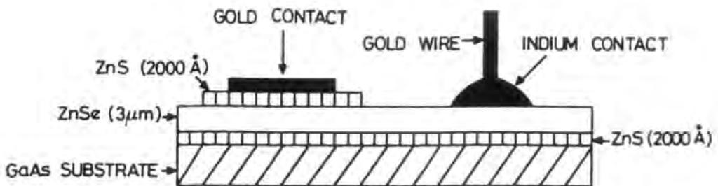
Figure 5.6 ZnSe MIS device with evaporated polycrystalline ZnS I-layer.
