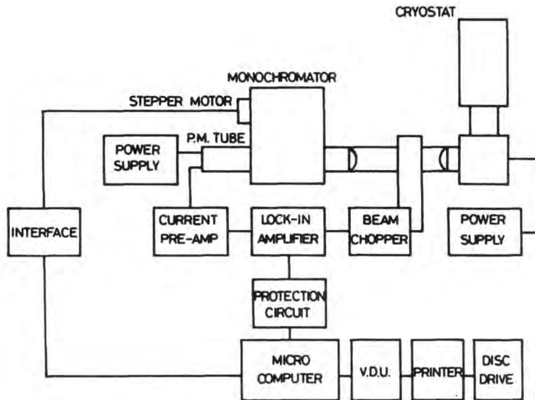
Figure 3.8 Schematic diagram of the automated electroluminescence system.
