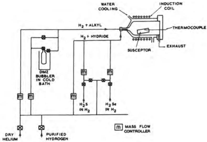
Figure 4.1 Horizontal reactor MOCVD growth system (ref. [9]).
