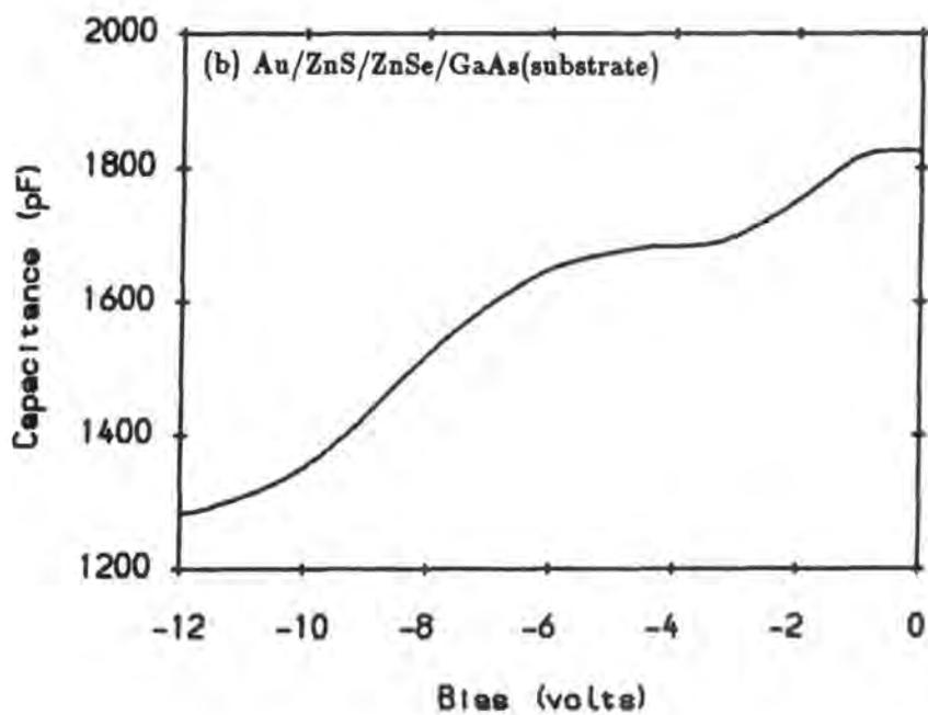
Figure 5.11 Capacitance–voltage characteristics of epitaxial MIS devices: (a) Au/ZnS/ZnSe, (b) Au/ZnS/ZnSe/GaAs(substrate).
