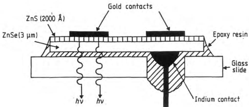
Figure 5.2 ZnSe MIS device with epitaxial ZnS I-layer.
