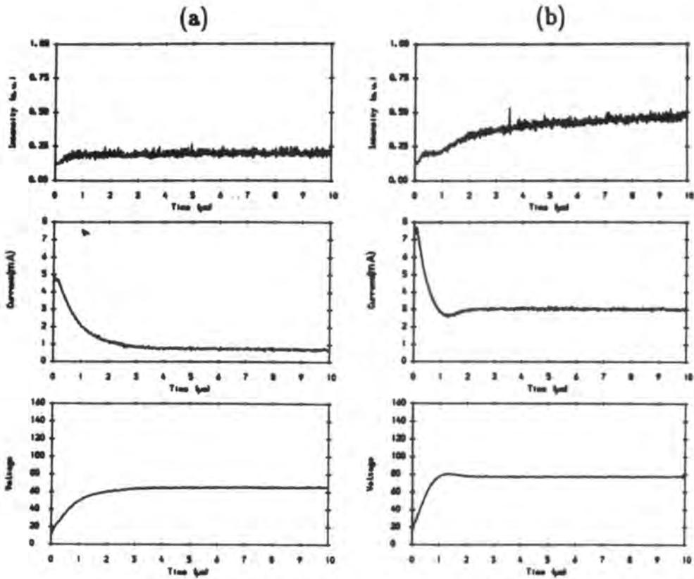
Figure 6.18 Luminescence, current and voltage transients, recorded from an epitaxial DCTFEL device with a ZnS:Mn layer  $\sim 0.3 \mu\text{m}$  thick, showing an initial instantaneous EL emission at voltages (a) below, and (b) above, the voltage threshold for the main EL transient.
