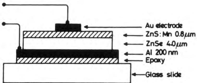
Figure 6.2 Epitaxial thin film ZnS:Mn DCEL device geometry.
