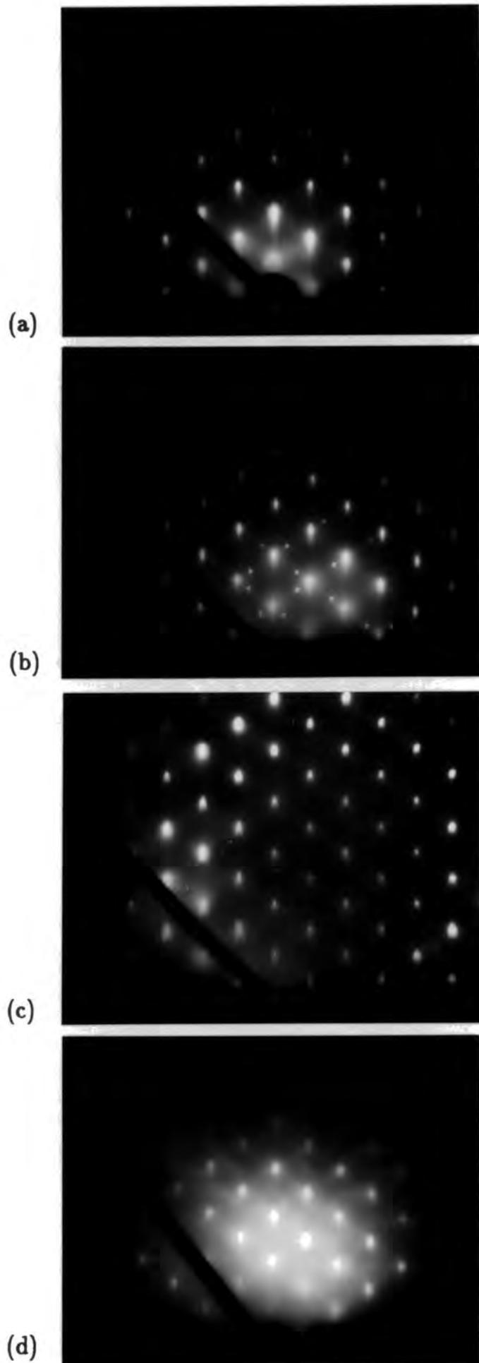
Figure 4.7 100 kV  $\langle 110 \rangle$  zone axis RHEED patterns recorded from the as-grown surface of: (a) GaAs/ZnSe, (b) GaAs/ZnS/ZnSe (beam along  $[110]$ ), (c) GaAs/ZnS/ZnSe (beam along  $[\bar{1}10]$ ), and (d) GaAs/GaAlAs/GaAs/ZnS/ZnSe structures.
