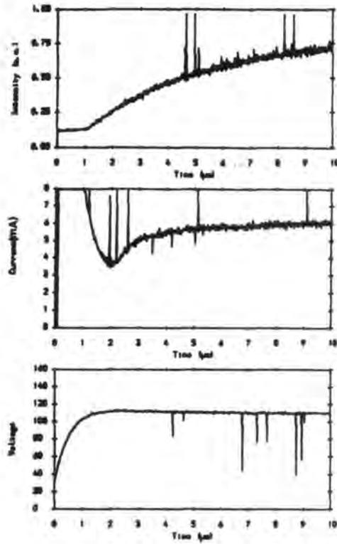
Figure 6.13 Luminescence, current and voltage transients recorded from an epitaxial DCT-FEL device under constant voltage operation with 120 V pulses.
