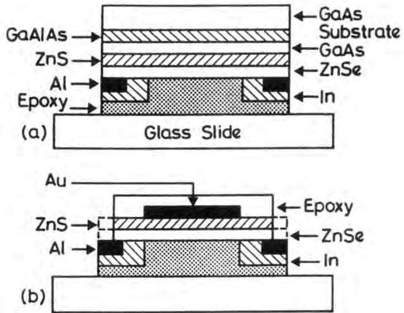
Figure 5.5 Fabrication sequence for an epitaxial ZnS/ZnSe device using III-V compound buffer layers (a) as-grown structure, (b) final device geometry (dotted region indicates structure prior to final etch to expose ohmic contacts).
