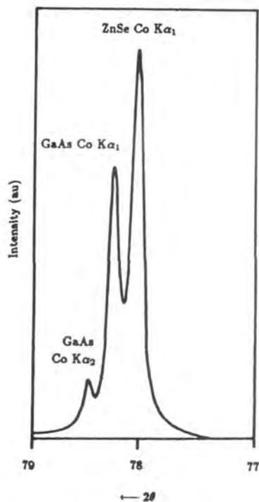
Figure 4.4 X-ray diffraction peaks for the (400) reflection from a ZnS/ZnSe epitaxial structure on (100) orientated GaAs.
