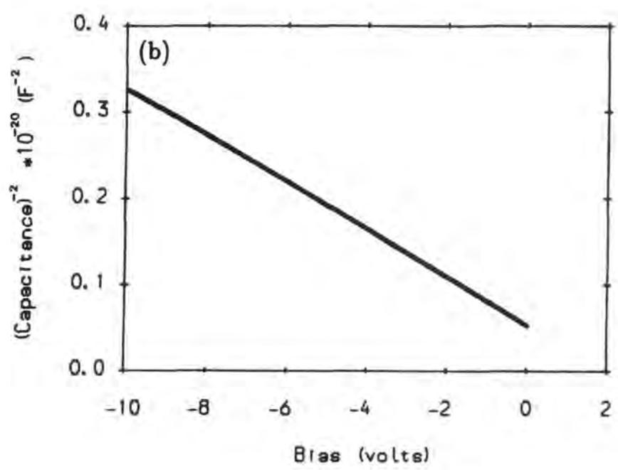
Figure 3.14 Typical plots of (a) capacitance ( $C$ ) vs voltage ( $V$ ), and (b)  $\frac{1}{C^2}$  vs  $V$  for an Au/ZnSe diode.
