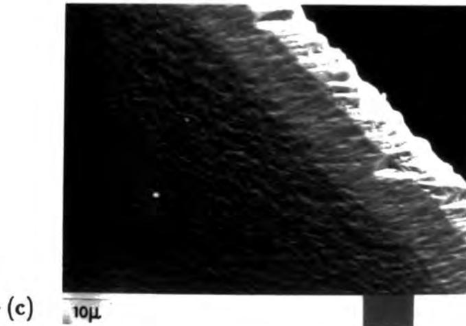
Figure 4.6 Growth features at the substrate edge: (a) ZnSe ( $8.0\ \mu\text{m}$ ) grown with a "high" DMZ flow rate, (b) X-ray map for zinc taken from the same area, (c) ZnSe ( $3.0\ \mu\text{m}$ ) grown at the "normal" DMZ flow rate.
