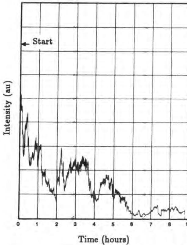
Figure 6.19 Typical intensity-time plot for an epitaxial DCTFEL device, with a ZnS:Mn layer  $\sim 0.8 \mu\text{m}$  thick, during operation with  $10 \mu\text{s}$  pulses of 100 V with a 1% duty cycle.
