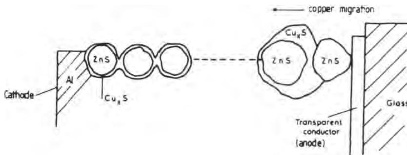
Figure 2.25 Structure of a formed DCEL powder panel (ref. 78).
