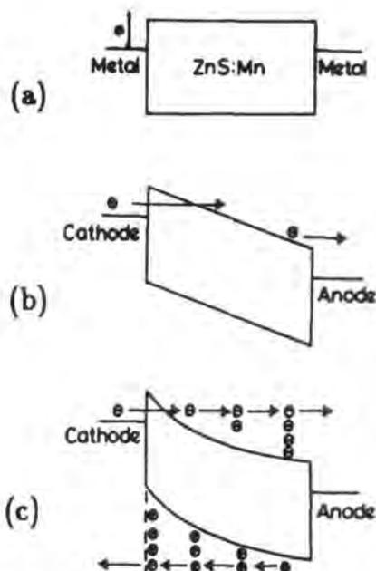
Figure 6.4 The idealised energy band diagram of a DCEL device: (a) at zero bias, (b) with moderate bias, (c) with a localised region of high electric field at the cathode.
