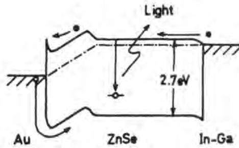
Figure 3.2 Minority carrier injection in the forward biased Au/ZnSe/ZnSe MIS junction (ref. [8]).
