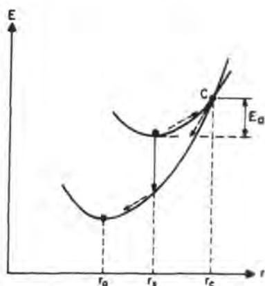
Figure 2.16 Configuration diagram showing radiative transition (solid arrow) and non-radiative transition via point c (ref. 34).
