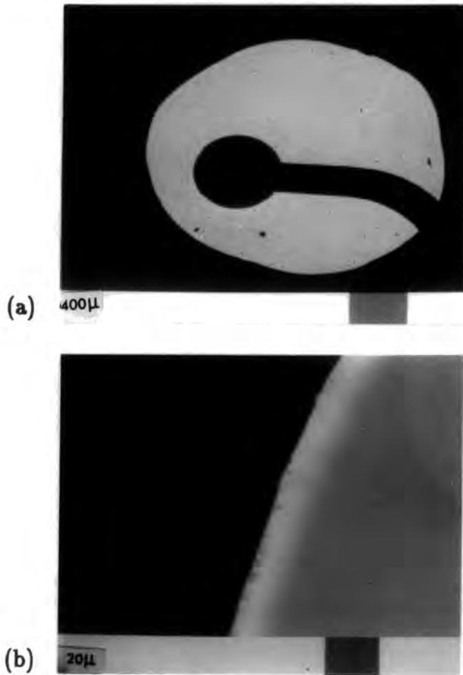
Figure 5.14 EBIC images of a ZnSe MIS device with an epitaxial ZnS I-layer at (a) low and (b) high magnification.
