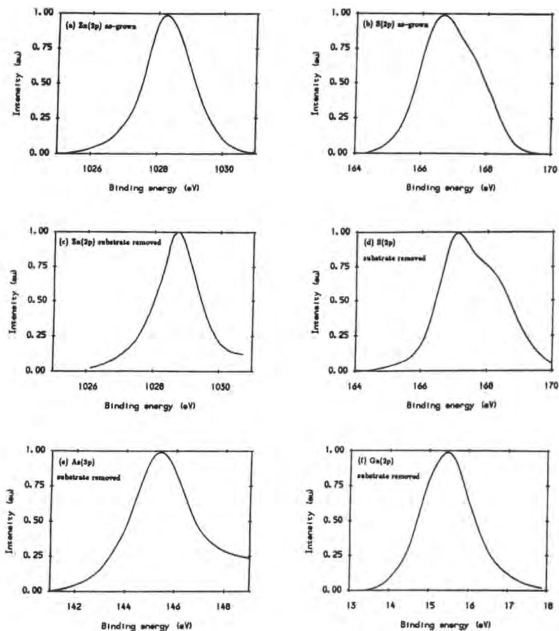
Figure 5.9 ESCA profiles from a MOCVD ZnS I-layer: (a) zinc and (b) sulphur on the as-grown MOCVD ZnS surface; (c) zinc, (d) sulphur, (e) arsenic and (f) gallium on the surface revealed by removal of the GaAs substrate.
