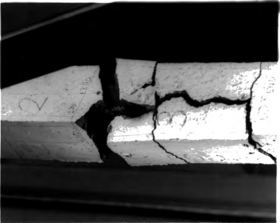
Fig. 6.7.1 Failed specimens Specimen 250T12/12
