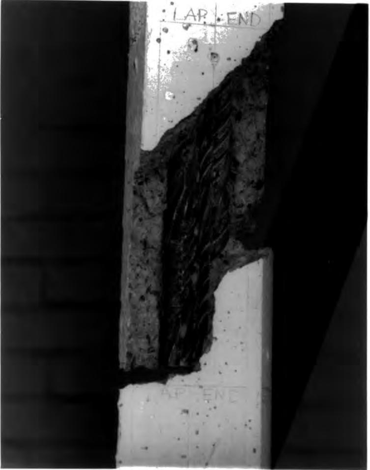
Fig. 6.7.2 Failed specimens Specimen 250T20/20
