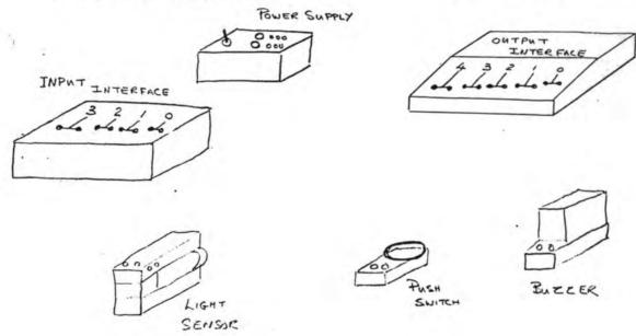
3.) You have been asked to design a computer controlled doorbell. The doorbell will only work during the day. If the switch is pressed at night the bell will not ring.
