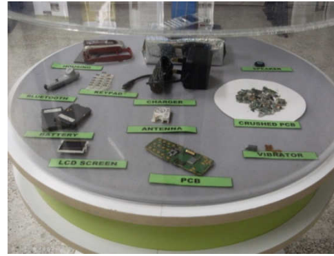
Plate 2.2: Dismantled components of a mobile phone. (Source: author - courtesy of Tes-Amm (M) Sdn. Bhd.)
