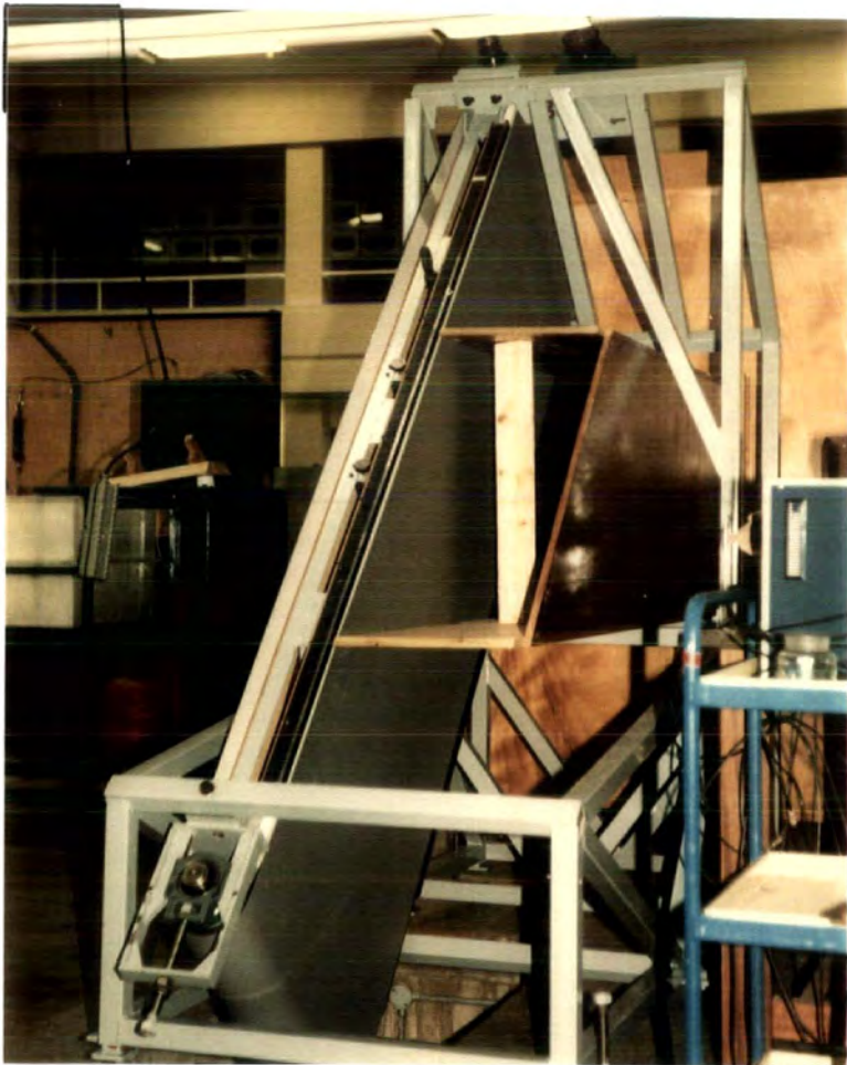
FIGURE 3.8: Moving Belt Mounted Into Tunnel
