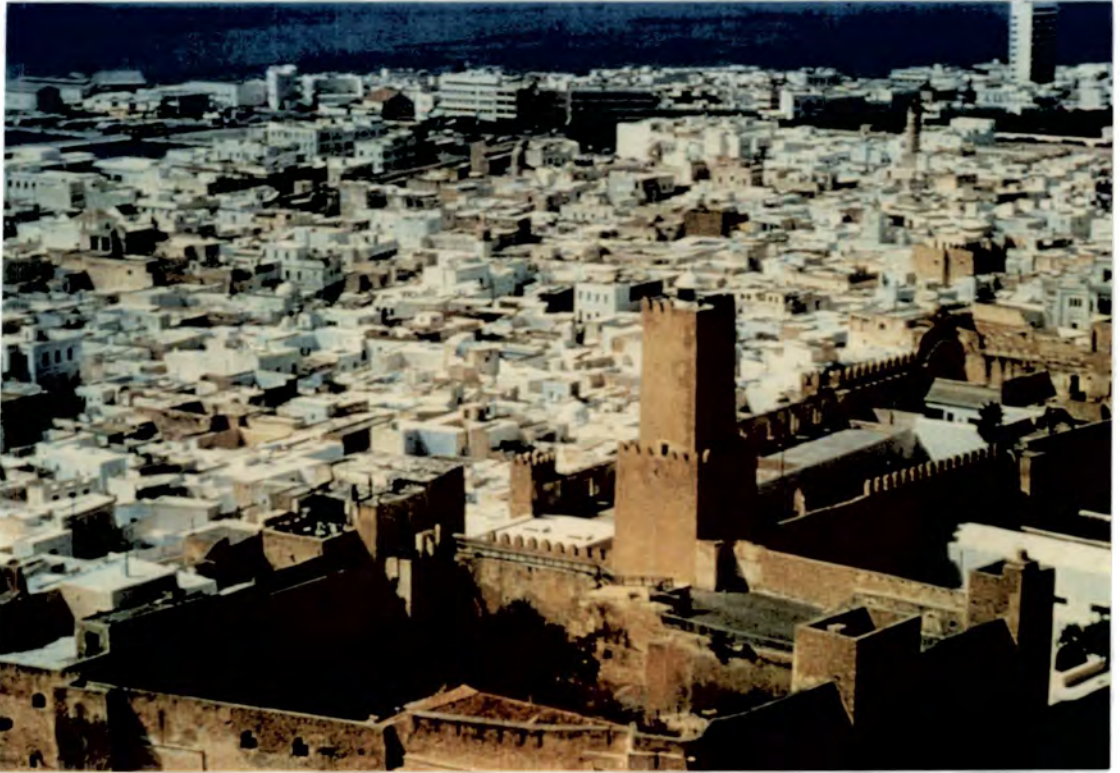
Plate 5.1 The large coastal settlement of Sousse. The narrow streets and square buildings of the old town produce high levels of Seasat backscatter due to the action of corner reflectors.
