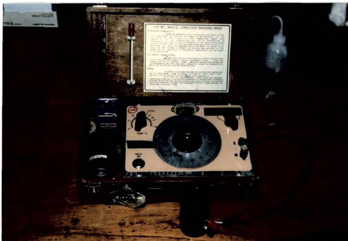
Plate 6.11 Conductivity meter used for the measurement of specific conductivity of samples collected in the field.
