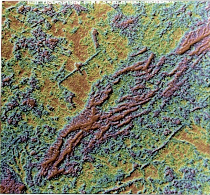
Plate 5.54 HSI transform of filtered SIR-A image of Djebel Henndi. Hue is determined by the low-pass filter, saturation by the high pass filter and intensity by the directional filter. The image is particularly useful for the identification of linear features and relief form.
