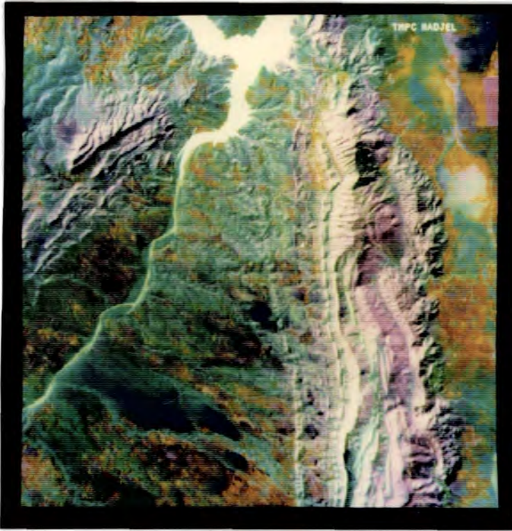
Plate 5.31 Image derived from TM Principal Components 1, 2 and 3 for the Hadjel Valley and Djebel Nara. Variations in soil and vegetation are depicted by variations in green, blue and orange hue. The upland areas are characterized by white and purple hues in accordance with lithology and shadowing.
