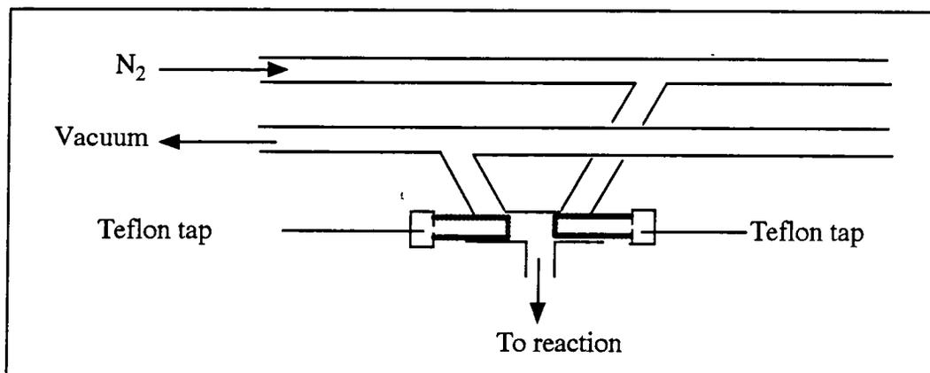
The nitrogen supply was dried by passage through concentrated sulphuric acid, phosphorous pentoxide, and activated 13X and 4A molecular sieves. An Edwards P2 pump was used to provide the vacuum ( $10^{-3}$  torr).
