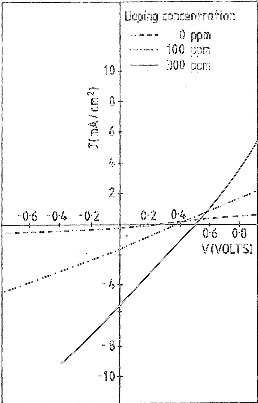
Fig. 8.5 : Photovoltaic behaviour of Hetrojunction with different Cu concentrations.
