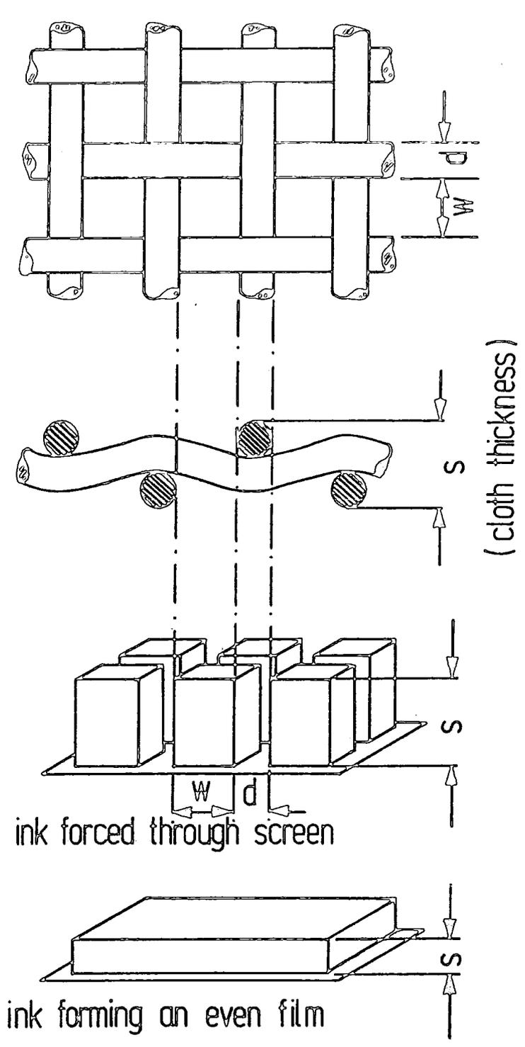
Fig. 4.4 Significance of screen parameters on print quality
