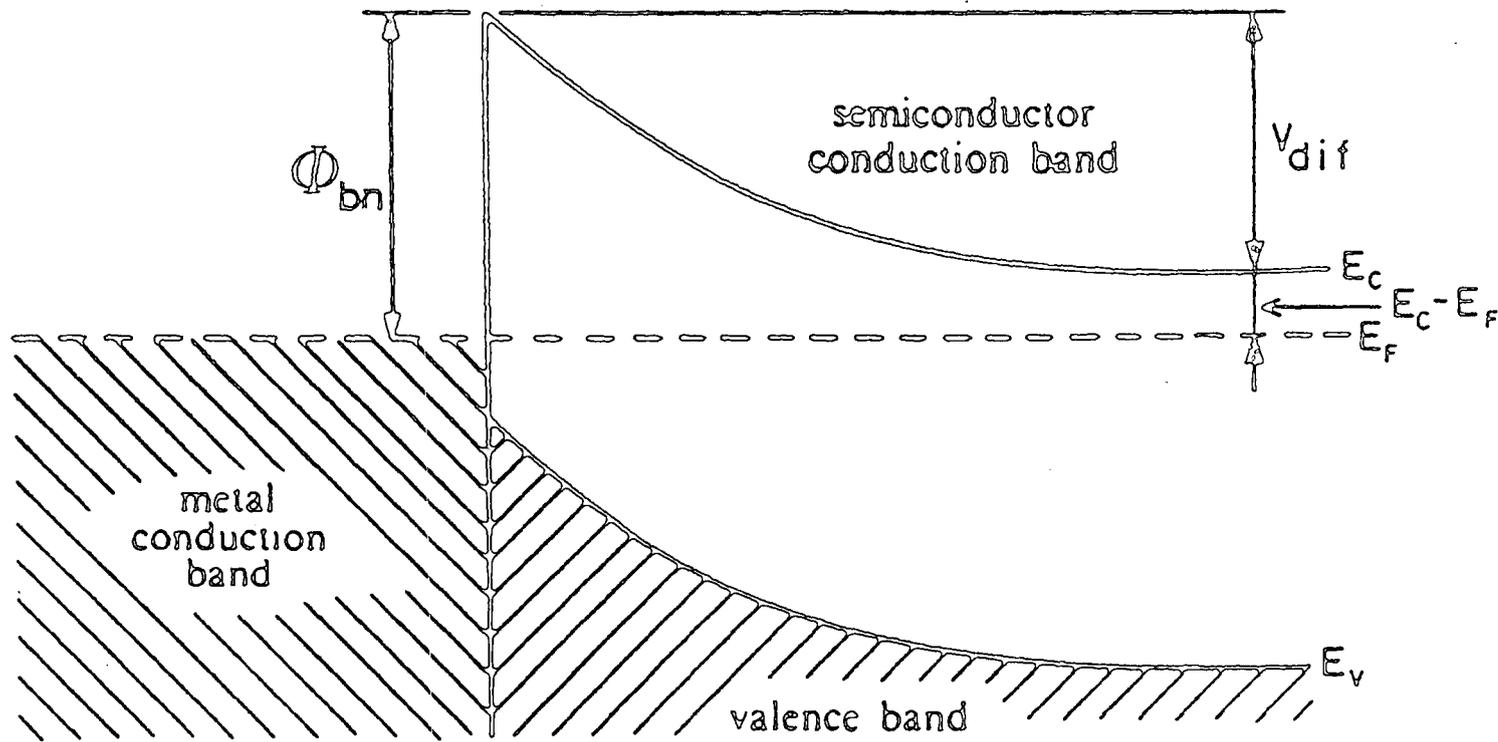
Fig. 2.2 : Energy band diagram of an ideal metal n-type semiconductor contact (Schottky barrier).
