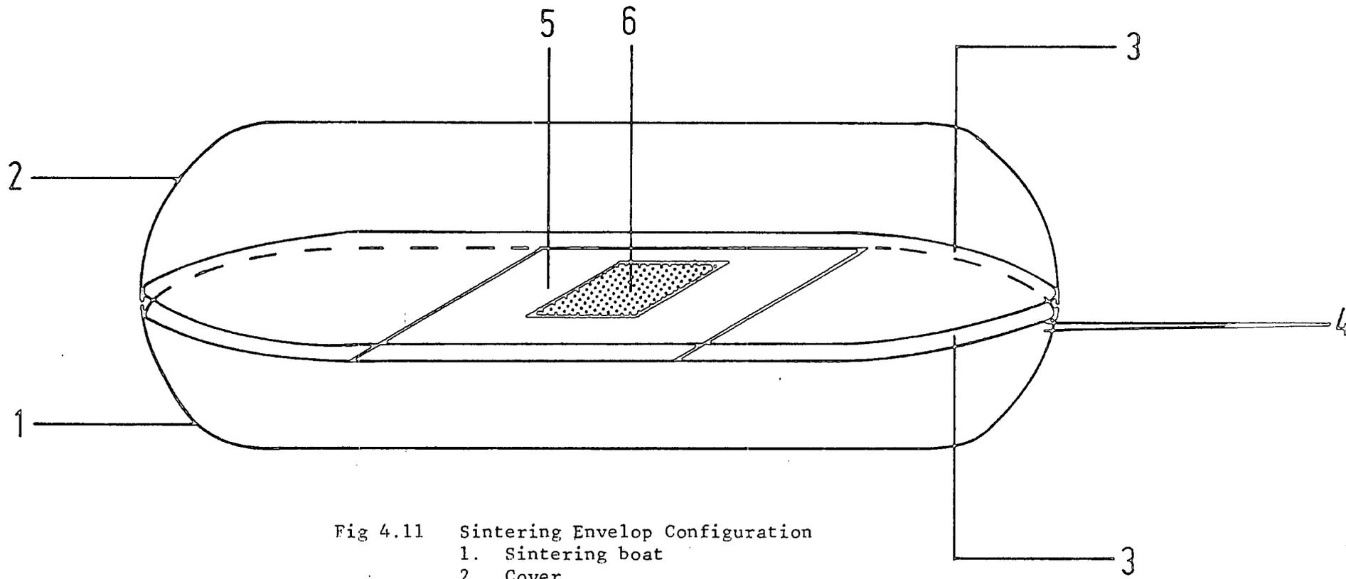
Fig 4.11 Sintering Envelop Configuration
