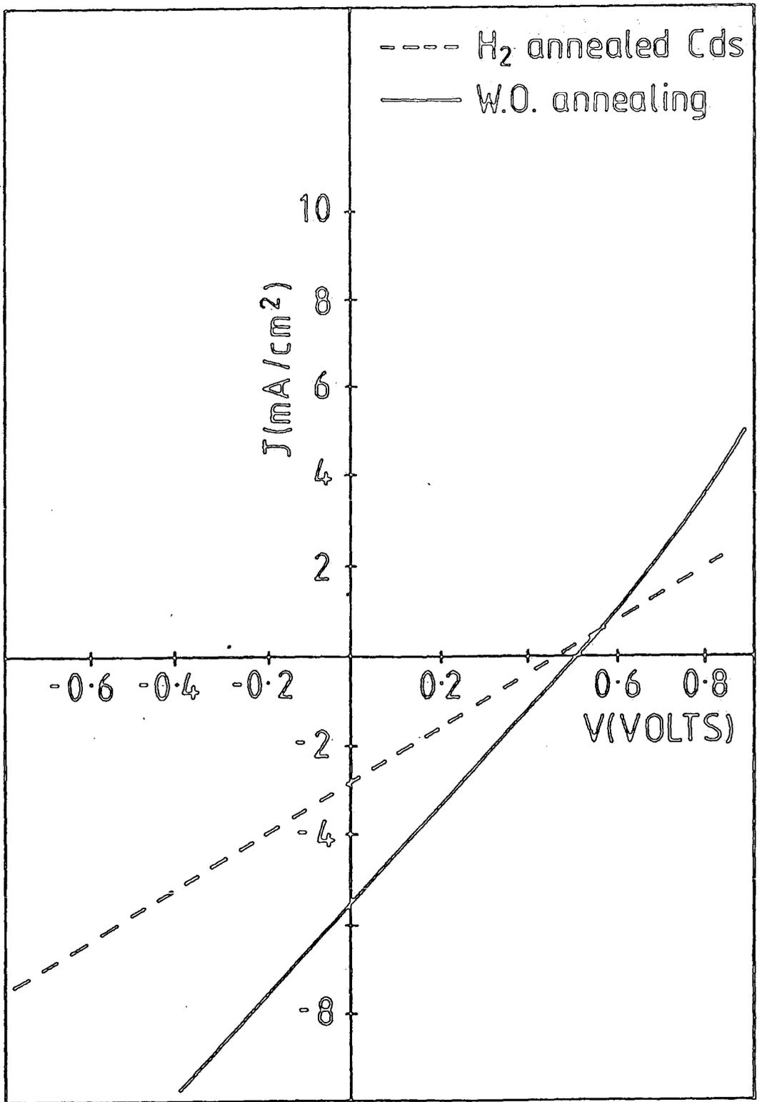
Fig. 8.12 : Photovoltaic behaviour of Hetrojunctions using Hydrogen annealed CdS layers.
