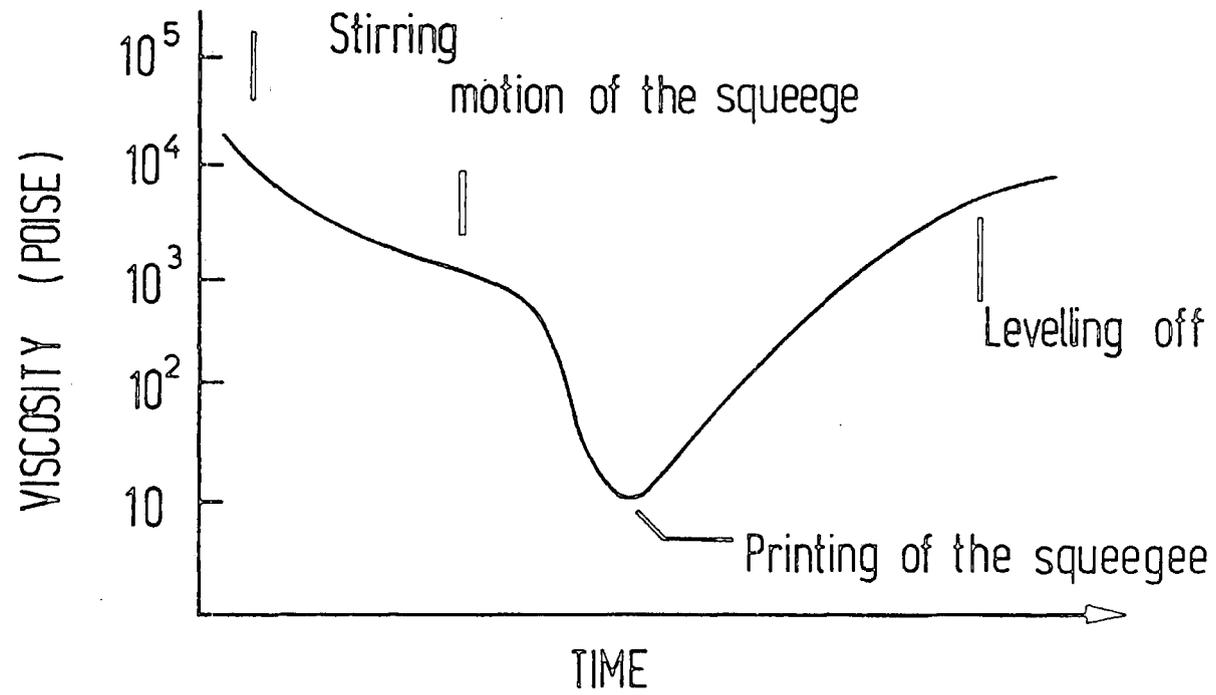
Fig. 4.6 Paste viscosity as a function of time (ref.4)
