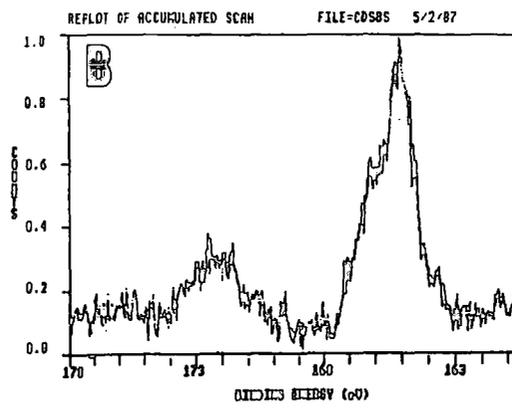
Fig. 6.24 ESCA spectra of S(2P) peaks in the high resolution scan
