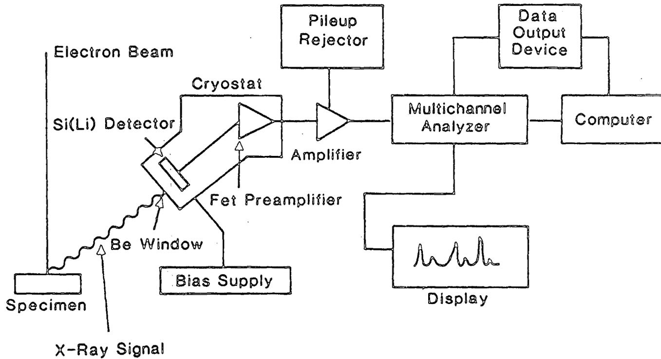
Figure 3.3 Energy dispersive X-ray analyser.
