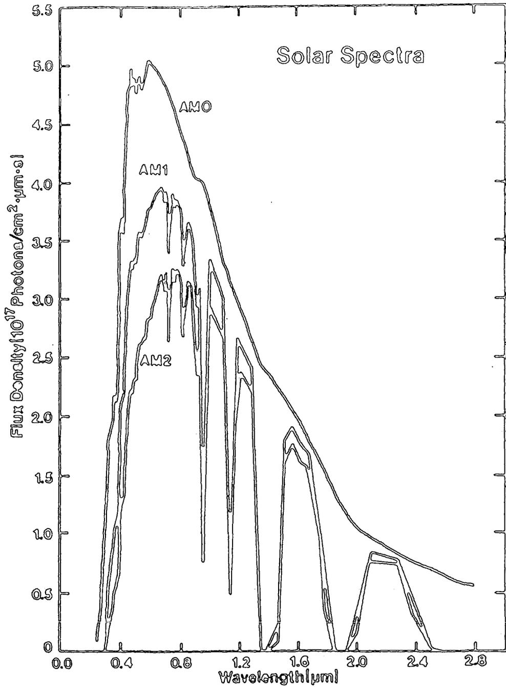
Figure 1.1 : Spectral distribution of solar radiation under different conditions.
