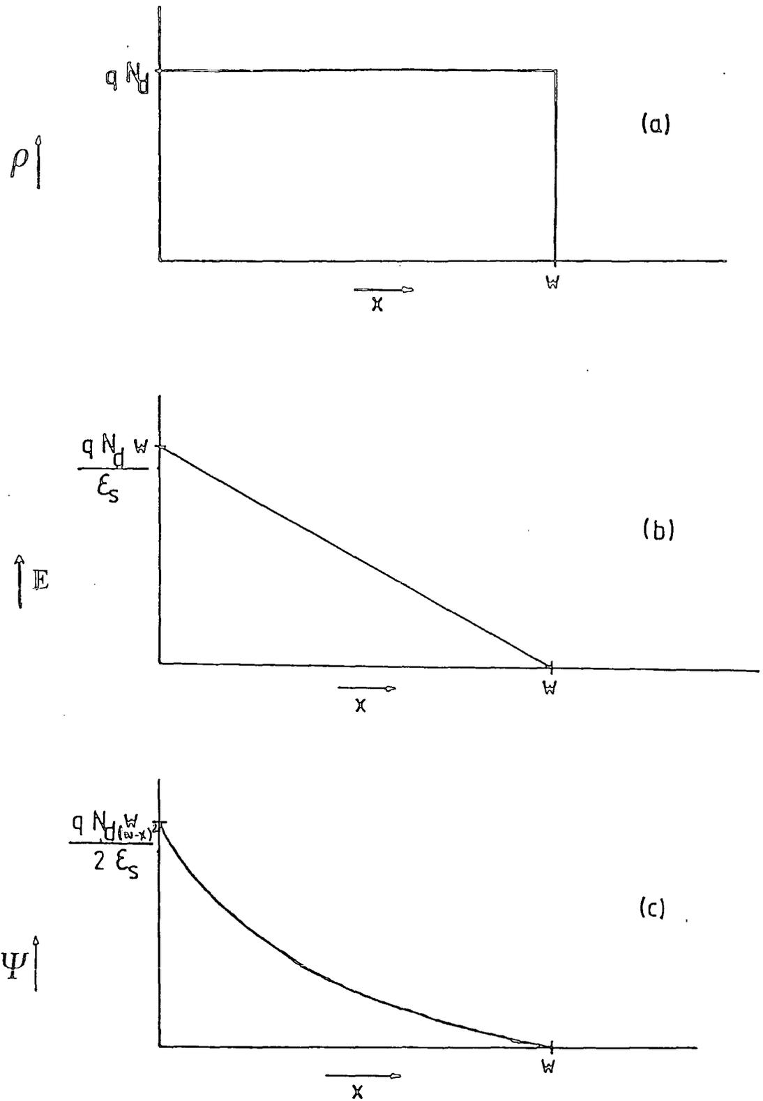
Fig. 2.1 : Variation of (a) charge density (b) electric field strength and (c) electrostatic potential with distance according to the depletion approximation.
