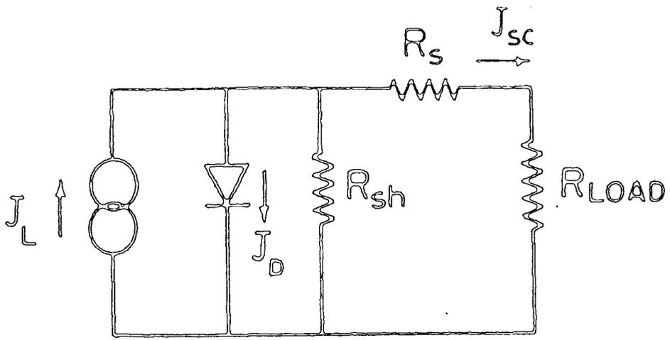
Fig. 2.6 : Equivalent circuit of a solar cell.
