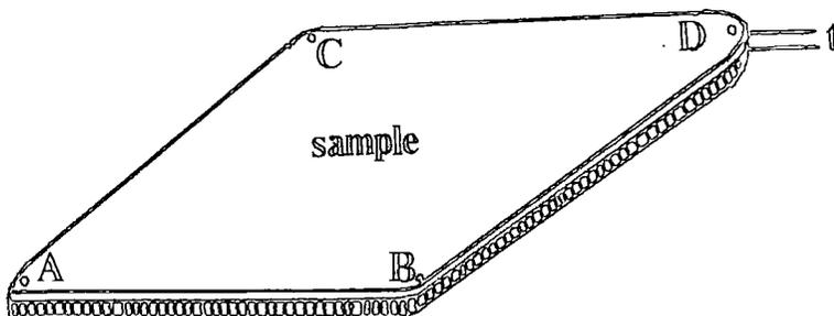
When a current  $I_{AB}$  is allowed to flow across the contacts A and B, a potential drop  $V_{CD}$  is produced between the contacts C and D. The ratio of  $V_{CD}$  to  $I_{AB}$  is defined as the resistance  $R_{AB,CD}$ . Similarly  $R_{BC,DA}$  is determined by establishing a current  $I_{BC}$  across the contacts B and C, and measuring the potential drop  $V_{DA}$  between the contacts D and A. The expression for the resistivity  $P$  is then given by
