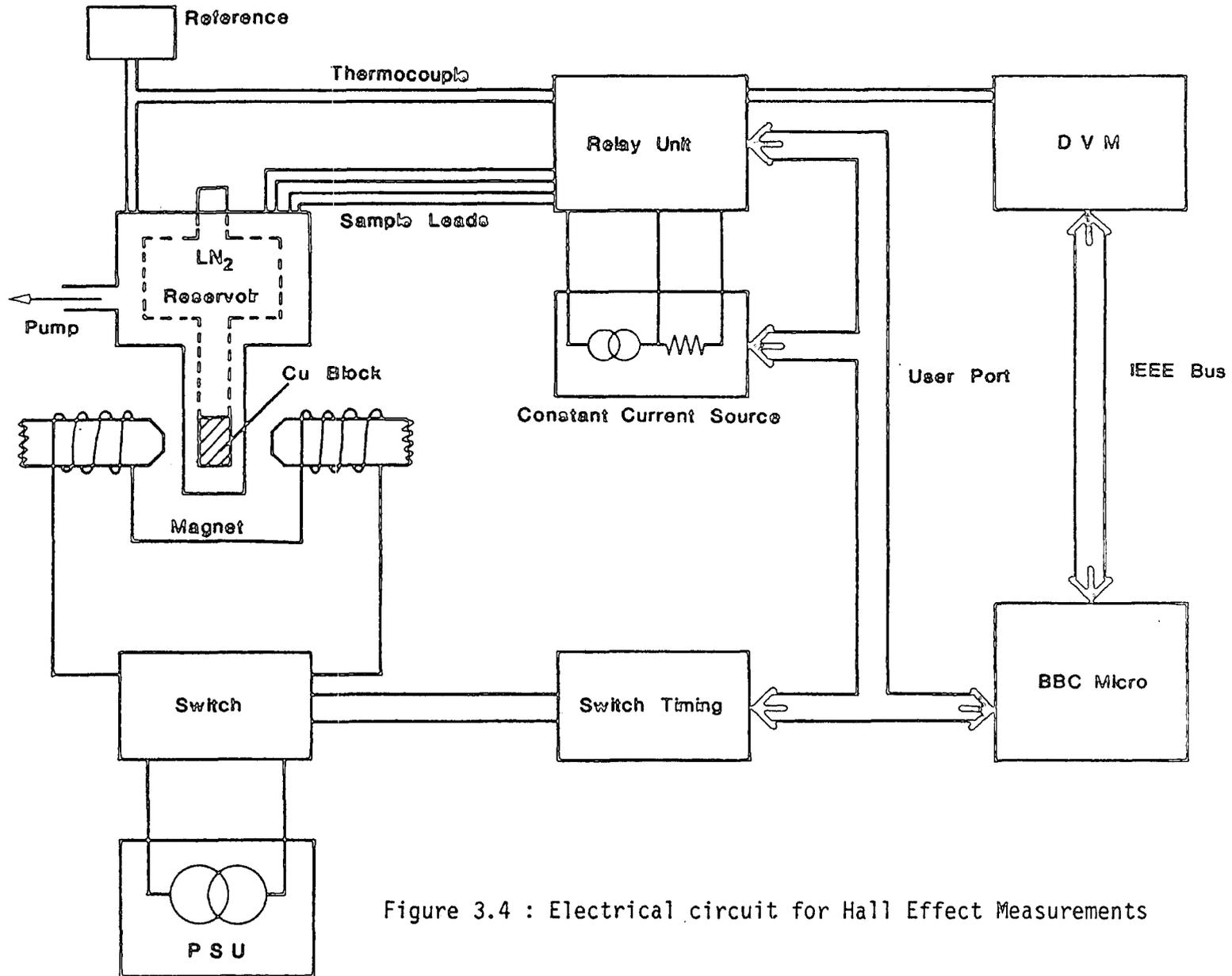
Figure 3.4 : Electrical circuit for Hall Effect Measurements
