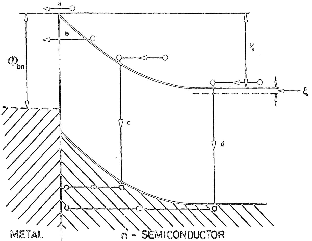
Fig. 2.4 : Current transport mechanisms in a forward-biased Schottky barrier
