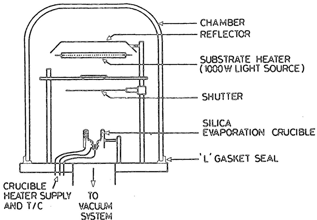
Figure 3.7 : Bell jar fixtures of the evaporator used in the deposition of CdTe films.
