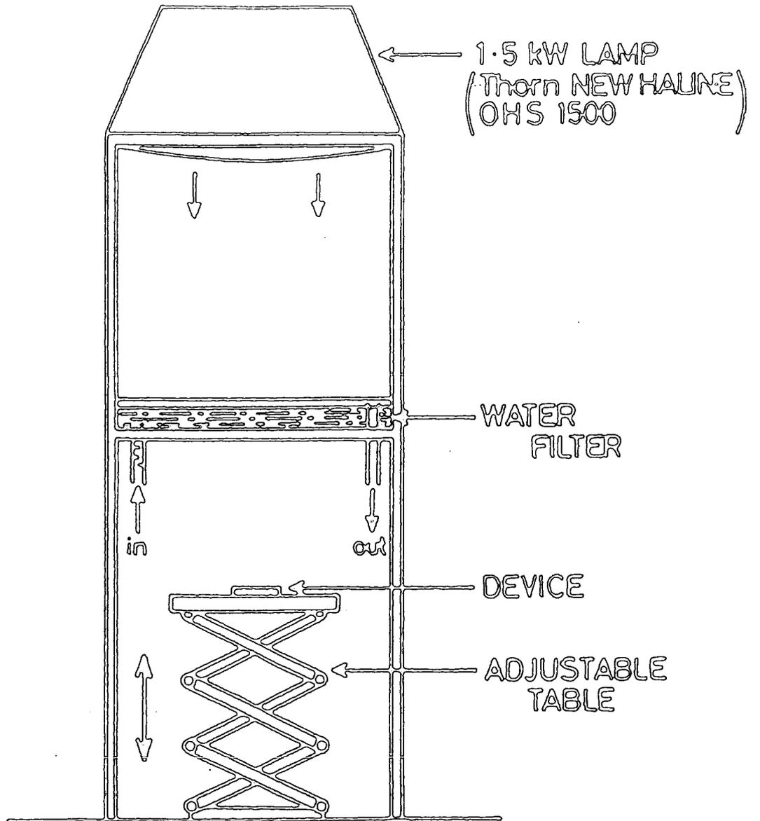
Figure 3.5 : Solar simulator for AMI illumination
