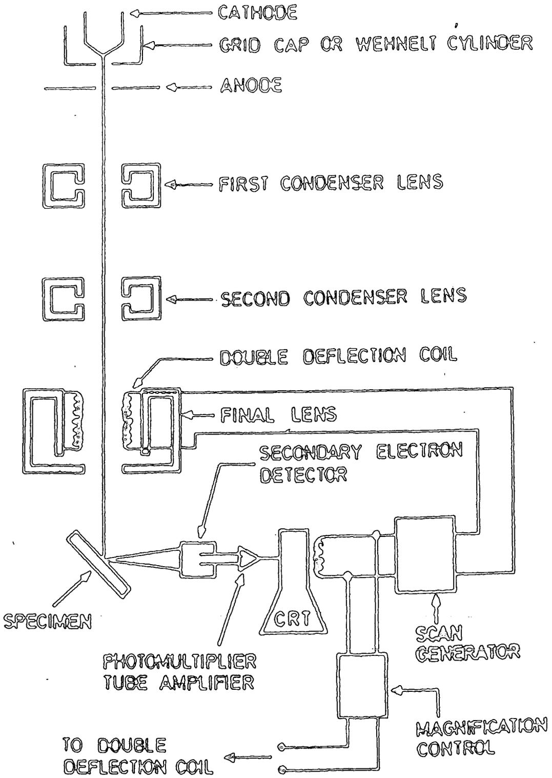
Figure 3.1 Schematic diagram of the SEM.
