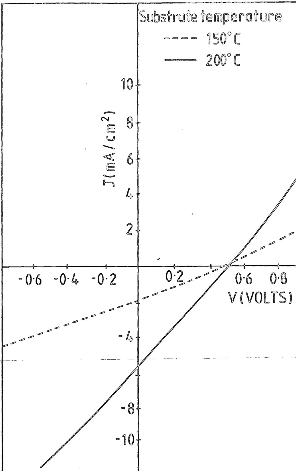
Fig. 8.2 : Photovoltaic behaviour of Hetrojunction using different CdTe layers.
