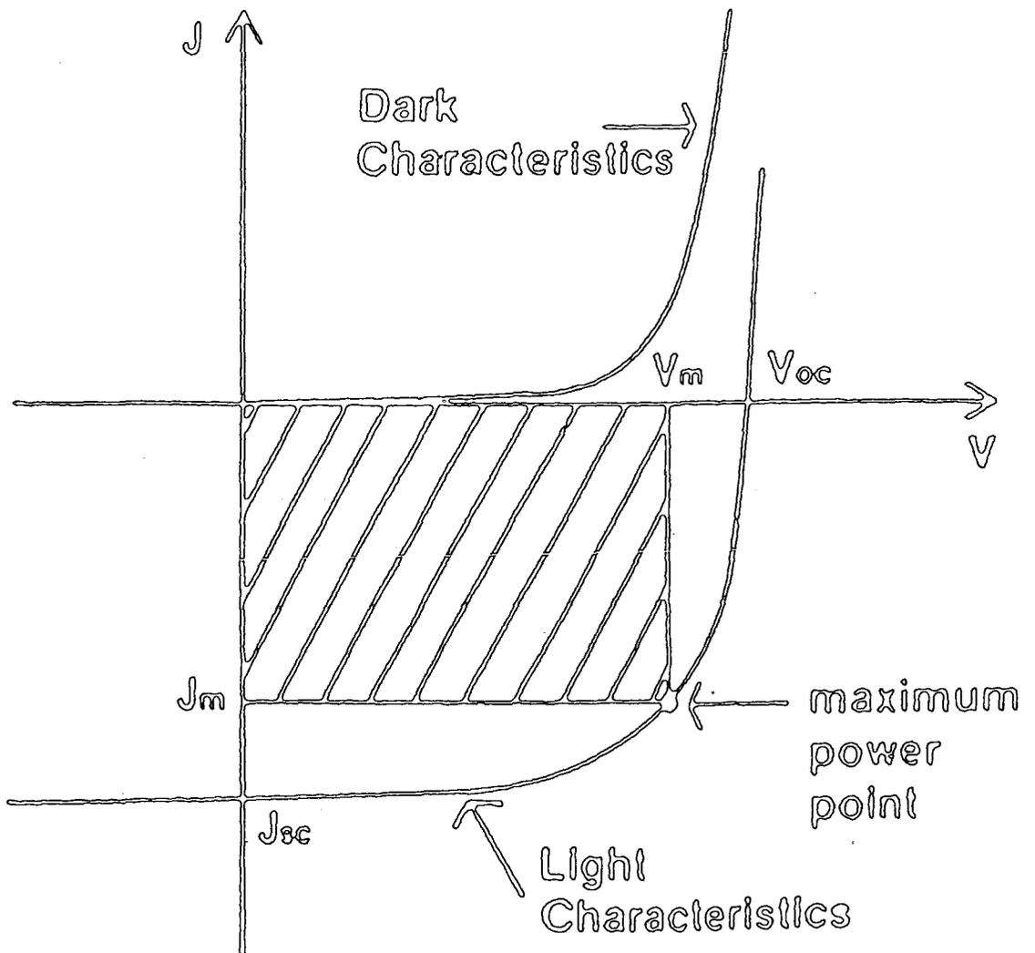
Fig. 2.7 : Typical dark and light J-V characteristics of an ideal solar cell
