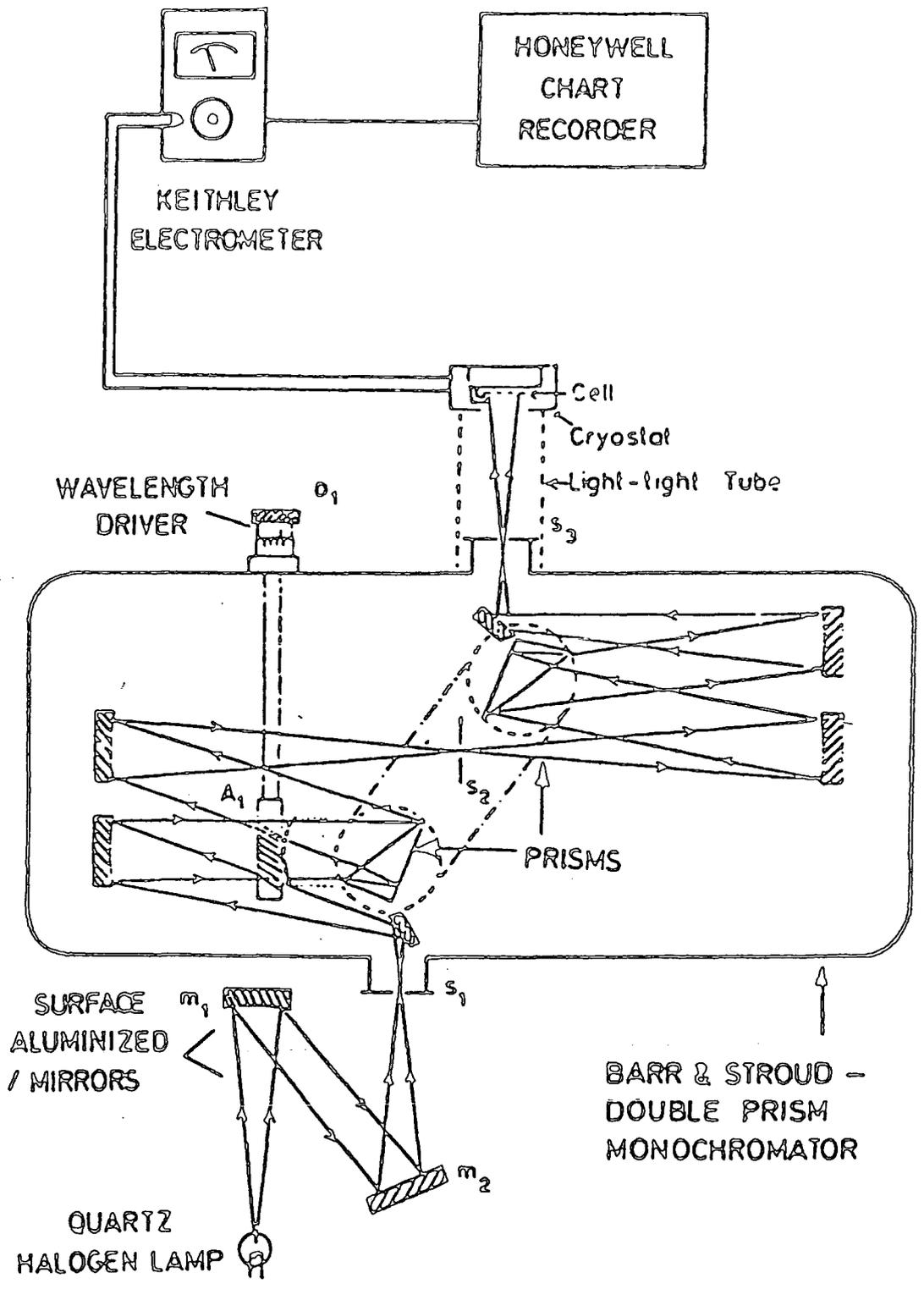
Figure 3.6 : Schematic diagram of spectral response measurement system.
