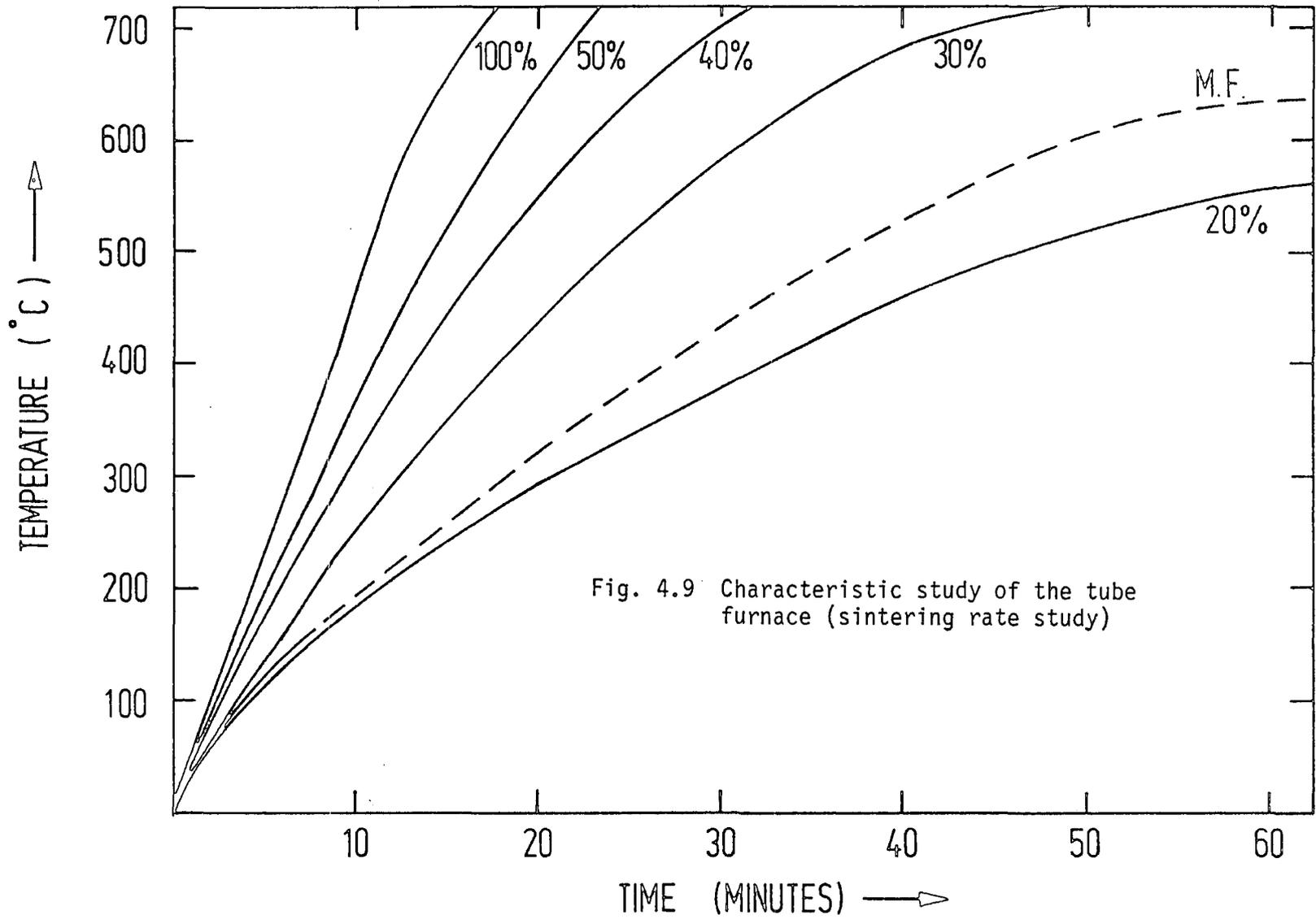
Fig. 4.9 Characteristic study of the tube furnace (sintering rate study)
