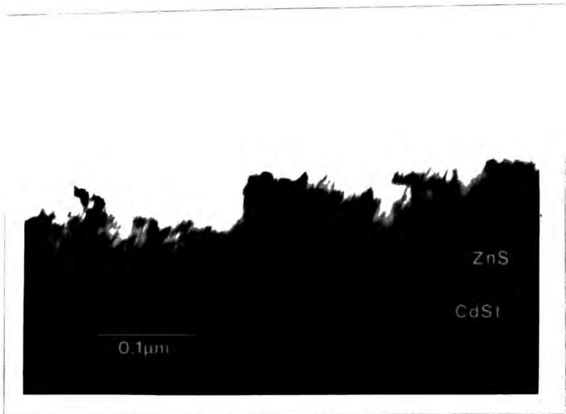
Figure 4.18a TEM micrograph of ZnS/CdSt/glass showing faint indications of columnar growth.
