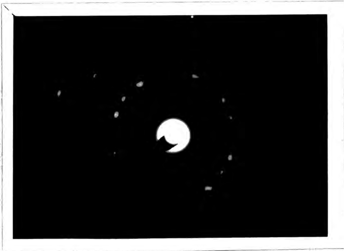
Figure 4.18b Associated SAD pattern demonstrating the polycrystalline nature of the epilayer and indicating a slight amount of preferential orientation.
