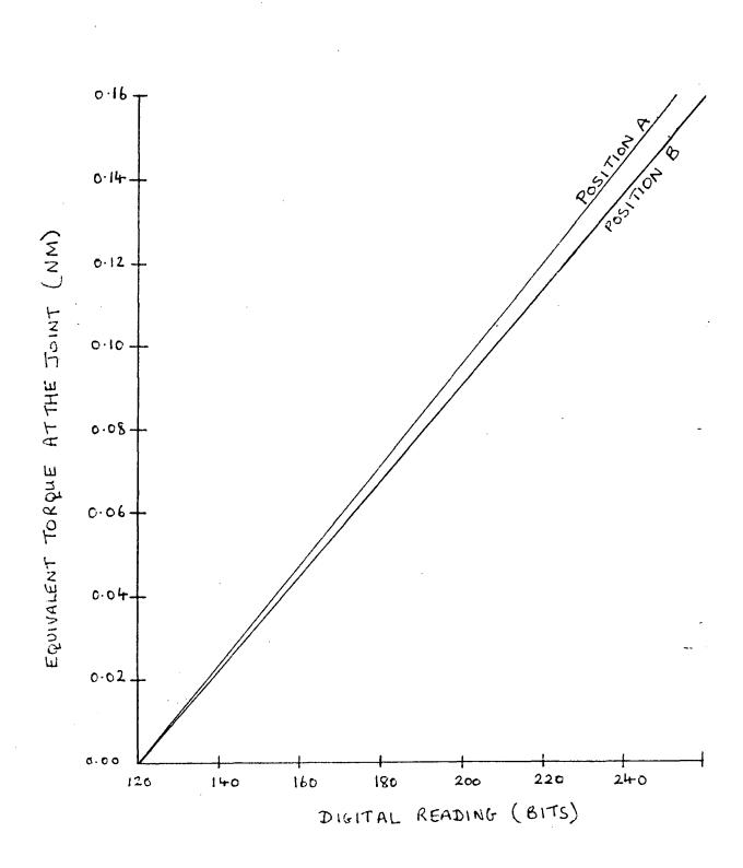
Fig. 4.7 Responses of the torque transducer loaded at A and B
