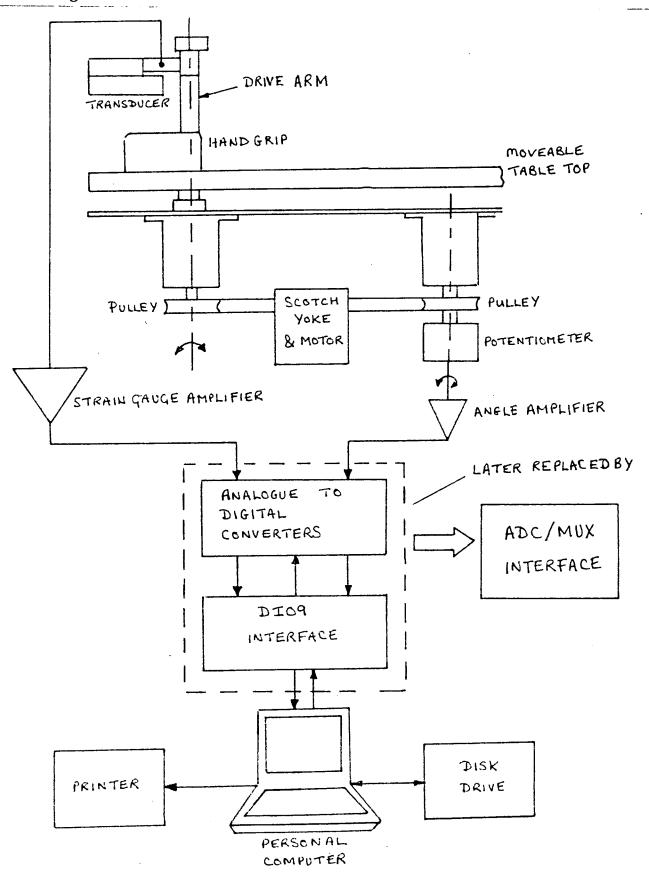
Fig. 4.5 Schematic diagram of the arthrograph
