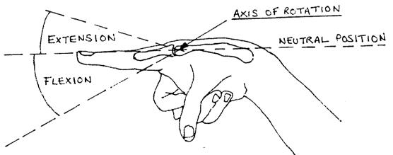
The proximal phalanx is caused to move by moments (or torques ) applied about the shown axis of rotation by the extensor tendon apparatus and the flexor tendon apparatus of the hand. The sum of the moments acting so as to move the joint into extension is known as the extension moment. Similarly, the sum of the moments acting to move the joint into flexion is known as the flexion moment.
