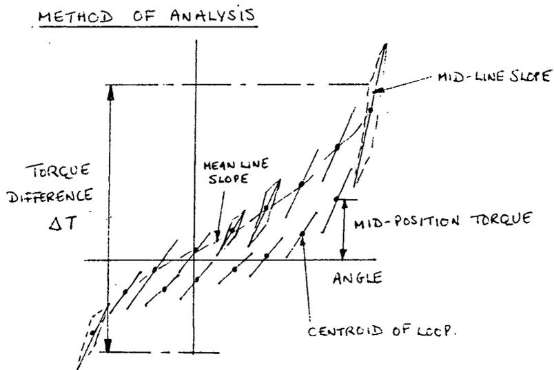
Figure 3.8 Idealised torque displacement characteristics
