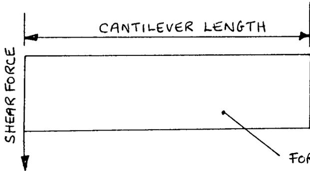
FOR THE SAME APPLIED LOAD, THE SHEAR FORCE ALONG THE LENGTH OF THE CANTILEVER IS CONSTANT, REGARDLESS OF POSITION.
