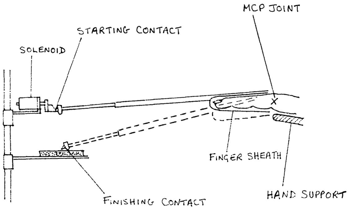
The time taken for the lever to fall through a ten degree arc from the neutral position was measured by a digital frequency meter, which was started and stopped by the opening and closing of contacts at either end of the ten degree arc. The complete system was capable of measuring fall times accurate to one millisecond.
