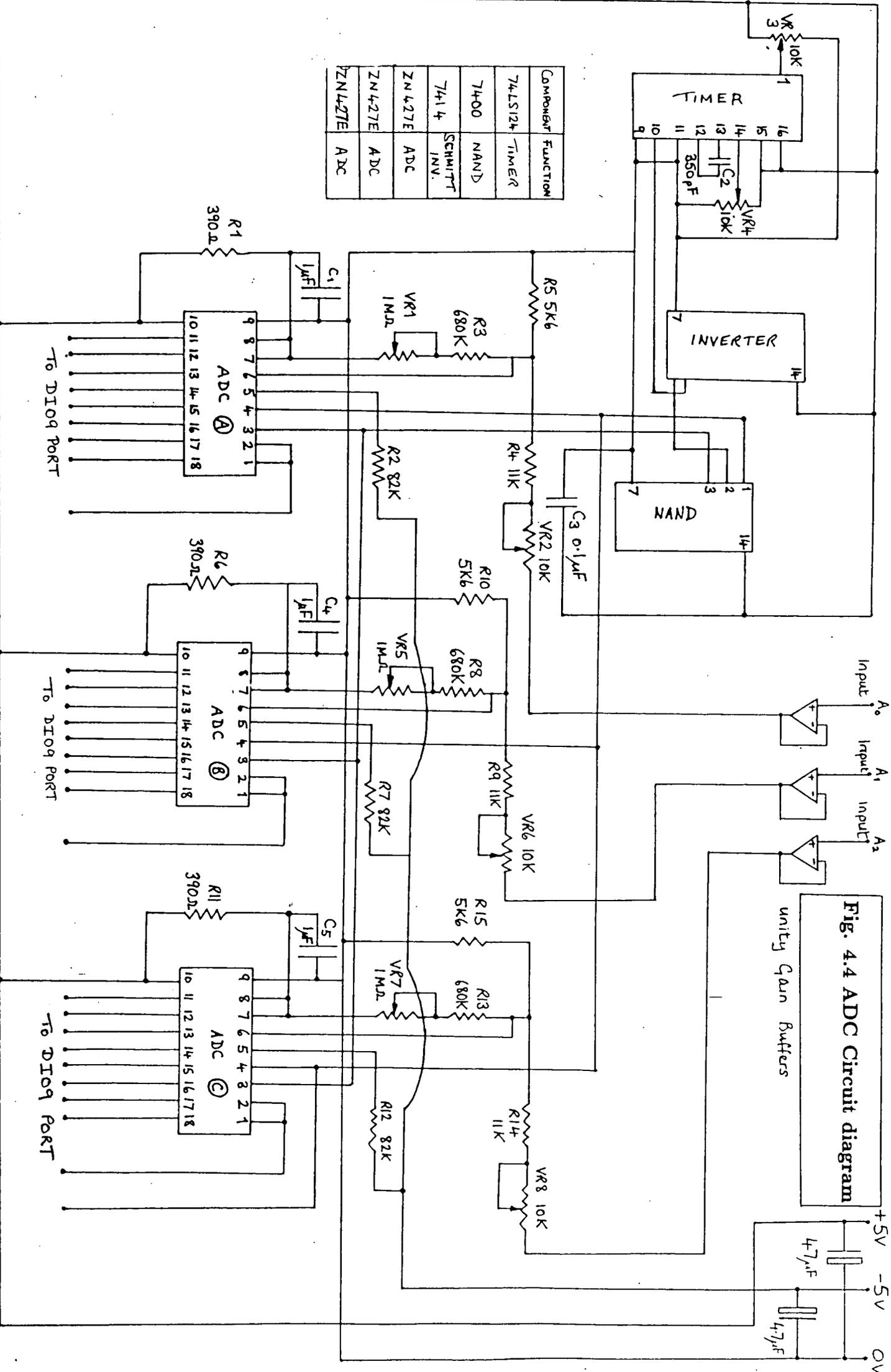
Fig. 4.4 ADC Circuit diagram
