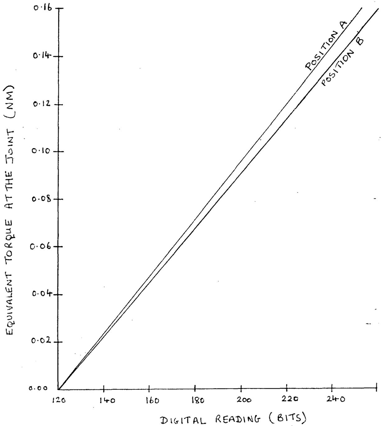
Fig. 4.8 Final Calibration curve for the torque transducer
