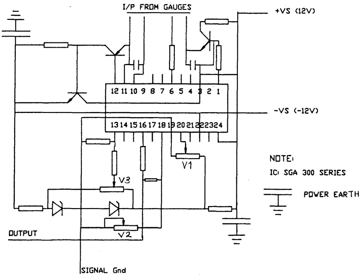
Potentiometers V1, V2 and V3 allowed adjustment of gain, range and zero offset respectively. The only real disadvantage of using this amplifier IC was that a warm up time of approximately five minutes was necessary before the output signal was free from drift. The amplifier circuit was mounted within the arthrograph body as close as possible to the transducer so that the length of the input lines, and hence the level of effect of external noise and signal distortion, was reduced.
