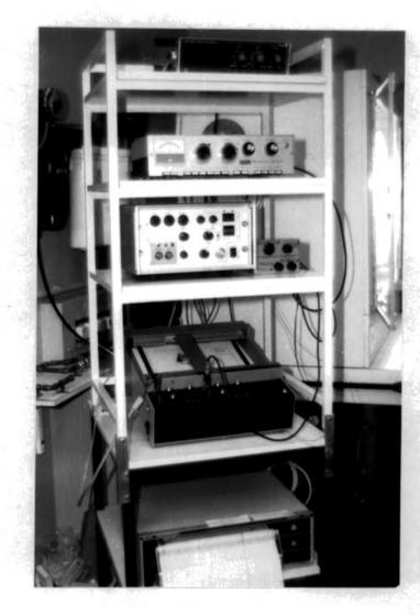
Figure 4.3 Photograph of the instrumentation associated with a conventional Langmuir trough.
