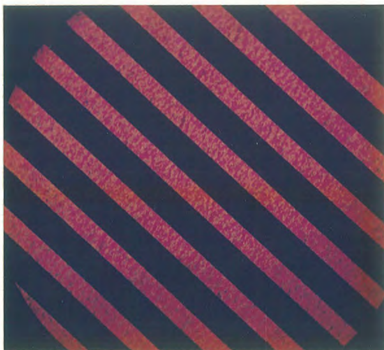
FIGURE 7.13(a) The texture of undyed GN3/3 immediately after alignment with 140V, 3 kHz sine wave, applied between interdigitated electrodes (60x magnification).
