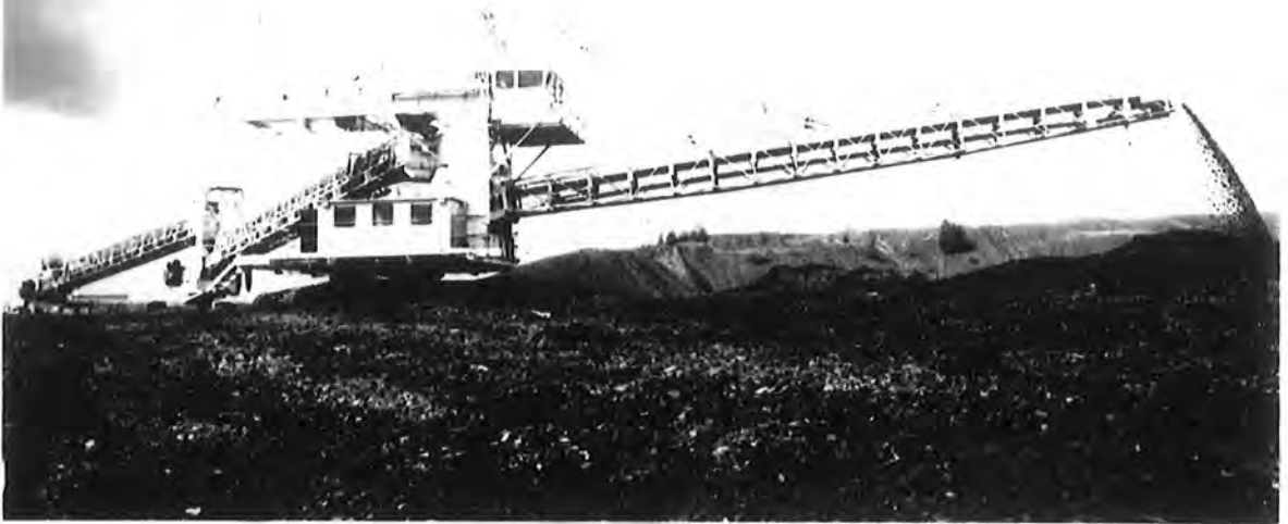
A 1,000 tonnes per hour Waste Disposal System for mine waste employed on an opencast site.
