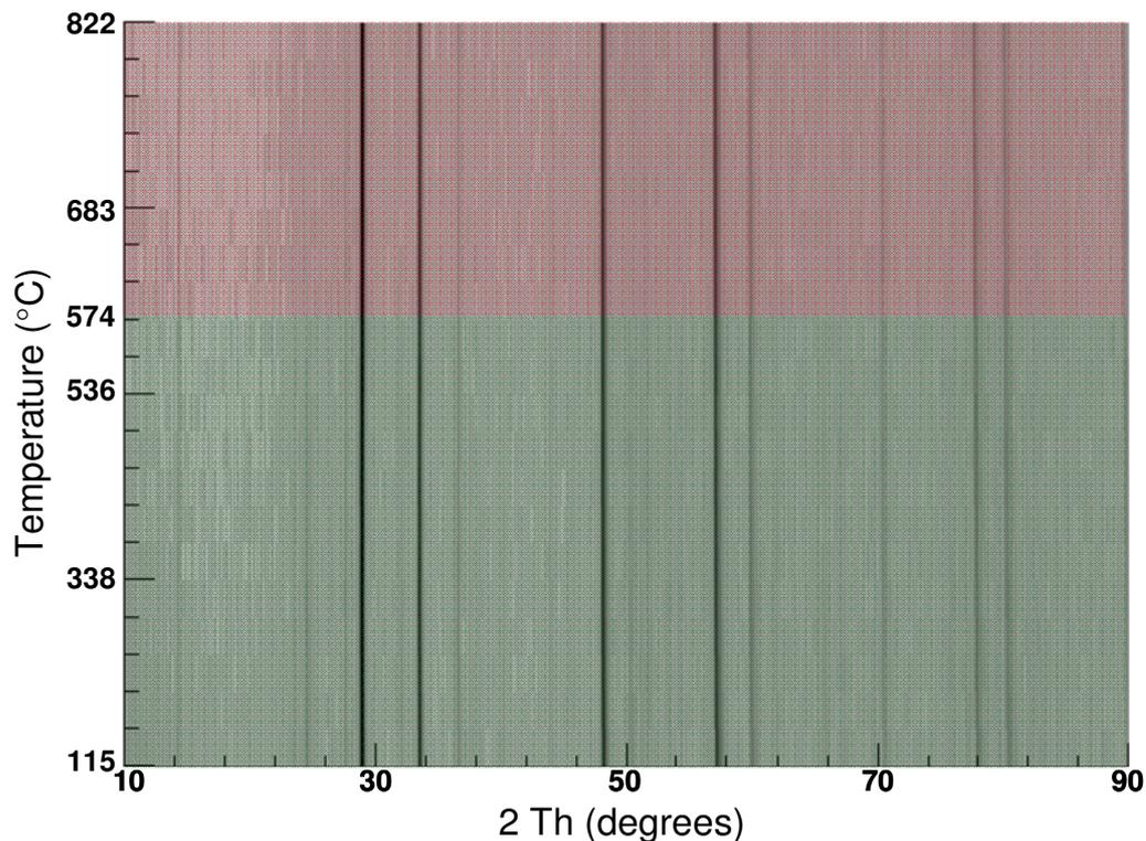
**Figure 4.24:** d8\_03758: VT-PXRD pattern of  $\text{Bi}_{1.8}\text{Ca}_{0.2}\text{Sn}_2\text{O}_{6.90}$ . Green patterns show stability region of  $\beta$  phase, whilst red patterns show the stability of the pyrochlore phase (up to 822 °C).
