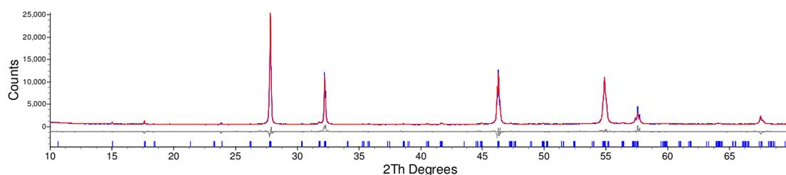
Figure 7.11: d9\_04599: Rietveld fit of  $\text{Bi}_{18.9}\text{Sr}_{0.1}\text{V}_2\text{O}_{33.45}$ .  $R_{\text{wp}} = 7.914\%$ .
