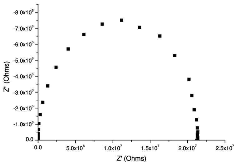
Figure 3.24: Complex impedance plot for  $\text{Bi}_2\text{Ti}_2\text{O}_7$  at 398 °C.
