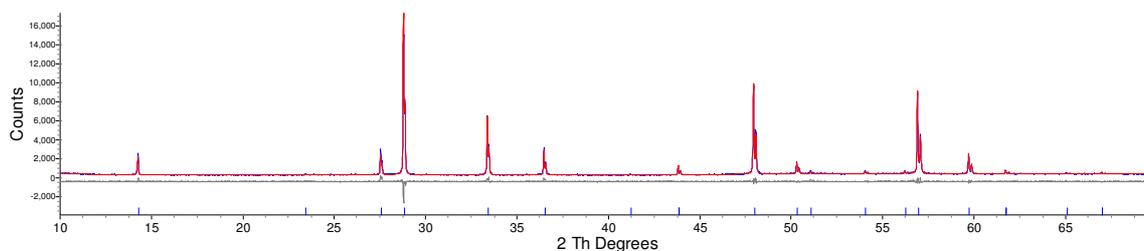
Figure 4.31: d9\_03284: Rietveld refinement for  $\text{Bi}_2\text{Sc}_{1.05}\text{Nb}_{0.95}\text{O}_{6.95}$ ,  $R_{\text{wp}} = 6.447\%$ .
