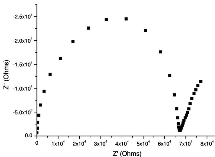
Figure 6.22: Impedance plot for  $\text{Bi}_6\text{W}_{0.95}\text{Nb}_{0.05}\text{O}_{11.975}$  at  $290\text{ }^\circ\text{C}$ .
