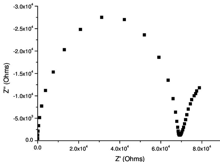
Figure 6.26: Complex impedance plot for  $\text{Bi}_6\text{W}_{0.95}\text{Zr}_{0.05}\text{O}_{11.95}$  at 192 °C.
