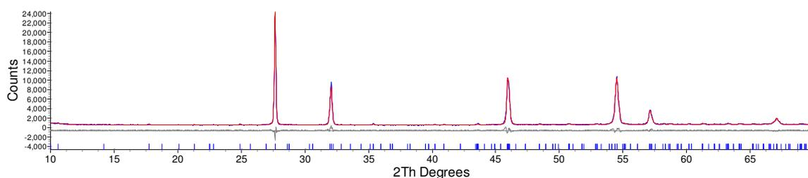
**Figure 6.28:** d9\_03885: Rietveld refinement for  $\text{Bi}_{5.6}\text{Er}_{0.4}\text{WO}_{12}$ .  $R_{\text{wp}} = 6.006\%$
