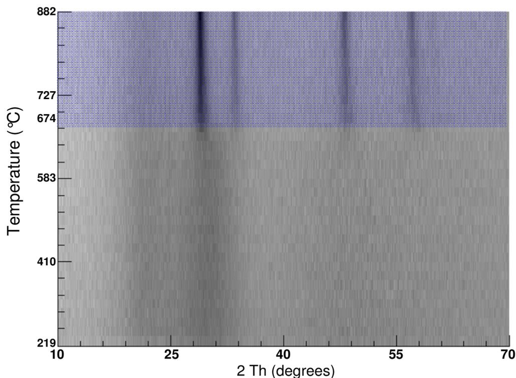
Figure 5.2: d8\_03593: *In-situ* VT-PXRD study of the  $\text{Nd}_2\text{Zr}_2\text{O}_7$  precursor.  $\text{Nd}_2\text{Zr}_2\text{O}_7$  forms at 674 °C. Below this temperature, the sample is amorphous.  $\text{Nd}_2\text{Zr}_2\text{O}_7$  stability range is shaded in pale blue.
