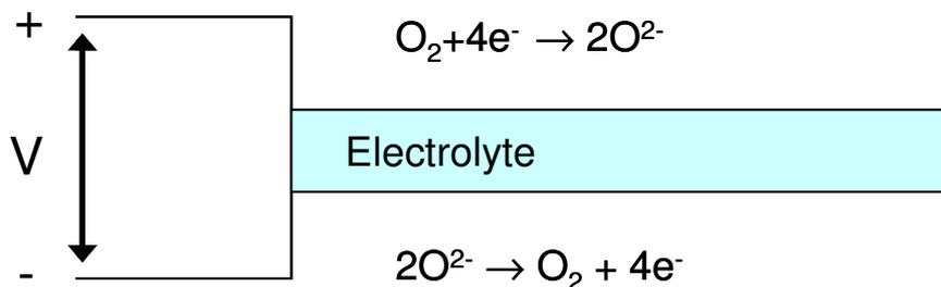
Figure 1.7: Diagram of an oxygen pump.<sup>20</sup>
