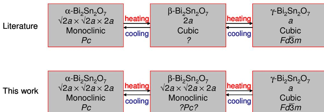
Figure 4.13: Phase transitions of  $\text{Bi}_2\text{Sn}_2\text{O}_7$  and relationship between the structures, highlighting our work which suggests an isosymmetrical phase transition for the  $\alpha\text{-Bi}_2\text{Sn}_2\text{O}_7$  to  $\beta\text{-Bi}_2\text{Sn}_2\text{O}_7$  phase transition.
