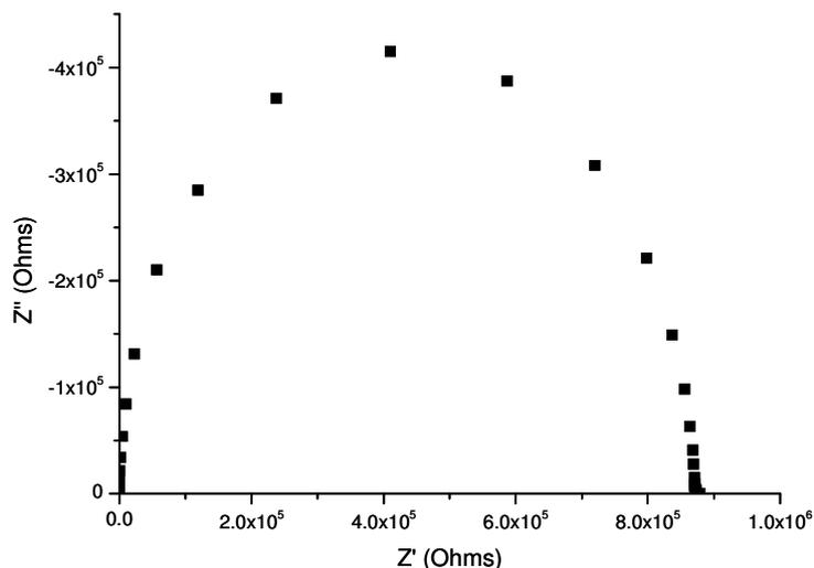
Figure 4.40: Complex impedance plot for  $\text{Bi}_2\text{ScNb}_{0.95}\text{Zr}_{0.05}\text{O}_{6.975}$  at 427 °C.
