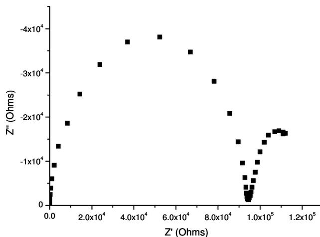
Figure 6.36: Complex impedance plot for  $\text{Bi}_{5.95}\text{Er}_{0.05}\text{W}_{0.90}\text{Zr}_{0.10}\text{O}_{11.90}$ .
