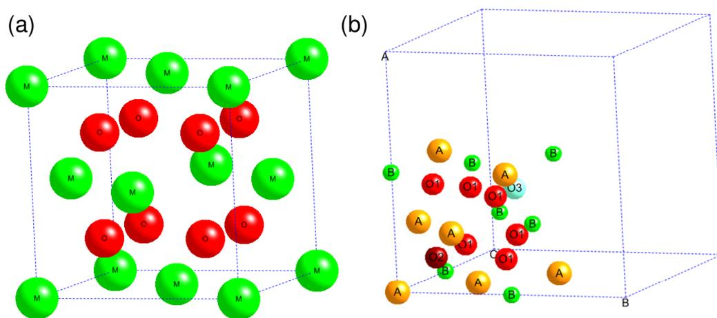
**Figure 1.1:** (a) Unit cell of  $\text{MO}_2$ , a typical fluorite. Green spheres are metal atoms and red spheres are oxygen atoms. (b) One-eighth of the pyrochlore  $\text{A}_2\text{B}_2\text{O}_7$  unit cell. Orange spheres are A cations, green spheres are B cations, red spheres are 48f oxygen, dark red spheres are 8a oxygen and the light blue sphere is the vacancy (8b).
