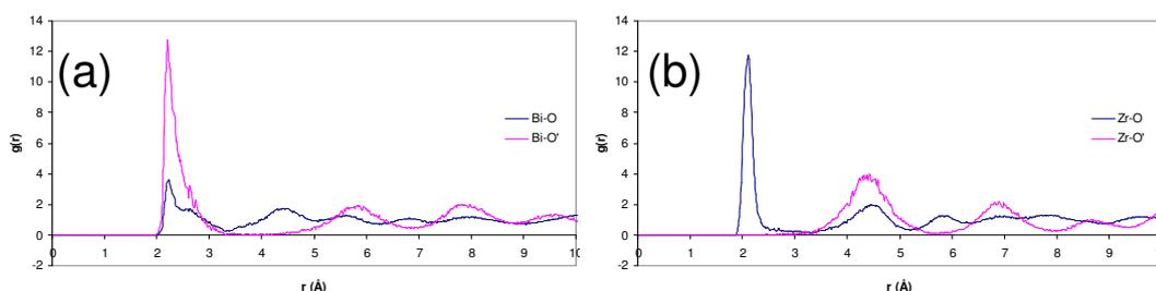
**Figure 3.9: Bond length distributions from RMCProfile refinements using a pyrochlore model for  $(\text{BiZr})_2\text{O}_7$ . (a) Bi-O and Bi-O' distributions and (b) Zr-O and Zr-O' distributions.**
