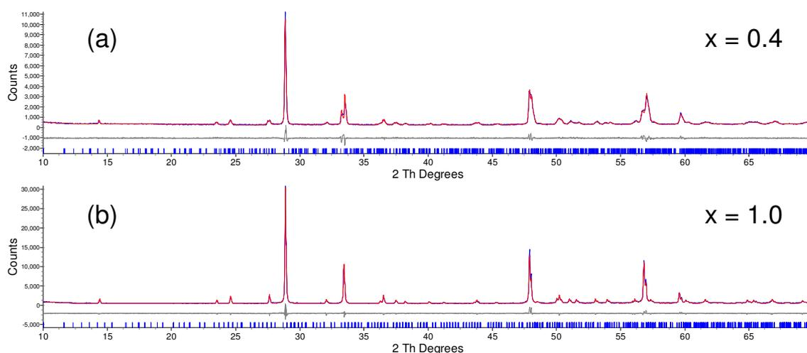
Figure 4.14: (a) d9\_04773:  $\text{Bi}_2\text{Sn}_{1.6}\text{Zr}_{0.4}\text{O}_7$  Rietveld refinement using the  $\alpha$ - $\text{Bi}_2\text{Sn}_2\text{O}_7$  model. (b) d9\_04743:  $\text{Bi}_2\text{SnZrO}_7$  Rietveld refinement using the  $\alpha$ - $\text{Bi}_2\text{Sn}_2\text{O}_7$  model.
