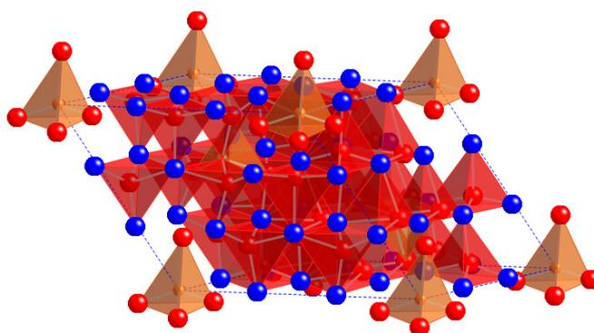
**Figure 7.1:** Kashida’s model of  $\text{Bi}_9\text{VO}_{16}$ . Orange polyhedra are  $\text{VO}_4$  tetrahedra, red polyhedra are  $\text{OBi}_4$  tetrahedra, blue spheres are bismuth atoms, orange spheres are vanadium atoms and red spheres are oxygen atoms.
