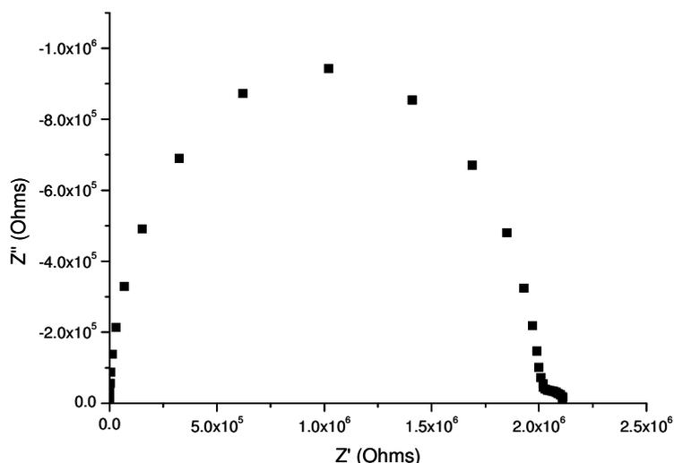
**Figure 4.29: Complex impedance plot for  $\text{Bi}_2\text{ScNbO}_7$  at 387 °C.**
