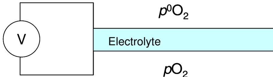
Figure 1.6: Diagram of a typical oxygen sensor.<sup>20</sup>
