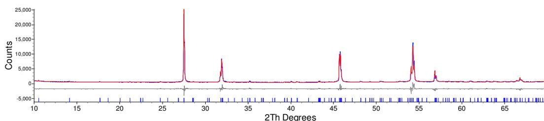
Figure 6.21: d9\_03745:  $\text{Bi}_6\text{W}_{0.9}\text{Nb}_{0.1}\text{O}_{11.95}$ .  $R_{\text{wp}} = 8.692\%$
