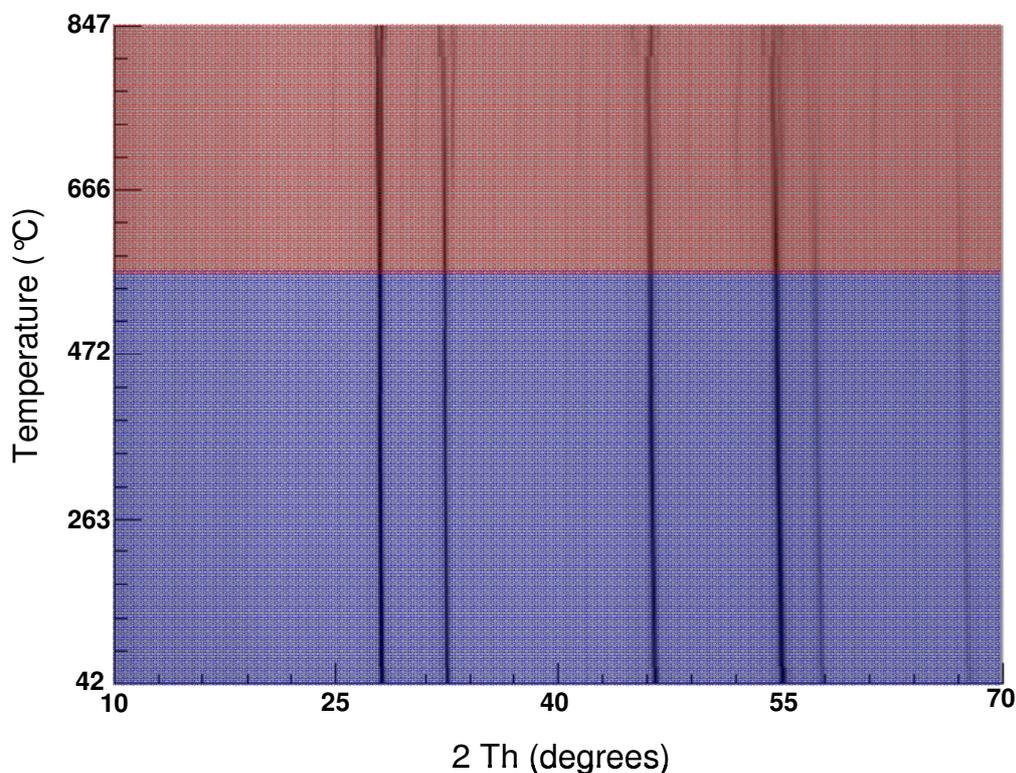
Figure 7.7: d9\_04850: VT-PXRD on  $\text{Bi}_{18.9}\text{Ca}_{0.1}\text{V}_2\text{O}_{33.45}$ . No phase transitions were observed over the temperature range studied and partial decomposition occurred at 571 °C and above. Pale blue region represents stability range, whilst light red region represents decomposition ranges.
