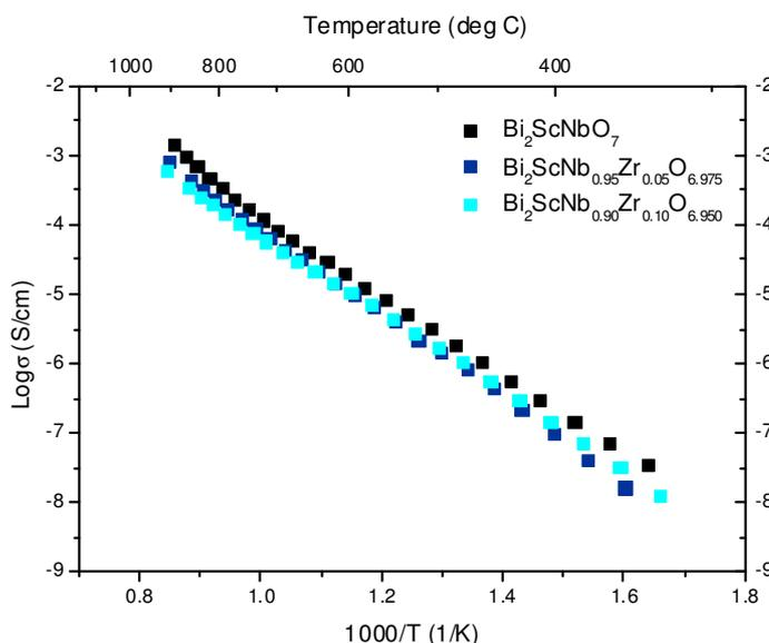
Figure 4.41: Plot of variation of conductivity versus temperature for the  $\text{Bi}_2\text{ScNb}_{1-x}\text{Zr}_x\text{O}_{7-x/2}$  system.
