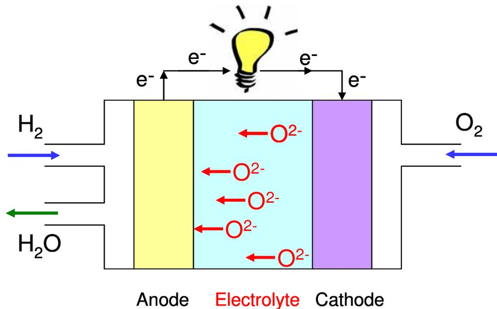
**Figure 1.5: Diagram of a typical solid oxide fuel cell.**
