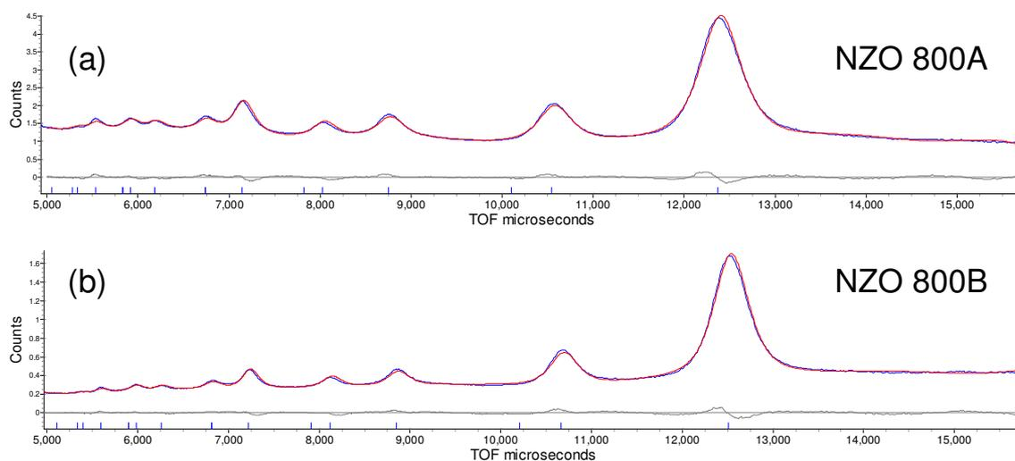
**Figure 5.5: GEM43539: Refinement for NZO 800A using a fluorite model and 3 banks of data. Bank 5 (91.3°) is shown.  $R_{wp} = 2.317\%$ ,  $a = 5.2590(2)$  Å. (b) GEM43540: Rietveld refinement for NZO 800B. using 3 banks of data and a fluorite model.  $R_{wp} = 2.476\%$ ,  $a = 5.3176(1)$  Å. Bank 5 (91.3°) is shown.**
