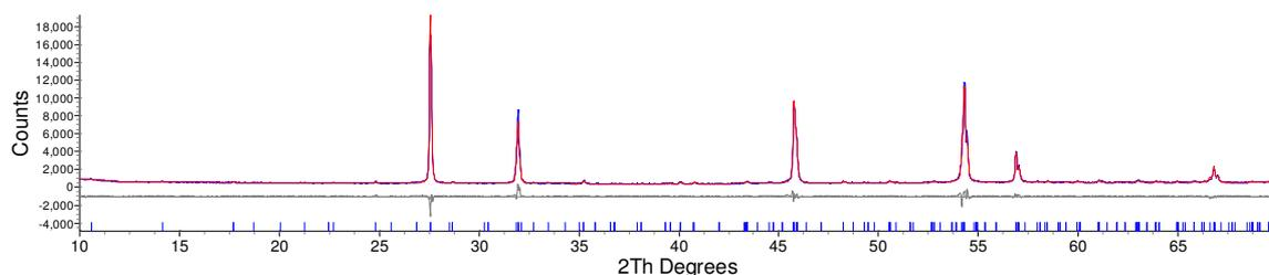
Figure 6.24: d9\_03900: Rietveld refinement for  $\text{Bi}_6\text{W}_{0.90}\text{Zr}_{0.10}\text{O}_{11.90}$ .  $R_{wp} = 6.838\%$ .
