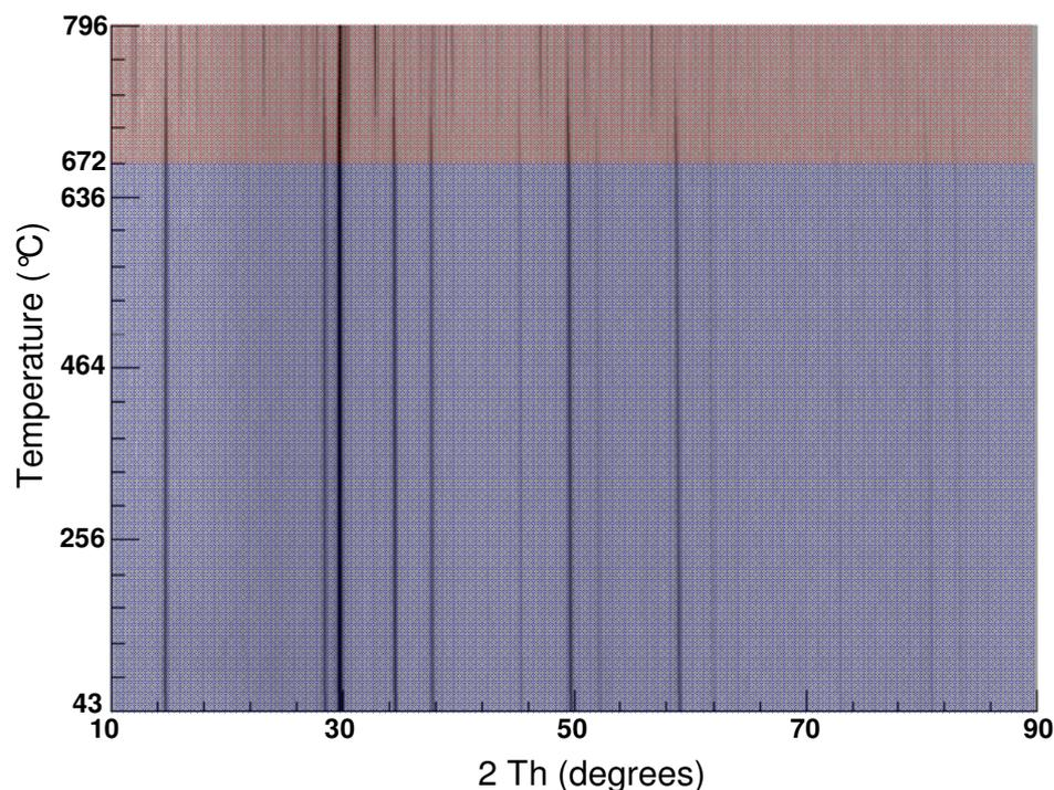
Figure 3.13: *In-situ* VT-PXRD of  $\text{Bi}_2\text{Ti}_2\text{O}_7$ . Decomposition occurs at 672 °C. Pale blue regions represent the stability range and the pale red regions show multiphase regions after decomposition.
