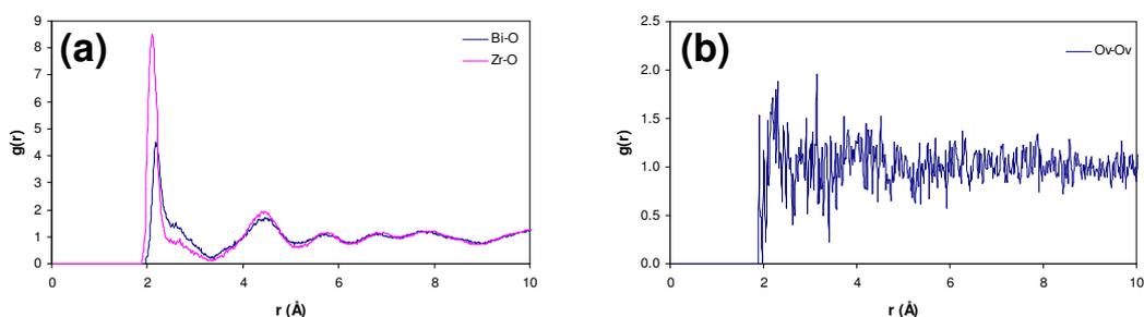
Figure 3.7: (a) Zr-O and Bi-O partial  $g(r)$  and (b) Ov-Ov partial  $g(r)$  as obtained from a RMCProfile fit using a  $(\text{BiZr})_2\text{O}_7$  fluorite starting configuration.
