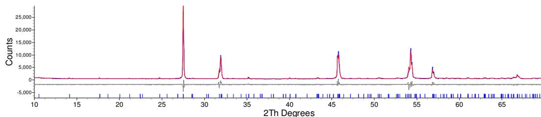
Figure 6.18: d9\_03821: Rietveld fit for  $\text{Bi}_{5.8}\text{Ca}_{0.2}\text{WO}_{11.9}$ .  $R_{\text{wp}} = 9.740\%$ .
