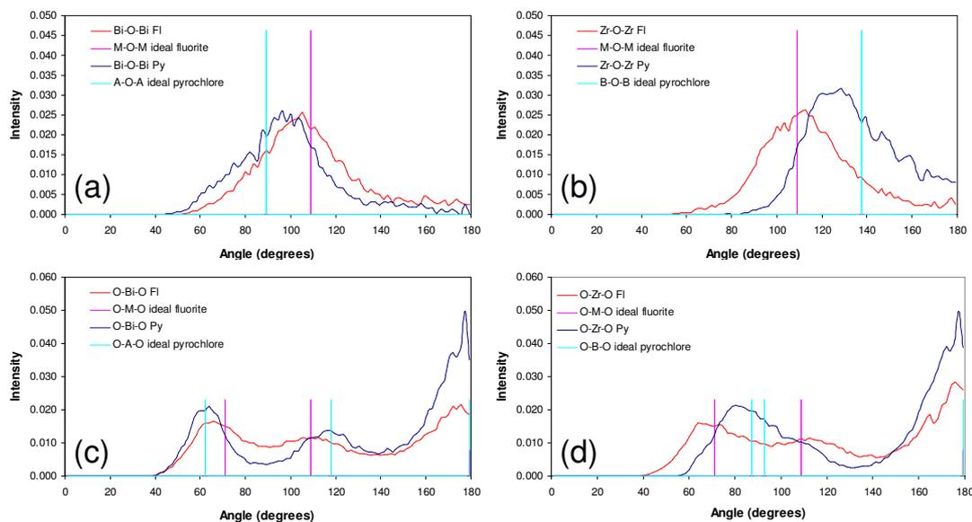
**Figure 3.11**  $(\text{BiZr})_2\text{O}_7$  bond angle outputs from RMCProfile fitting. (a) Bi-O-Bi angles, (b) Zr-O-Zr angles, (c) O-Bi-O angles and (d) O-Zr-O angles. Ideal fluorite pink, ideal pyrochlore light blue. RMC fluorite red, RMC pyrochlore blue.
