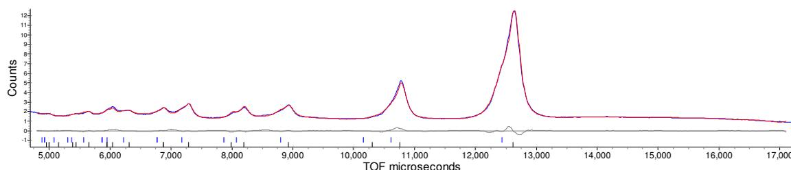
**Figure 3.5: Rietveld fit for  $(\text{BiZr})_2\text{O}_7$  using powder neutron diffraction data.  $R_{wp} = 2.948\%$ .**
