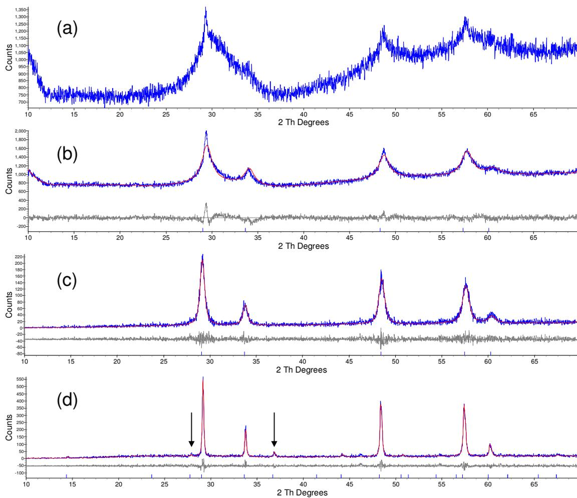
**Figure 5.1:**  $\text{Nd}_2\text{Zr}_2\text{O}_7$  after firing at different temperatures. (a) d9\_02696:  $\text{Nd}_2\text{Zr}_2\text{O}_7$  after firing at 600 °C. (b) and (c) are refinements using a fluorite model. (b) d9\_02697:  $\text{Nd}_2\text{Zr}_2\text{O}_7$  after firing at 700 °C. (c) d5\_07671:  $\text{Nd}_2\text{Zr}_2\text{O}_7$  after firing at 900 °C. (d) d5\_07691:  $\text{Nd}_2\text{Zr}_2\text{O}_7$  after firing at 1200 °C, refinement using a pyrochlore model.
