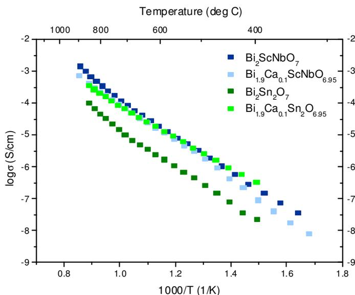
**Figure 4.38:** Comparison of the conductivities for  $\text{Bi}_2\text{ScNbO}_7$  and  $\text{Bi}_2\text{Sn}_2\text{O}_7$  and their 0.1 Ca doped analogues.
