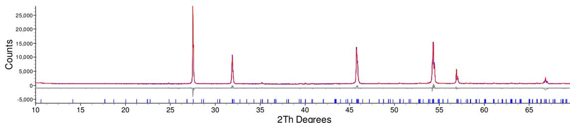
**Figure 6.35:** d9\_04121: Rietveld fit for  $\text{Bi}_{5.95}\text{Er}_{0.05}\text{W}_{0.90}\text{Zr}_{0.10}\text{O}_{11.90}$ .  $R_{wp} = 6.734\%$ .
