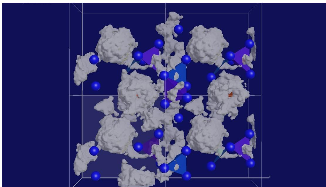
Figure 6.16:  $ab$  plane showing oxygen diffusion between  $\text{WO}_x$  and  $\text{OBi}_4$  units at 1173 K. Blue spheres are bismuth atoms, blue polyhedra are  $\text{OBi}_4$  units and orange polyhedra are  $\text{WO}_x$  units.
