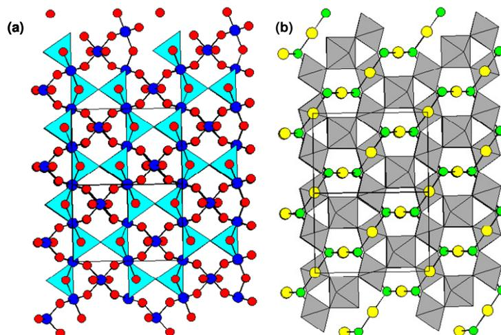
**Figure 1.3:** View of the two interpenetrating networks of the pyrochlore structure. (a) shows the  $A_2O'$  network of corner sharing,  $O'A_4$ , tetrahedra (blue). Blue spheres are B cations and red spheres are 48f oxygens respectively. (b) shows the  $B_2O_6$  network of corner sharing  $BO_6$  octahedra (grey). Yellow spheres are A cations and green spheres are  $O'$ .
