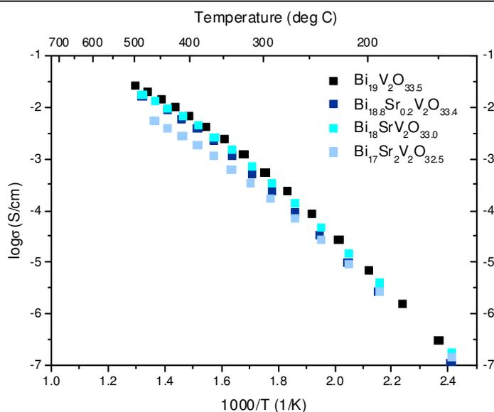
Figure 7.15: Arrhenius plot of conductivity showing  $\text{Bi}_{19-x}\text{Sr}_x\text{V}_2\text{O}_{33.5-x/2}$  phases.
