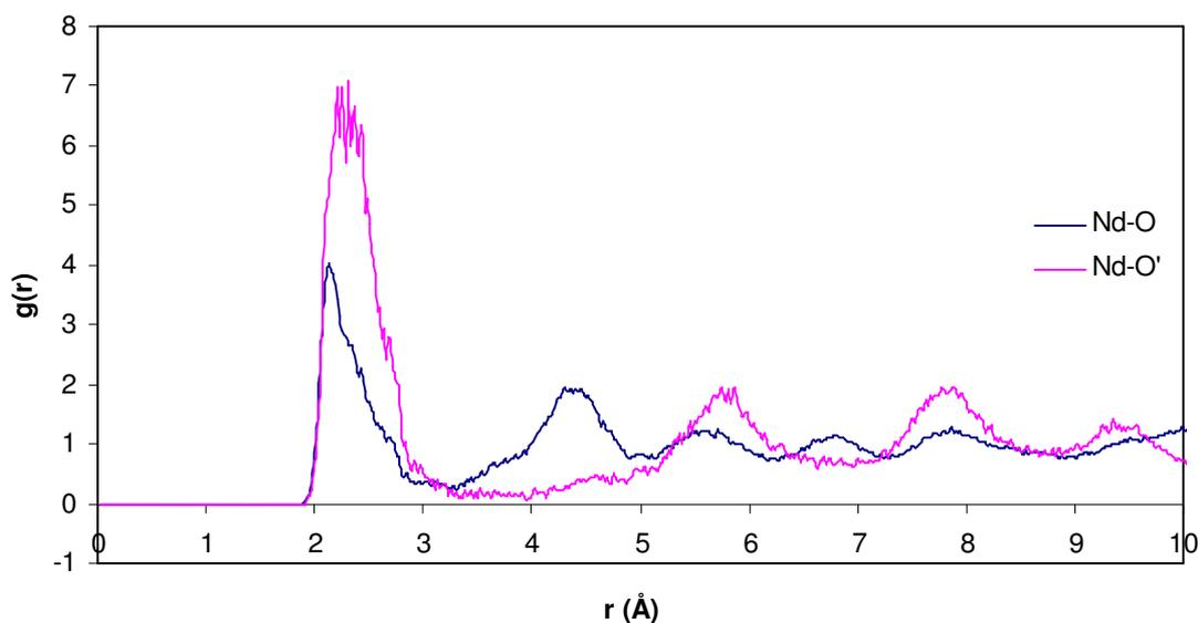
Figure 5.14: Nd-O and Nd-O' partial  $g(r)$  which indicate bond length distributions. These have been obtained from RMC simulations using a  $\text{Nd}_2\text{Zr}_2\text{O}_7$  pyrochlore starting configuration.
