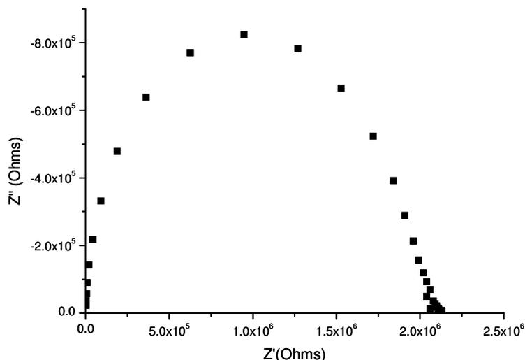
Figure 4.20: Complex impedance plot of  $\text{Bi}_2\text{Sn}_2\text{O}_7$  at  $470 \text{ }^\circ\text{C}$ .
