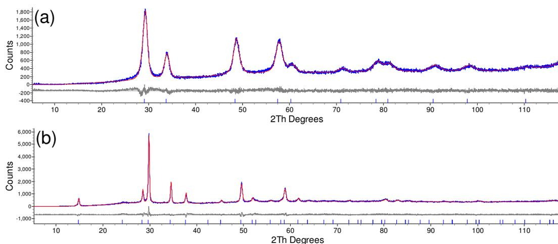
Figure 3.20: (a) d5\_07560:  $(\text{BiZr}_{0.8}\text{Ti}_{0.2})_2\text{O}_7$ . Rietveld fit using a single fluorite model.  $R_{\text{wp}} = 6.913\%$
