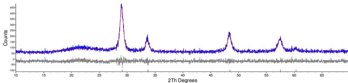
**Figure 5.3:** d8\_03593 range 37 (19 °C):  $\text{Nd}_2\text{Zr}_2\text{O}_7$  synthesised *in-situ* in the diffractometer, post VT-PXRD and after cooling to room temperature. Rietveld refinement using a fluorite structural model.  $R_{\text{wp}} = 11.065\%$ ,  $a = 5.311(8)$  Å.
