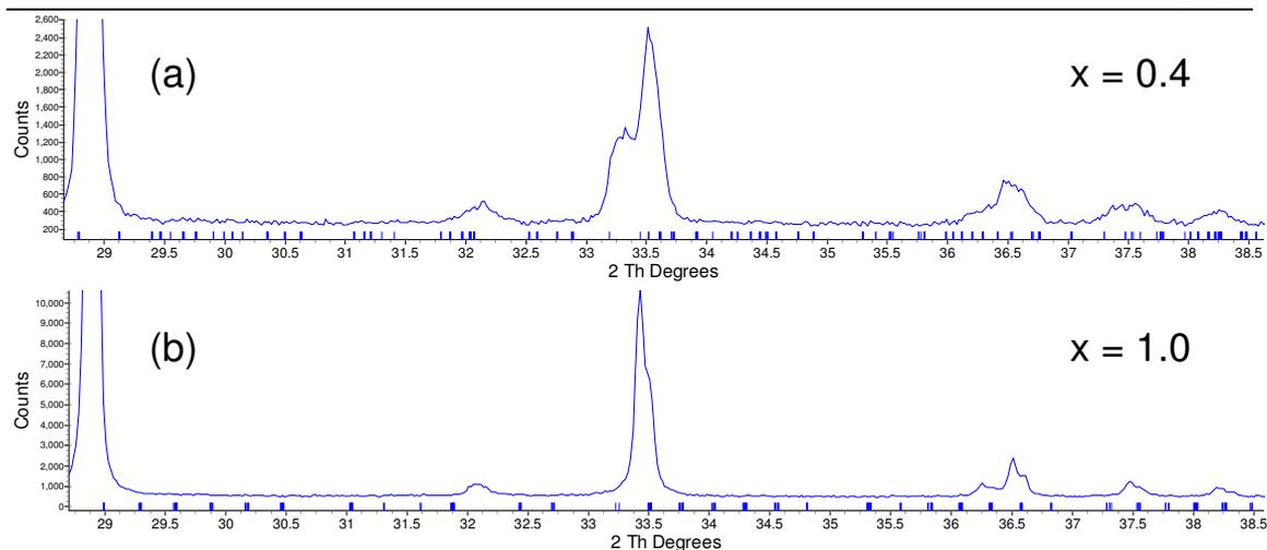
Figure 4.15: (a) d9\_04773:  $\text{Bi}_2\text{Sn}_{1.6}\text{Zr}_{0.4}\text{O}_7$  zoomed region showing peak centred around  $33.5^\circ$ , characteristic of  $\alpha\text{-Bi}_2\text{Sn}_2\text{O}_7$ . (b) d9\_04743:  $\text{Bi}_2\text{SnZrO}_7$  zoomed region showing peak centred around  $33.5^\circ$ , characteristic of  $\beta\text{-Bi}_2\text{Sn}_2\text{O}_7$
