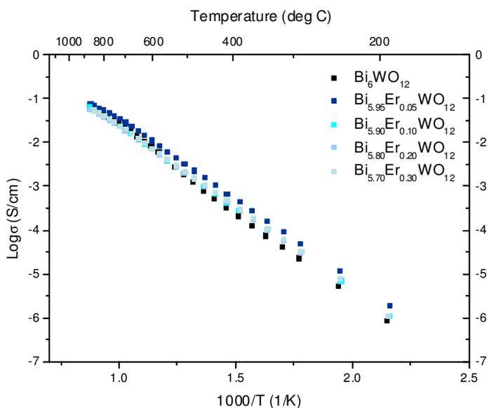
**Figure 6.31: Arrhenius curves of conductivity for all samples measured in the  $\text{Bi}_{6-x}\text{Er}_x\text{WO}_{12}$  system.**
