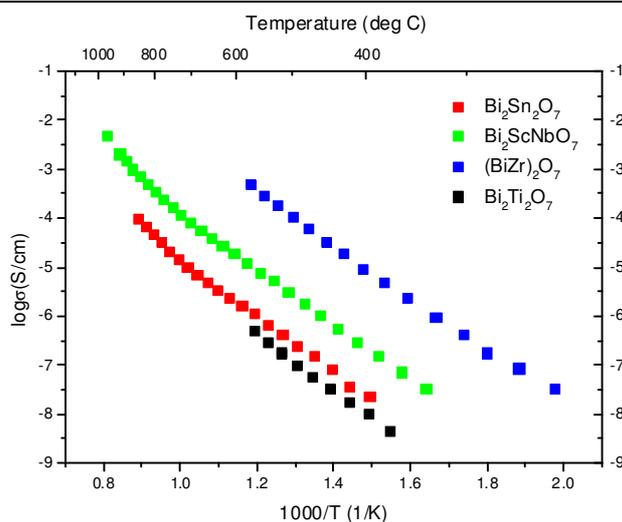
**Figure 8.1: Comparison of the conductivity of  $Bi_2Ti_2O_7$ ,  $Bi_2Sn_2O_7$ ,  $Bi_2ScNbO_7$  and  $(BiZr)_2O_7$ .**
