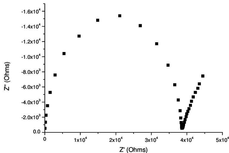
Figure 6.19: Complex impedance plot for  $\text{Bi}_{5.9}\text{Ca}_{0.1}\text{WO}_{11.95}$  at 241 °C.
