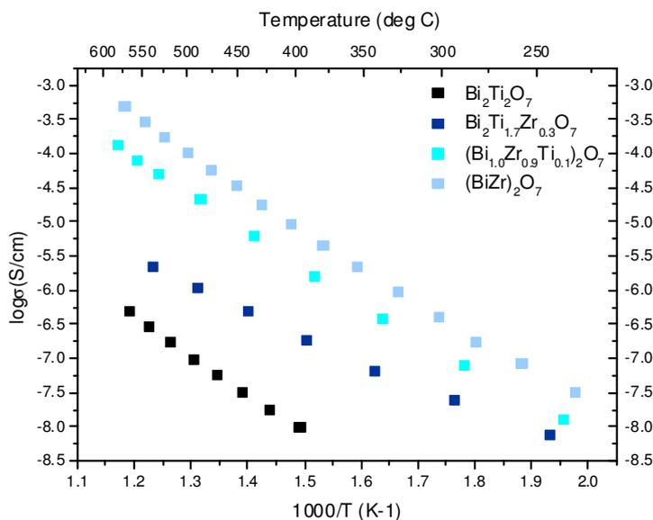
Figure 3.25: Variation of conductivity with temperature for members of the  $\text{Bi}_2\text{Zr}_{2-x}\text{Ti}_x\text{O}_7$  system.
