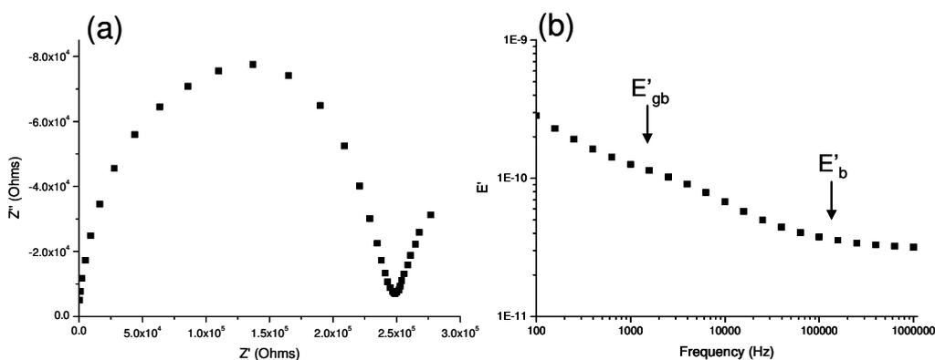
**Figure 6.9:** (a) Complex impedance plot for  $\text{Bi}_6\text{WO}_{12}$  at 193 °C. (b) Graph of capacitance versus frequency for  $\text{Bi}_6\text{WO}_{12}$  at 193 °C, which shows two plateaus and they have been assigned to the bulk ( $E'_b$ ) and the grain boundary ( $E'_{gb}$ ).
