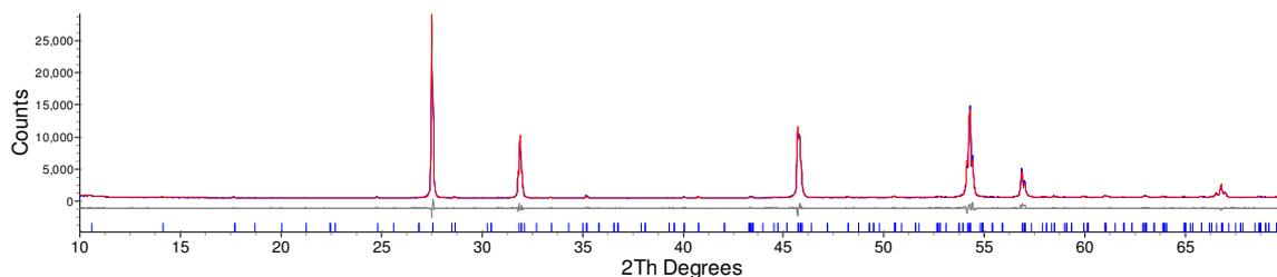
Figure 6.32: d9\_04106: Rietveld fit for  $\text{Bi}_{5.95}\text{Er}_{0.05}\text{W}_{0.95}\text{Zr}_{0.05}\text{O}_{11.95}$ .  $R_{\text{wp}}$  5.869%.
