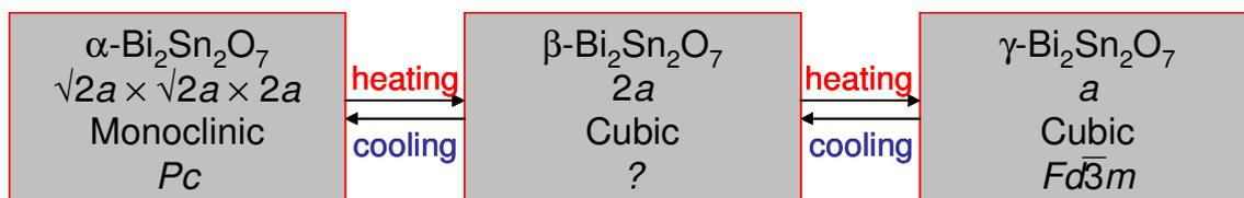
Figure 4.1: Phase transformations of  $\text{Bi}_2\text{Sn}_2\text{O}_7$ .<sup>1-3</sup>
