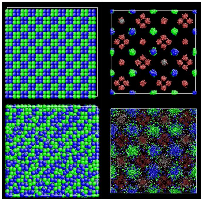
**Figure 3.19:** Comparison of the ideal pyrochlore structure with the RMC configuration for  $\text{Bi}_2\text{Ti}_2\text{O}_7$ . Top ideal pyrochlore, bottom RMC configuration of  $\text{Bi}_2\text{Ti}_2\text{O}_7$ . Left hand side: arrangement of cations in 6 x 6 x 6 supercell. Right hand side: RMC configuration condensed down onto one unit cell.
