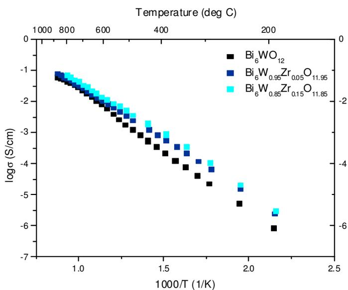
Figure 6.27: Arrhenius plots for the  $\text{Bi}_6\text{W}_{1-x}\text{Zr}_x\text{O}_{12-x}$  system.
