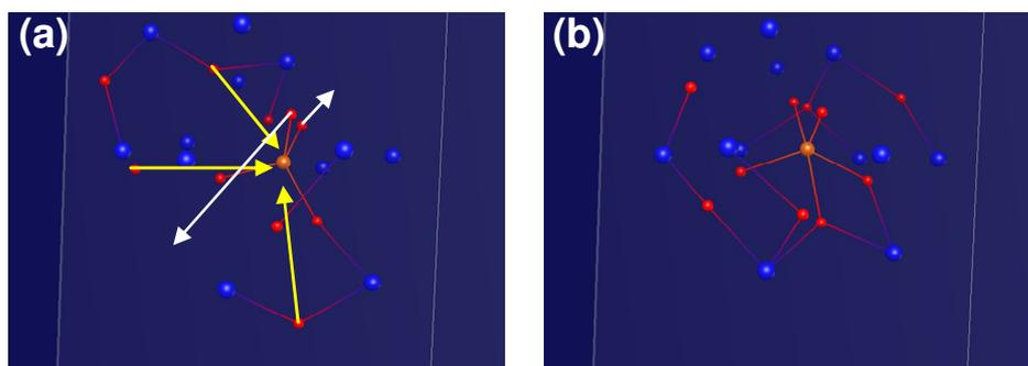
Figure 7.4: Variable coordination number environments for  $VO_x$  at 873 K. (a) Four coordinate vanadium and (b) five coordinate vanadium. White arrows show oxygen atoms leaving the coordination sphere of vanadium, whilst yellow arrows show oxygen atoms entering the coordination sphere of vanadium. Red spheres are oxygen atoms, orange spheres are vanadium atoms and blue spheres are bismuth atoms.
