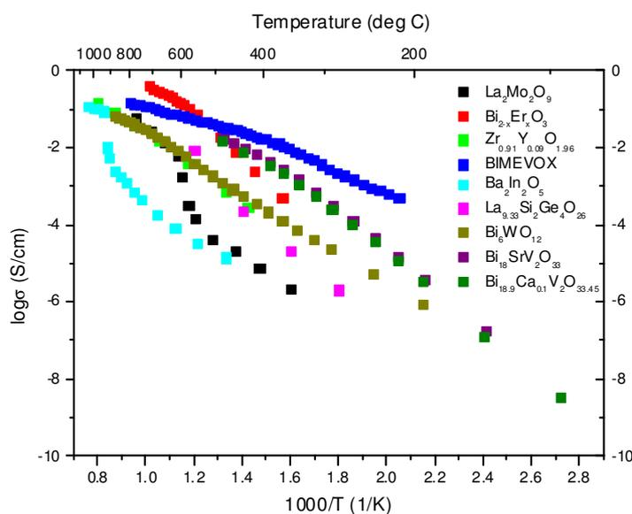
Figure 7.16: Comparison of conductivity of  $\text{Bi}_{18.9}\text{Ca}_{0.1}\text{V}_2\text{O}_{33.45}$  and  $\text{Bi}_{18}\text{SrV}_2\text{O}_{33}$  with that of other good, well known oxide ion conductors.<sup>4, 10-13</sup>
