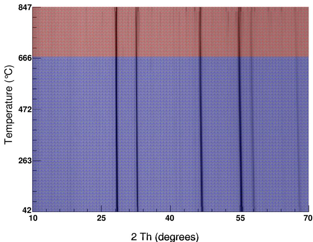
Figure 7.12: d9\_04852: *In-situ* VT-PXRD for  $\text{Bi}_{18}\text{SrV}_2\text{O}_{33}$ . No phase transformations were observed in the laboratory PXRD data and decomposition occurred at 666 °C. Pale blue region represents the stability range, whilst pale red region represents the decomposition range.
