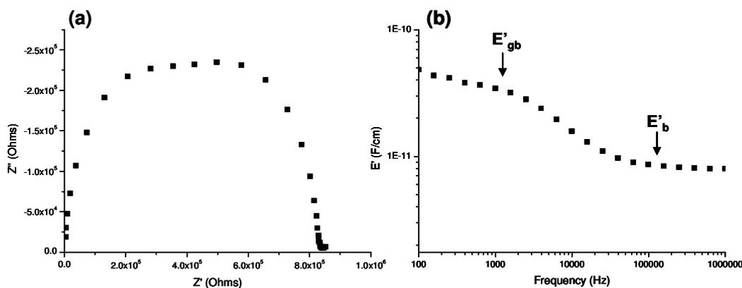
**Figure 4.26:** (a) Complex impedance plot for  $\text{Bi}_{1.8}\text{Ca}_{0.2}\text{Sn}_2\text{O}_{6.9}$  and (b) variation of capacitance ( $E'$ ) with frequency for  $\text{Bi}_{1.8}\text{Ca}_{0.2}\text{Sn}_2\text{O}_{6.9}$  showing two plateaus, indicative of the bulk ( $E_b$ ) and grain boundary ( $E'_{gb}$ ) responses.
