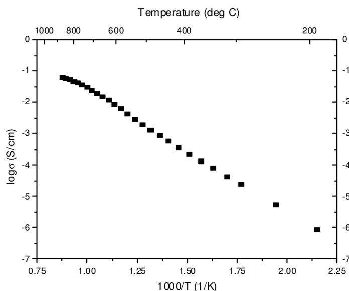
Figure 6.10: Arrhenius plot of conductivity for  $\text{Bi}_6\text{WO}_{12}$ .
