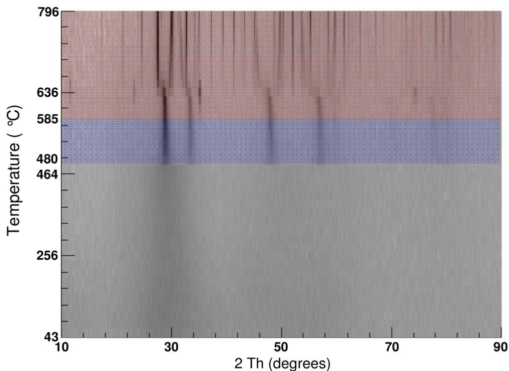
Figure 3.2: d8\_03517: *In-situ* VT-PXRD of the  $(\text{BiZr})_2\text{O}_7$  precursor, showing the  $(\text{BiZr})_2\text{O}_7$  formation and stability range (shaded pale blue) and the onset of decomposition (shaded pale red).
