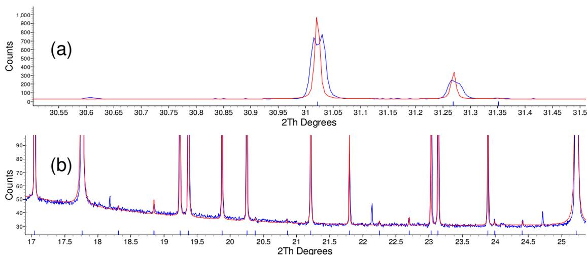
**Figure 4.5: Zoomed regions of Pawley fit for  $\beta\text{-Bi}_2\text{Sn}_2\text{O}_7$  in space group  $F\bar{4}3c$ . (a) Unaccounted peak splitting and (b) un-fitted peaks indicate that  $F\bar{4}3c$  cannot be the correct space group.**
