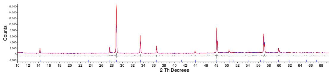
**Figure 4.39:** d9\_03333: Rietveld refinement of  $\text{Bi}_2\text{ScNb}_{0.9}\text{Zr}_{0.1}\text{O}_{6.95}$ .  $R_{\text{wp}} = 5.831\%$ .
