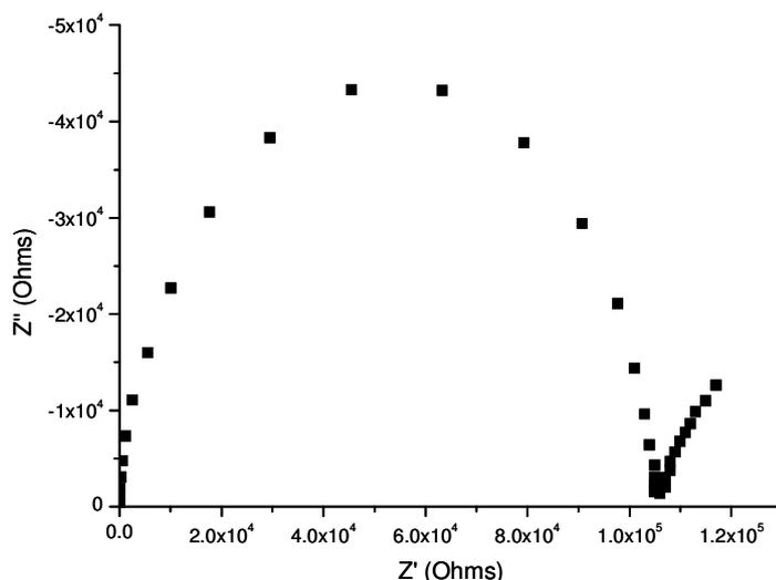
**Figure 6.30: Complex impedance plot at 191 °C for  $\text{Bi}_{5.95}\text{Er}_{0.05}\text{WO}_{12}$ . Response shows one high frequency arc due to the bulk contributions and one low frequency arc due to the electrode response.**
