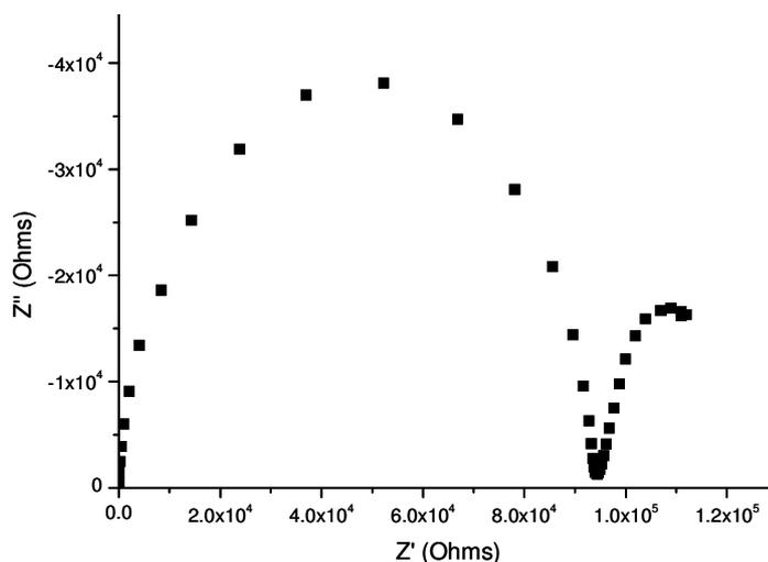
Figure 6.33: Complex impedance plot for  $\text{Bi}_{5.95}\text{Er}_{0.05}\text{W}_{0.95}\text{Zr}_{0.05}\text{O}_{11.95}$  at 190 °C.
