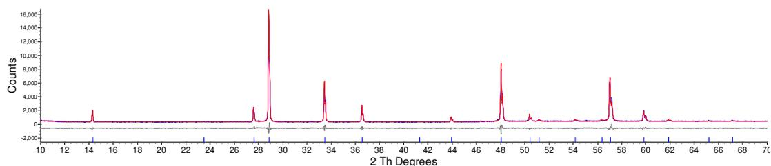
Figure 4.34: d9\_03232: Rietveld refinement for  $\text{Bi}_{1.9}\text{Ca}_{0.1}\text{ScNbO}_{6.95}$ .  $R_{wp} = 5.862\%$ .
