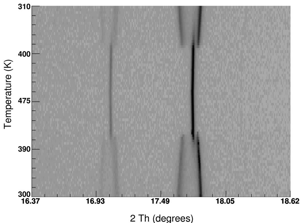
**Figure 4.2:** A small  $2\theta$  region of the heating and cooling I11 *in-situ* VT-PXRD data showing the  $\alpha\text{-Bi}_2\text{Sn}_2\text{O}_7$  -  $\beta\text{-Bi}_2\text{Sn}_2\text{O}_7$  phase transition.
