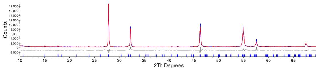
Figure 7.6: d9\_04445: Rietveld fit for  $\text{Bi}_{18.9}\text{Ca}_{0.1}\text{V}_2\text{O}_{33.45}$ ,  $R_{\text{wp}} = 8.387\%$ .
