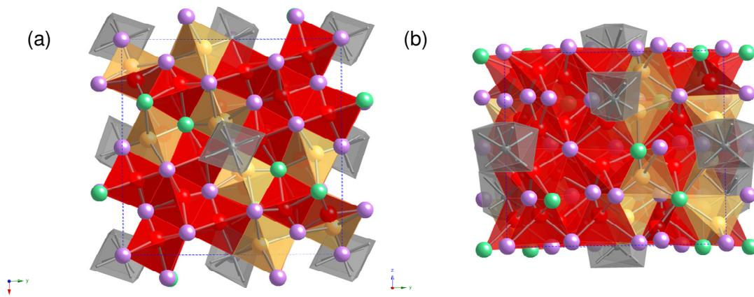
**Figure 6.5:** (a)  $ab$  plane and (b)  $ac$  plane of model for  $\text{Bi}_6\text{WO}_{12}$ . Red polyhedra are  $\text{OBi}_4$  tetrahedra, orange polyhedra are  $\text{OBi}_4$  tetrahedra with the oxygen site being partially occupied, grey polyhedra are  $\text{WO}_x$  units from fully occupied W site. Purple spheres are bismuth atoms and green spheres are the mixed bismuth/tungsten site.
