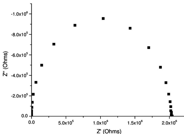
Figure 4.36: Complex impedance plot for  $\text{Bi}_{1.95}\text{Ca}_{0.05}\text{ScNbO}_{6.975}$  at 412 °C.
