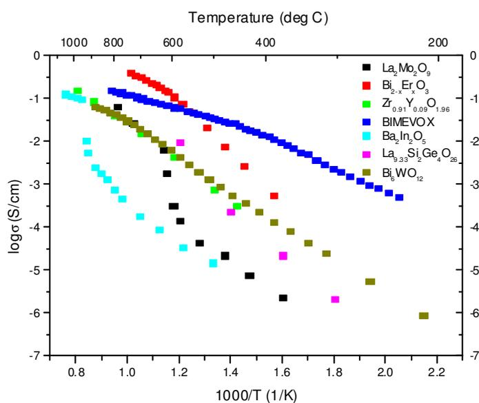
Figure 6.11: Comparison of oxide ion conductivity for  $\text{Bi}_6\text{WO}_{12}$  with that of other good oxide ion conductors.<sup>11-14</sup>
