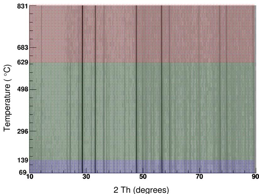
**Figure 4.19:** d8\_03718: VT-PXRD plot for  $\text{Bi}_2\text{Sn}_{1.6}\text{Zr}_{0.4}\text{O}_7$ . Blue patterns show stability of  $\alpha$  phase, green patterns show stability of  $\beta$  phase and red patterns show the stability of the pyrochlore phase.
