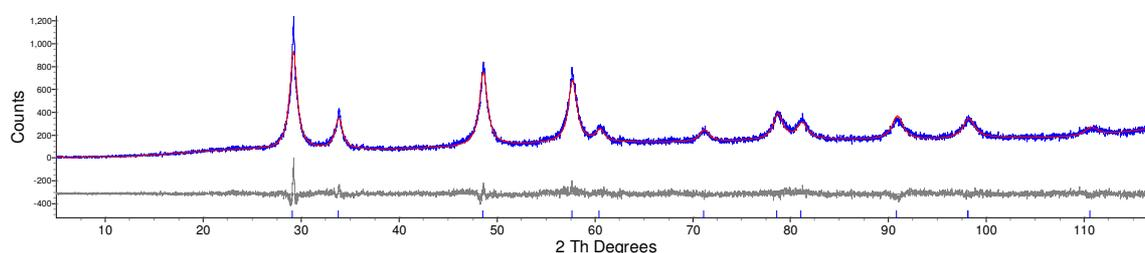
**Figure 5.4:** d5\_07882: Fluorite type  $\text{Nd}_2\text{Zr}_2\text{O}_7$  after annealing for 309 hours at 800 °C. Rietveld refinement for a fluorite structure.  $R_{\text{wp}} = 9.389\%$ ,  $a = 5.3014(4)$  Å.
