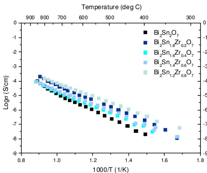
Figure 4.21: Variation of conductivity with temperature in the  $\text{Bi}_2\text{Sn}_{2-x}\text{Zr}_x\text{O}_7$  system.
