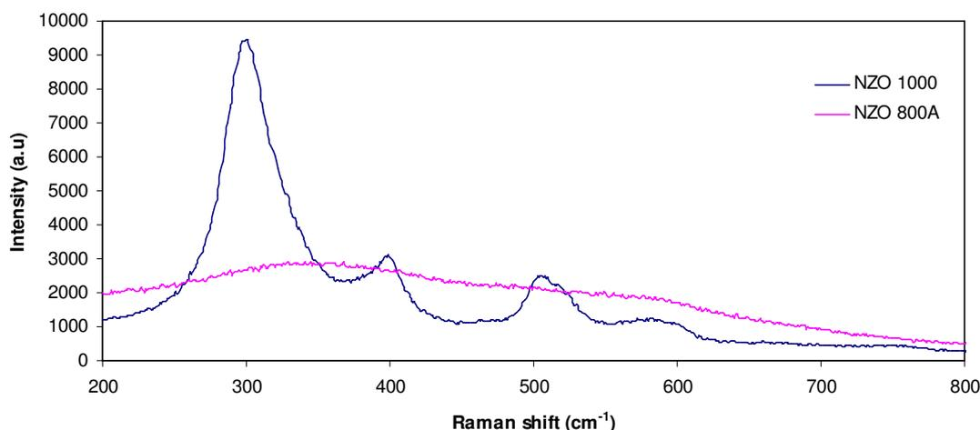
Figure 5.12: Raman spectra of NZO 1000 and NZO 800A.
