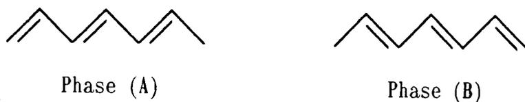
Figure 1.16 *Degenerate Forms of (CH)<sub>x</sub>.*
