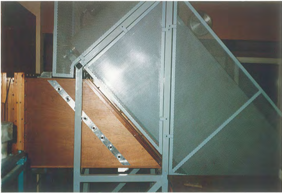
FIGURE 4.3 : Turbulence Grid Viewed From the Tunnel Side
