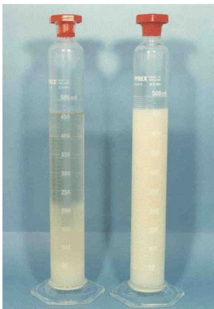
Figure 2.14: Wax crystals formed in the presence of EVA only (left); EVA and WASA (right), picture provided by Infineum
