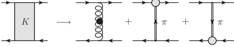
**Figure 6.8.:** Pion cloud effects into the quark-antiquark scattering kernel, as required by the axWTI, Eq. (6.13).
