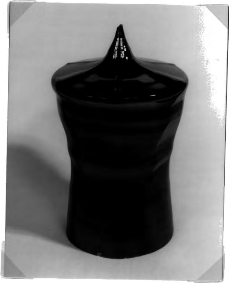
Fig. 4.9 Photograph of Silicon single crystals. It was grown by rapid increase in the diameter.
