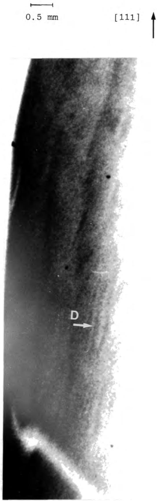
Fig. 3.2 X-ray reflection topograph revealing domains and a large misorientation region appears as a light band. 440 reflection, MoK $\alpha$  radiation.
