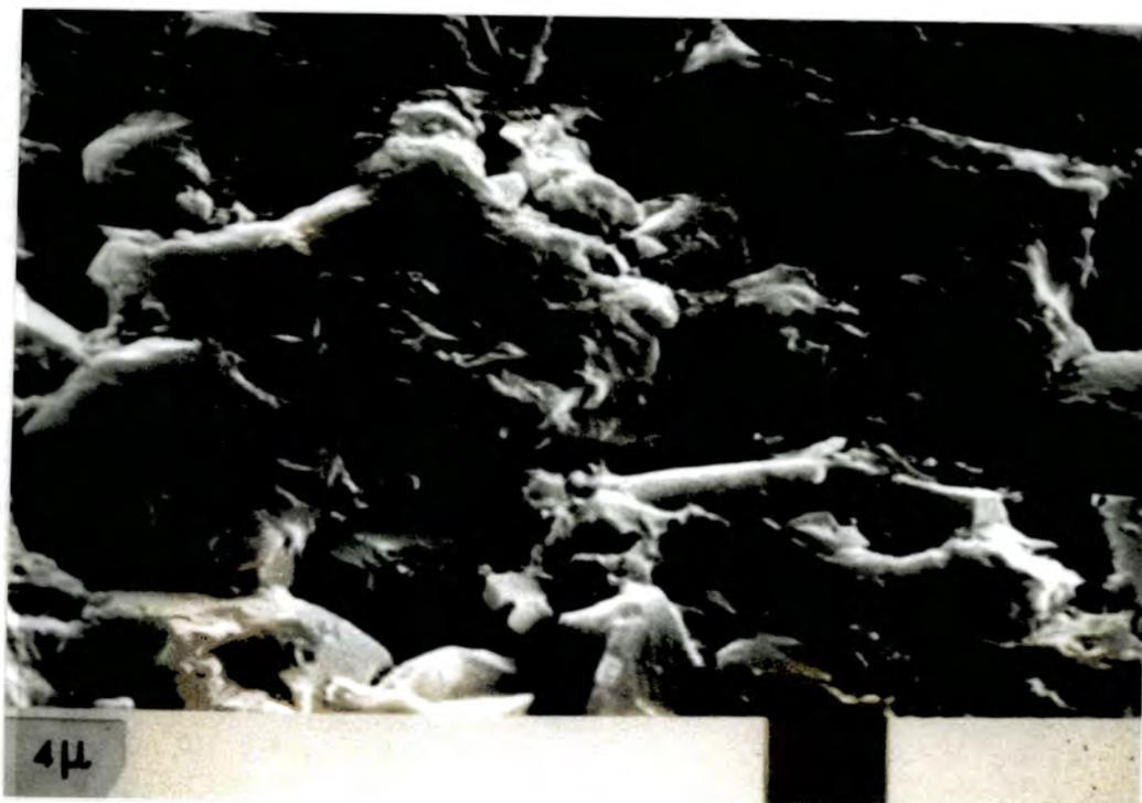
FIG 4.8: A typical SEM micrograph for black alumina
