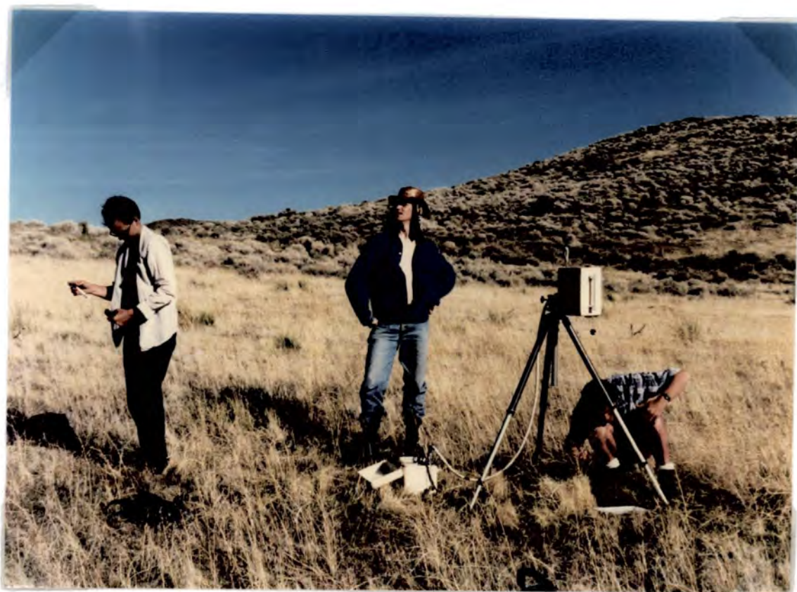
Plate 6.10 An area of dry grass (labelled B on the location map, figure 6.2). There is no outcrop and the grass cover is almost complete. Field spectral measurements were taken to determine the spectral response of the grass (figure 6.13).
