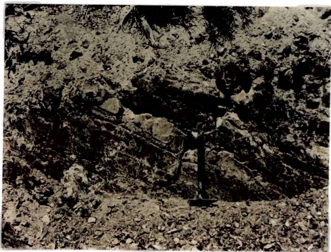
Plate 6.7 Adelaide mine, Site 3, Location 2. Situated above the mine entrance in a bulldozed cutting. The folded, silicified limestones are clearly visible.
