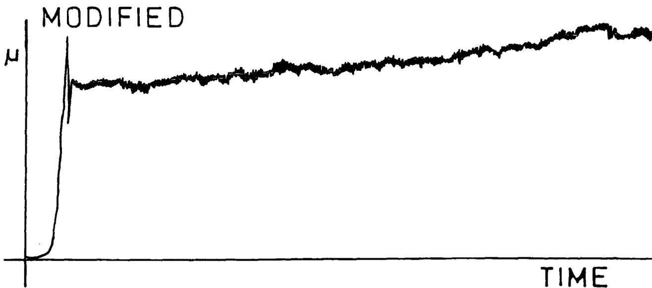
Figure 3.11 Variation of COF with Time for Nylon and Modified Nylon against Nylon.
