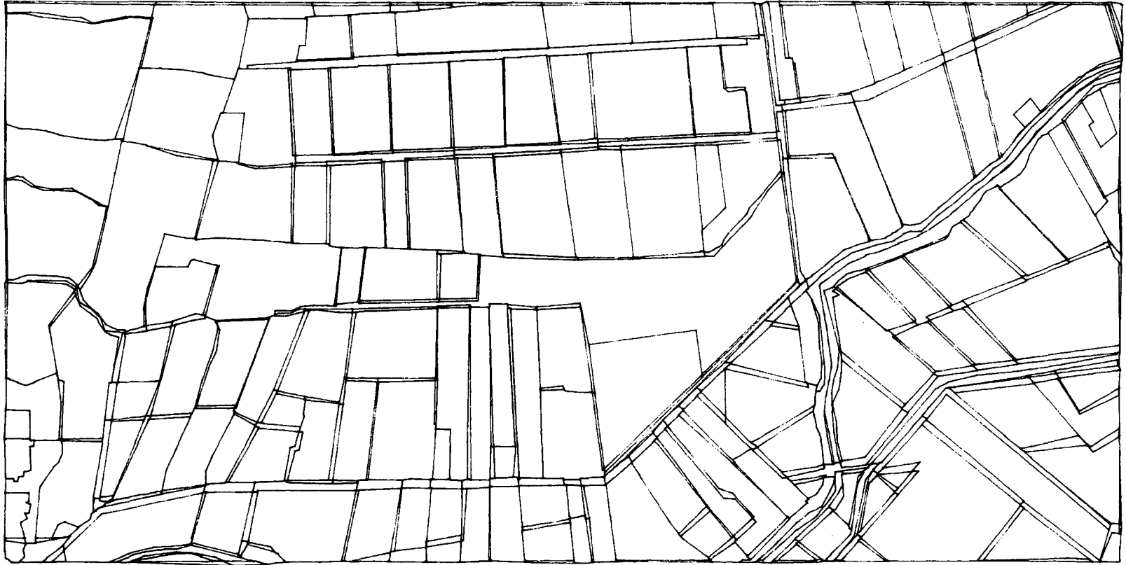
6.38 An overlay of the 1:50,000a coverage and the 1:50,000b coverage following an ELIMINATE of AREA 5,000 units
