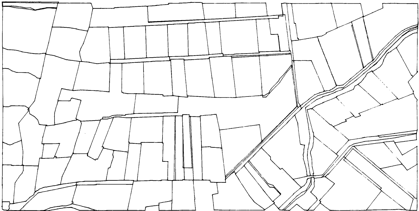
6.36 An overlay of the 1:50,000a coverage and the 1:50,000b coverage following an ELIMINATE of PERIMETER 2,000 units
