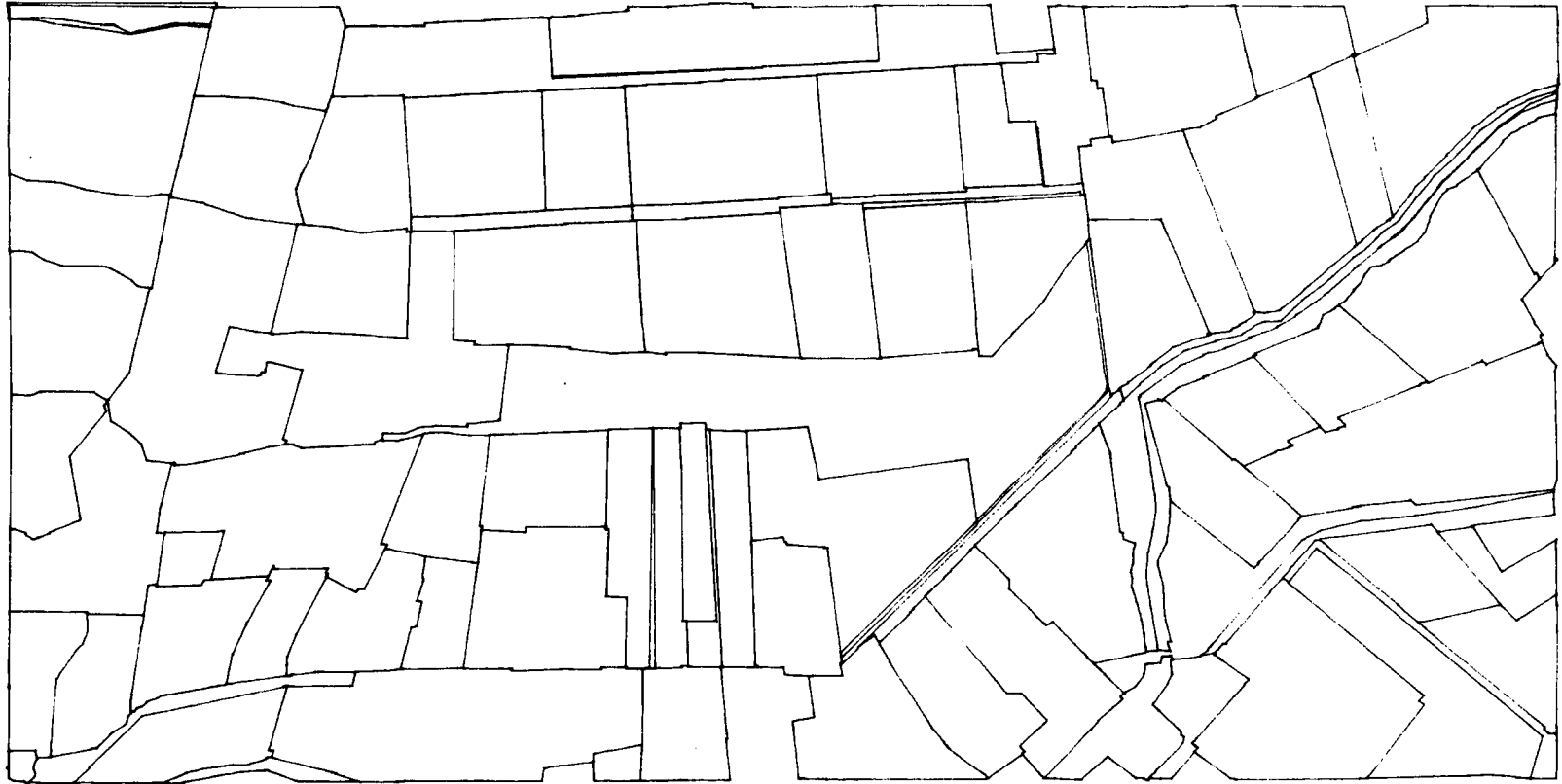
6.37 An overlay of the 1:50,000a coverage and the 1:50,000b coverage following an ELIMINATE of PERIMETER 2,500 units
