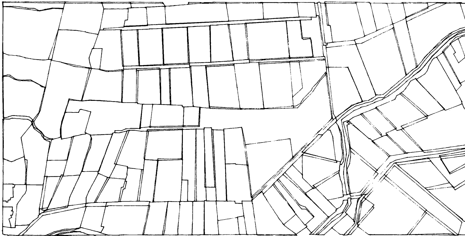
6.35 An overlay of the 1:50,000a coverage and the 1:50,000b coverage following an ELIMINATE of PERIMETER: 1,000 units
