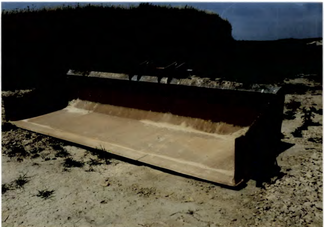
7/. Specially design "bucket" for transplanting turfs.
